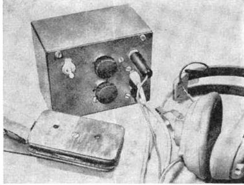
The complete assembly consists of the search coil, a pair of headphones and the electronics package.
