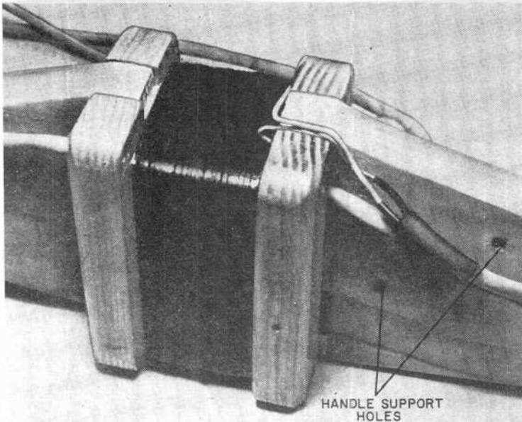
evenly and firmly as possible and avoid kinking the wire. When the winding is finished, protect it with a couple of layers of plastic electrical tape. Be sure that you can identify each end of the coil.
