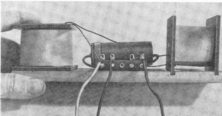
wire out through the remaining holes in the coil forms. Scrape away about  $\frac{1}{2}$ " of the insulating enamel from the free ends of the coil windings.
