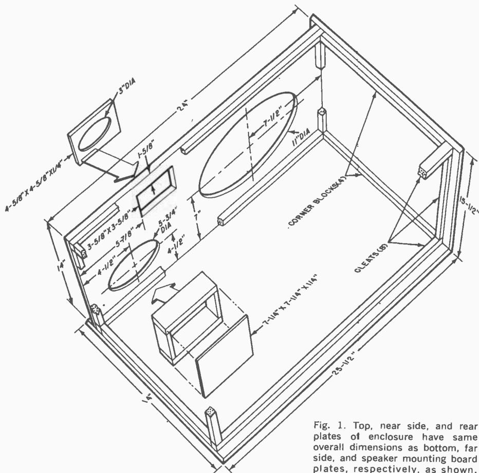
Fig. 1. Top, near side, and rear plates of enclosure have same overall dimensions as bottom, far side, and speaker mounting board plates, respectively, as shown.
