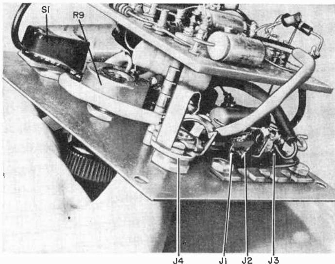
The perf board is mounted on four long spacers to provide room for the front-panel components. The battery is secured in a clip affixed to the panel.
