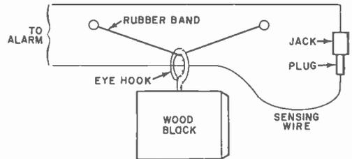
would be to use a length of solder (preferably the low-temperature kind) in place of the rubber band. The solder will melt through when heat is applied, and the block will fall as described.
