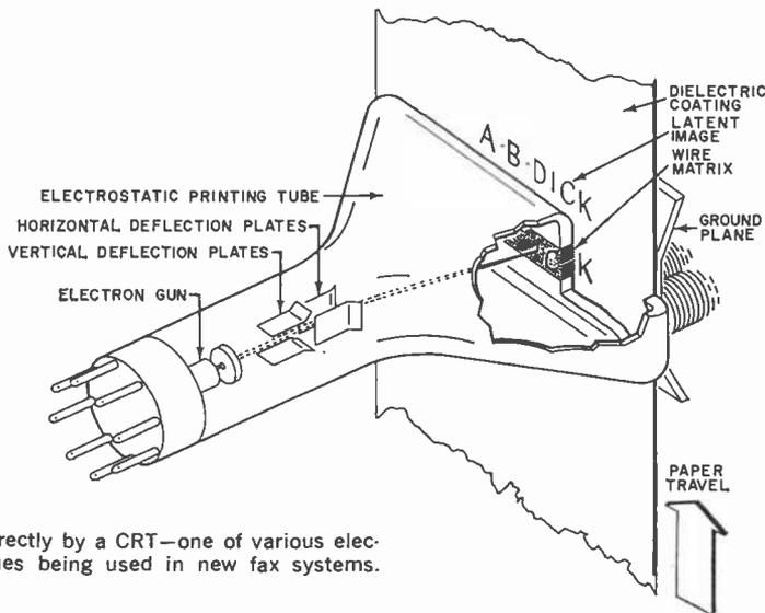
Fax printing directly by a CRT—one of various electronic techniques being used in new fax systems.
