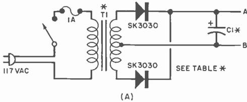
**M**ANY READERS have asked us to print a circuit design for a power supply that would be simple yet would provide the unusual d.c. voltages that may be required in experiments and project constructions involving semiconductor. In answer to these requests, we suggest a circuit given in the *RCA Solid-State Hobby Circuits Manual*. (The handbook is available at most electronics parts distributors for \$1.75.)
