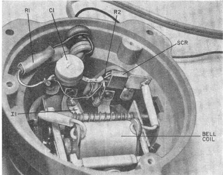
dered to a length of insulated wire (the touch contact connector lead). Insulate *R1* and its soldered contacts using plastic tape. Pass the loose end of the contact wire through the same rubber grommet holding the a.c. power line. The alarm is now ready to test.
