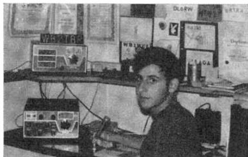
Using simple wire antennas in his attic and a Drake TR-3 transceiver backed up by a Drake R-4 receiver, Donald J. Perlstein, WB2TBP, has worked 50 states and 98 countries. Don has an Extra class license.
