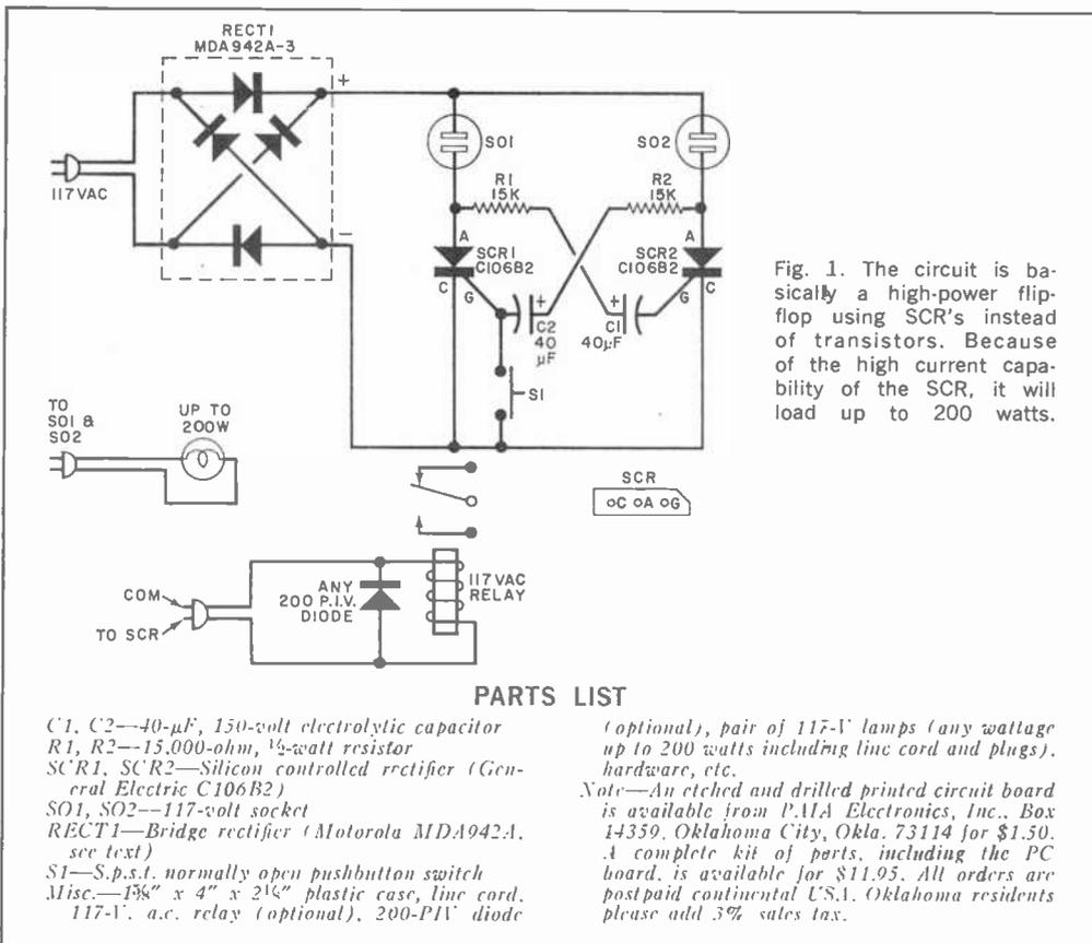
Fig. 1. The circuit is basically a high-power flip-flop using SCR's instead of transistors. Because of the high current capability of the SCR, it will load up to 200 watts.
