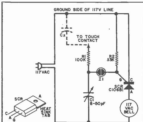
The capacitance of the body,  $Cx$ , when contact is made with lead to  $R1$ , causes voltage on  $C1$  to break down  $I1$  and fire SCR.
