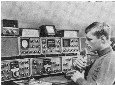
Henry Kirk, WA3DZE, Muncy, Penn., must like Heathkit equipment. However, a Hallicrafters HA-1 electronic keyer; Ham-M beam rotator; and an Astatic D-104 microphone appear amid the SB-110A 6-meter transceiver; SB-401 transmitter; SB-301 receiver; SB-201 linear amplifier; and other Heathkit gear.
