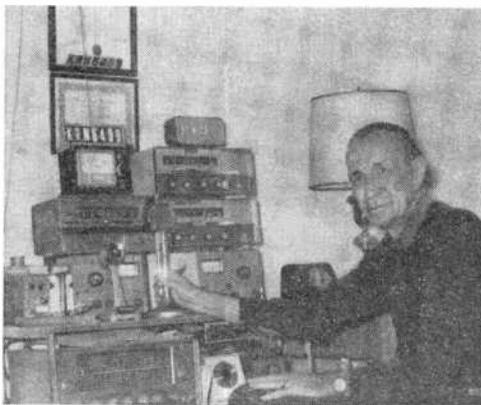
One of our monitors in the Far North is Clifford Duncan, VE5PE5V, Cut Knife, Saskatchewan, Canada. He uses a Trio 9R-59 receiver, and RCA transistorized portable recorder and an inverted L antenna. He has DX awards for 50 states and 20 zones.
