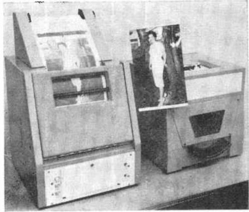
In units about the size of a treadbox, conventional fax system records photo by insertion at right and reproduces at left. (Photo International Scanatron)
