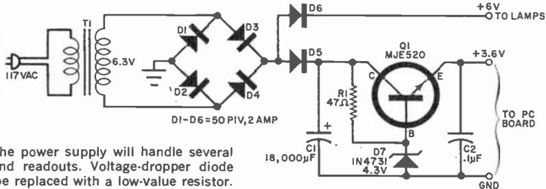
Fig. 8. The power supply will handle several DCU's and readouts. Voltage-dropper diode D6 can be replaced with a low-value resistor.
