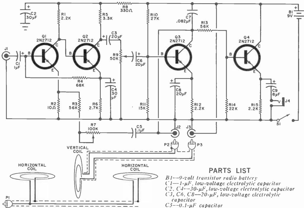
Fig. 1. Basically an unstable high-gain audio amplifier, the circuit breaks into oscillation when metal is detected between horizontal and vertical coils.
