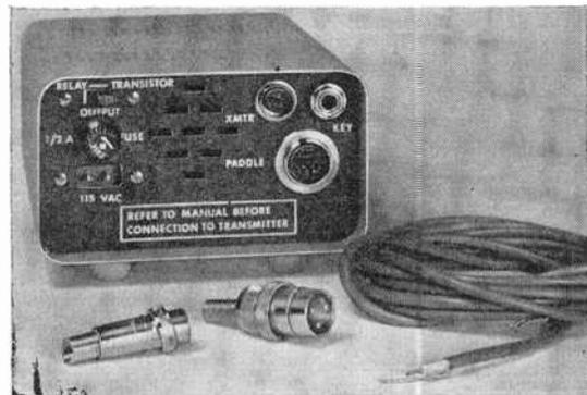
Rear apron of Curtis EK-38 electronic keyer accommodates all external cable connectors, a relay/transistor output selector switch, and power fuse. Mating connectors and cables (shown in foreground) are supplied with kit.
