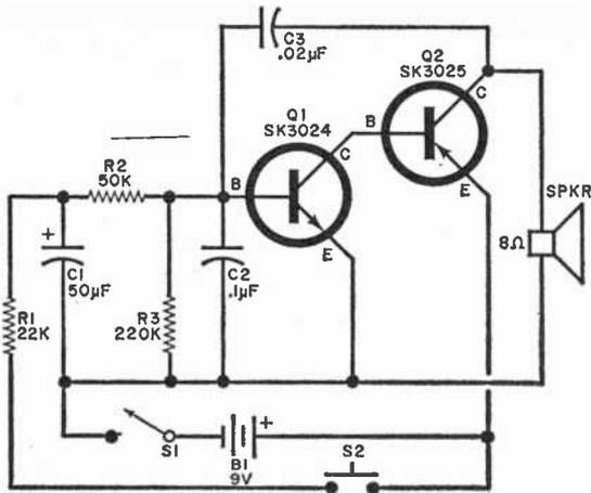
Fig. 2. Electronic siren circuit at left produces short, high-pitched scream when S2 is depressed, followed by the falling wail typical of sounds heard from police sirens.
