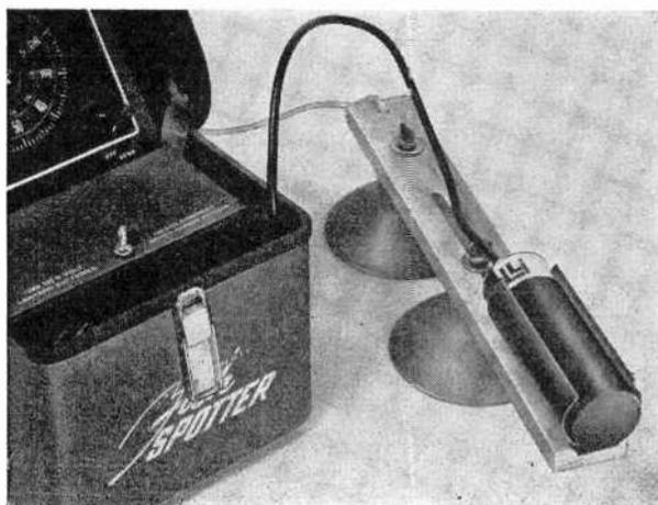
Except for the transducer, indicator assembly, and battery supply, all electronic parts mount on large printed circuit board, which is bolted to flip-up water-tight metal cover.
