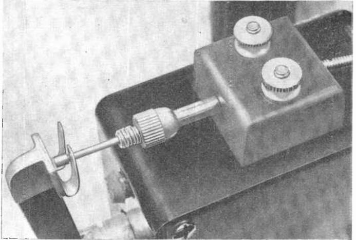
cate and drill the exit hole for the arm of the solenoid, centering it between the two sides of the box. Then drill the mounting holes for the solenoid and actuating arm pivot bracket, and for the potentiometer (located directly opposite the exit hole for the solenoid).
