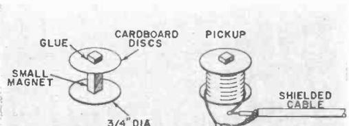
Bond cardboard discs to magnet with epoxy cement. Tape cable to pickup coil winding.
