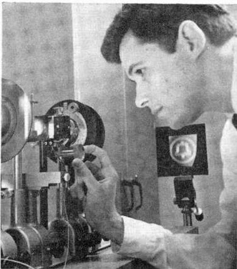
Bell Laboratories' Juan Maldonado adjusts focus of image from ferpic device on small viewing screen.
