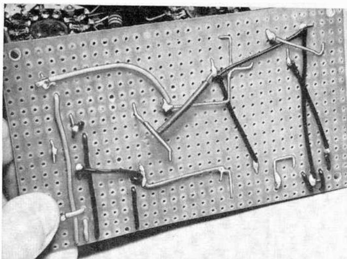
Insulated wiring is used to make interconnections. If a metal case is used, make sure spacers keep connections from touching the case.
