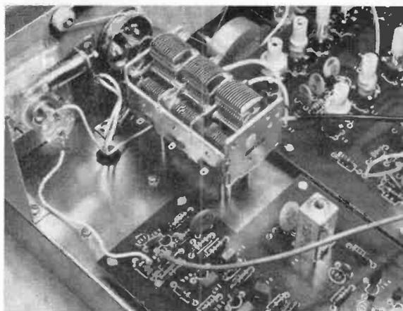
The printed circuit boards (above) are supplied pre-soldered and partially pre-aligned. Builder makes the necessary interconnections, mounts the front and rear panel controls and terminals and then threads that #14% dial cord through the hole.
