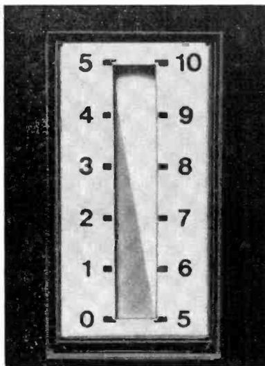
Two hundred microampere meter on new 150 is "different." Wired to collector of the audio output stage, the speaker had to be blasted to get reading half-way up scale. It looked like cat's eye.
