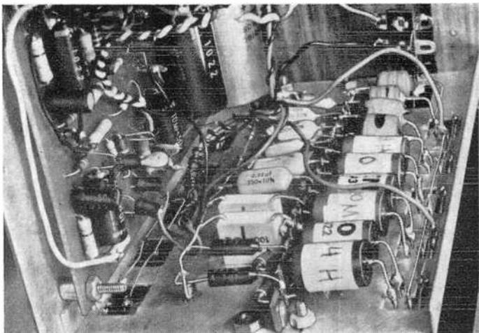
To provide clearance for and access to solder lugs on potentiometers, cutouts must be made through the filter subchassis bracket.
