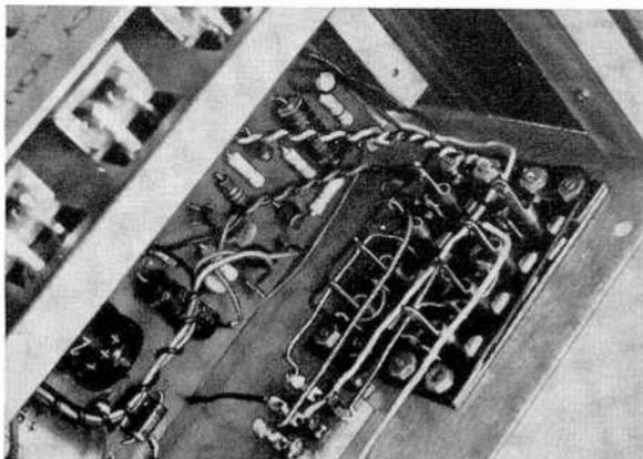
Note short wires for input connections and twisted pairs for the two outputs.
