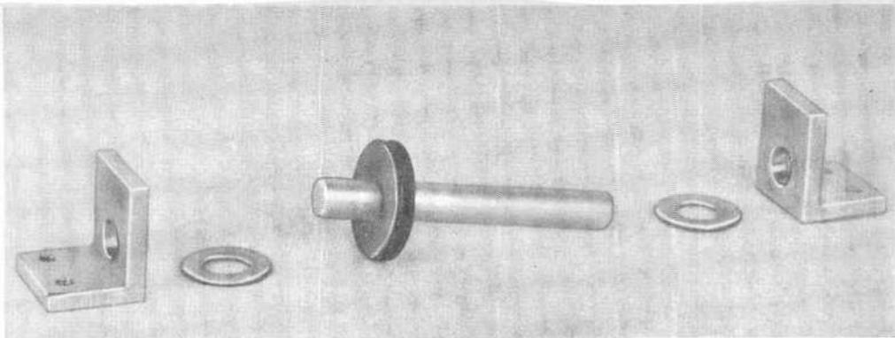
Shown is correct sequence of assembling parts that make up dial tuning assembly. Flat metal washers are used to reduce friction and wear between pulley and support brackets and to prevent play between them.
