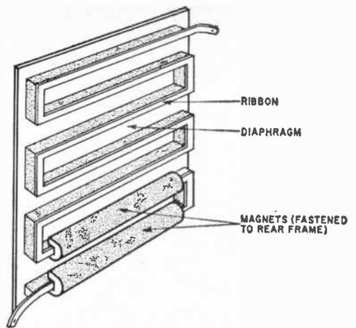
The Ge-Go "Orthophase" speaker had a long folded ribbon fastened to rear of flat diaphragm with a grooved magnet assembly interleaved with ribbon.
