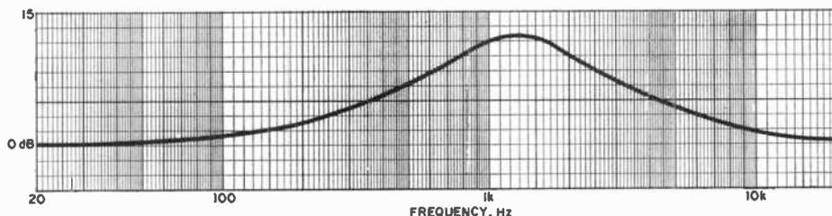
New curve was obtained with all controls set at zero, except 1000 Hz control set at  $+12$  dB.
