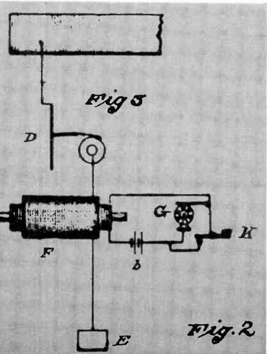
Above is one of the drawings from Edison's Patent No. 465,971, Dec. 29, 1891, describing a "Means for Transmitting Signals Electrically." Particularly interested in transmitting across bodies of water, he showed high towers and ships carrying "condensing surfaces" (which we would call antennas). At the right is an enlargement of the insert, in which Edison described how signal was generated and transmitted to antenna.
