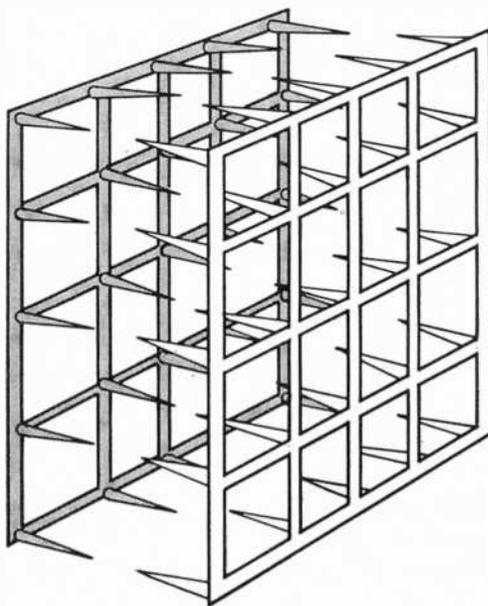
Corona-wind speaker has high-voltage charge on two elements to move air molecules between them.
