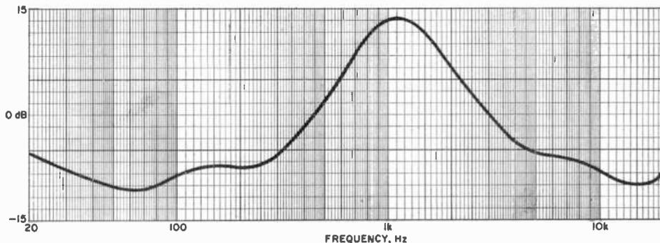
This curve was obtained with all controls set at  $-12$  dB, except 1000 Hz control at  $+12$  dB.
