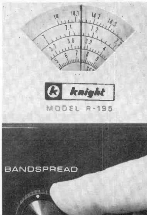
Considering the selectivity and excellent sensitivity of the R-195, the totally inadequate main tuning and bandspread arrangements are almost criminal. Only below 4 MHz does the operator have a chance of setting up cold on a desired frequency.
