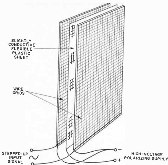
In push-pull electrostatic speaker, the flexible plastic sheet is either attracted or repelled by the opposing charges on the wire grids. Design must be large for good bass reproduction, but it makes good tweeter.
