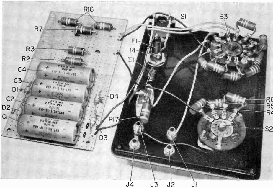
Perf board construction may be used with the operating controls and jacks mounted on the front panel of the selected cabinet. A TV-type "cheater" connector is used to make the power connection. Mount the perf board on suitable spacers and be sure that components on the board do not make electrical contact with any of the front-panel elements.
