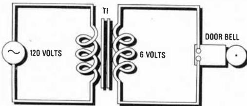
In this door bell circuit, which kind of transformer is T<sub>1</sub> — step-up or step-down?
