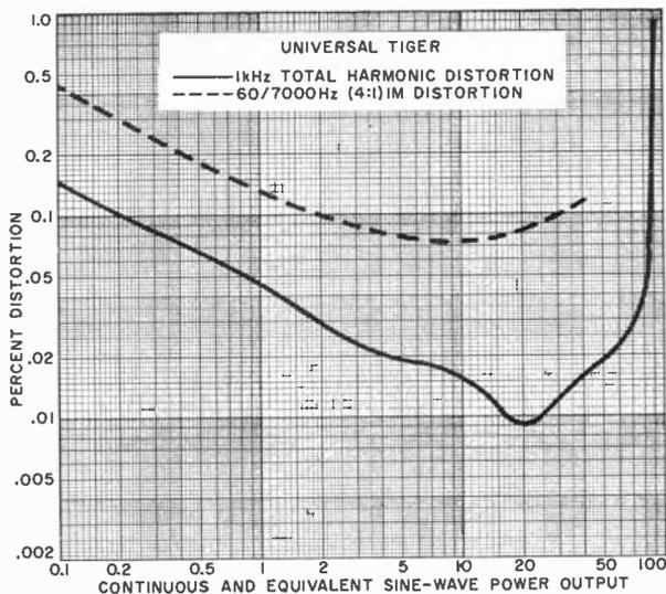
than 40 watts. These figures were measured with the bias adjust control set as received with best thermal stability. The low-level distortion could be reduced substantially with this control set at its opposite limit, where the measured reduction was from 0.045% to 0.023% at one watt and from 0.15% to 0.047% at 0.1 watt. However, it is hardly worth the bother to play with the bias adjust control, since we doubt that many people have the test equipment needed to make the adjustment.
