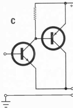
supply voltage. This simplifies design demands. Second, it is possible to keep distortion down to much lower levels in the driver circuit if it does not have to develop full supply positive and negative excursions. Additional temperature stability, by using 50 percent feedback in the output stage, is yet another advantage.
