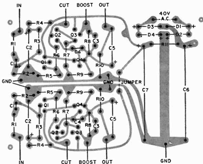
Fig. 3. When mounting components on circuit board, make sure that lead orientations of electrolytic capacitors, diodes, and transistors are correct.
