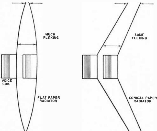
A flat surface, with minimal rigidity, moves a relatively large amount in reproducing necessary sound. The stiffness of the radiator is increased significantly, without affecting the mass when surface is shaped into cone.
