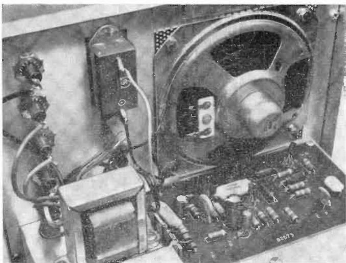
Behind the panel of the 150, wiring is very simple. Audio amplifier is assembled on a printed circuit board. Power transformer is at lower left.
