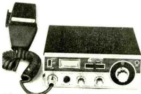
produces the last i-f. Channels are changed by switching in different crystals in proper combination at the first mixer. A delta-tune setup at the second conversion oscillator has three positions which permit the receiver's frequency to be shifted by a given amount around the center frequency.
