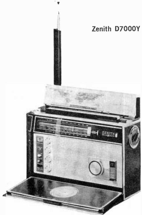
ing twice. Although the receiver gives the impression of being "hot," due to its busy-sounding bands, much of this is the result of spurious and image responses.
