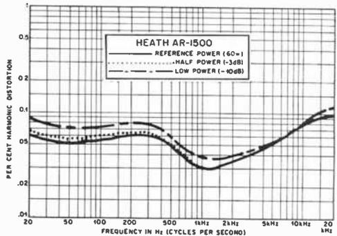
Curves on graph show percent harmonic distortion present at various power levels between 20 and 20,000 Hz.
