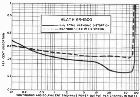
Total harmonic and intermodulation distortion are shown for continuous sine-wave output power per channel.
