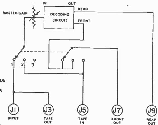
The Master volume control provides control of all four channels when decoding. To start, turn this control fully clockwise. Then advance the volume controls of the front and rear amplifiers to the loudest level you
