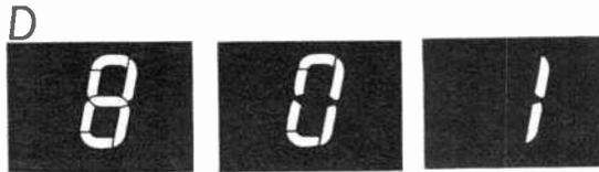
Microelectronic calculators such as those above with liquid crystal displays, are being manufactured in volume by such companies as North American Rockwell. In the display shown at (A), each digit has seven segments, each with an electrical lead, formed on glass plates with transparent tin oxide. Two glass plates are bonded together with about 1/1000 of an inch between them. This space
