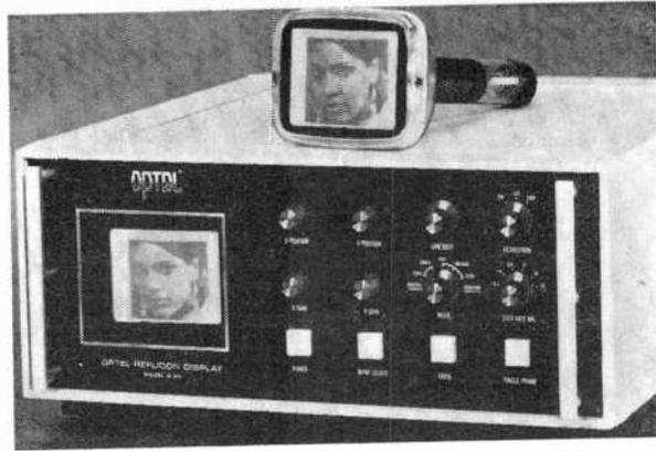
Fig. 4. Nematic storage-mode Reflicon tube and demonstrator. (Photo: Optel)
