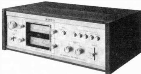
America. The decoder handles SQ and RM discs. Since SQ-encoded 4-channel records normally retain full left-to-right separation but exhibit reduced front-to-rear separation during playback, the SQD-2020 has a dual logic circuit that substantially increases front-to-rear
