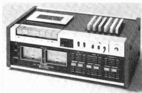
toggle-type switches and a pushbutton power switch. Two of the toggle switches are used to select bias and equalization, both recording and playback, for NORMAL and HIGH energy ferric-oxide and chromium-dioxide tape formulations. (The new 70  $\mu$ s playback equalization characteristic is used for chromium-dioxide tape to yield the best signal-to-noise ratio.)
