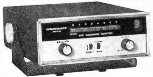
channel. Two IC amplifiers provide gain, limiting, and quadrature FM detection. A five-transistor squelch circuit cuts off the first audio amplifier in the absence of a pre-determined signal level. The audio amplifier supplies about 2 watts of power to a built-in loudspeaker or to an external 4-ohm speaker.
