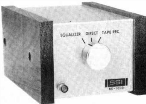
frequency equalizer introduced by Sound Systems International. This device boosts frequencies below 250 Hz without affecting the midrange or high frequencies. And it can be used with all types of speaker systems currently in use. For convenience and flexibility, the BD-1000 also has its own mode switch that allows the user to switch the equalizer in and out of a hi-fi system as desired.
