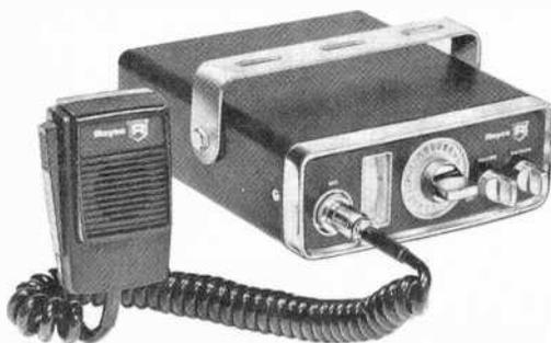
**T**HE moderately priced Model 1-600 solid-state mobile CB transceiver from Royce Electronics features crystal-synthesized operation at full legal power on all 23 AM channels. It has a meter that indicates relative signal strength on receive and relative output power on transmit. Additionally, the transceiver incorporates only the main essentials: adjustable squelch, a-f volume control, au-
