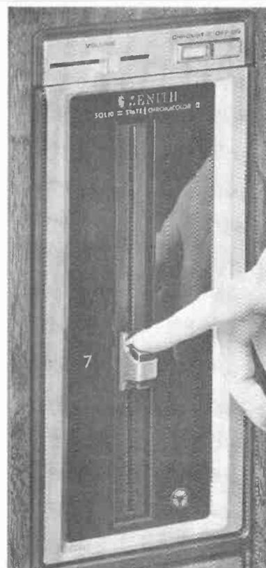
*Choosing channels on Zenith's color TV receiver line is accomplished with non-detented slide control*
