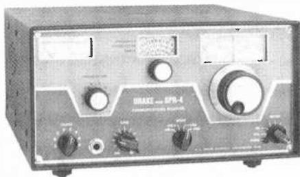
**T**HE Drake Model SPR-4 solid-state communications receiver covers any 23 bands (each 100-kHz wide) between 150 kHz and 30 MHz. Thus, it offers the user reception of international SW, amateur radio, and CB radio transmissions, among others.
