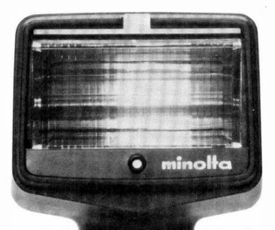
charge. (On manual, these same batteries would deliver only about 60 flashes per charge. Since no one shoots exclusively at distances of 2.5 ft (0.76 m), the more usual number of flashes per charge is about 100 to 200.
