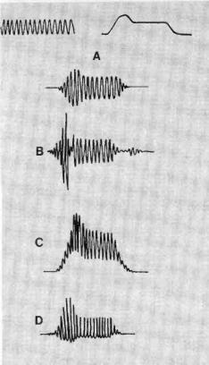
Fig. 1. In a good keyer, pitch and envelope waveforms (above A) are combined to produce a note which is their mathematical product (below A). Output of poor keyer (B) has excessive transients; (C) has envelope in output; (D) has unequal positive and negative swings.
