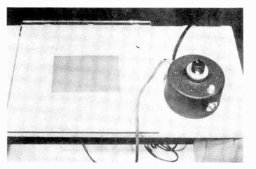
Electrophotography kit is set up on top of carton in which it is received.
