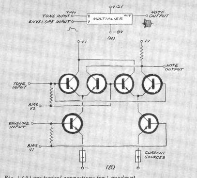
Fig. 4 (A) are typical connections for 4-quadrant multiplier. Key internal circuitry is shown at (B).
