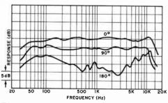
Fig. 3. Cardioid frequency response on axis and at two angles off-axis.
