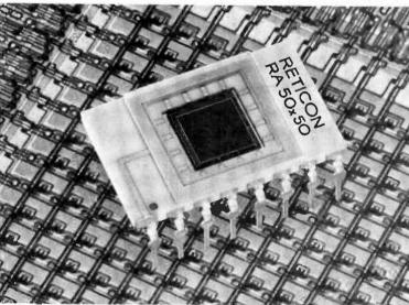
Fig. 4. Close-up of the Reticon RA 50×50 sensor. The background is photo of the array magnified many times.
