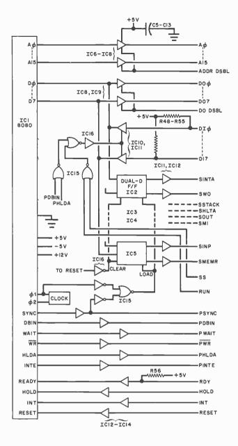
Fig. 3. The logic associated with the CPU (ICI) is shown at left. All of the buffers and latches are on a single pc board. Connecting wiring is through a 100-line buss.
