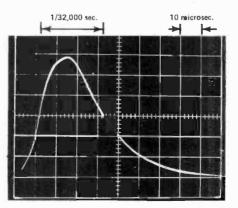
We used a high-speed oscilloscope to check flash duration of the Braun 2000, set to give briefest flash of 1/32,000 s. Measurement from pulse width at half height.
