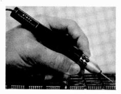
input. The LCA-2 is supplied with a 4-foot coaxial cable, BNC connector, and three input adapters. It can indicate polarity/duty cycle of pulse trains as high as 25 MHz. The probe measures 5½-in. long and %-in. in diameter. \$69.50.
