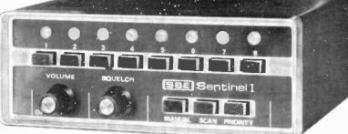
8 channels—continuous "scanning". Receiver locks on first channel on which signal appears.
