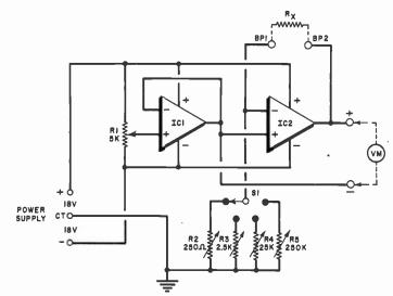
Linear scale ohmmeter uses two intergrated circuits. When the circuit is properly balanced (via range switch and potentiometers), the meter reading is proportional to the unknown resistor.
