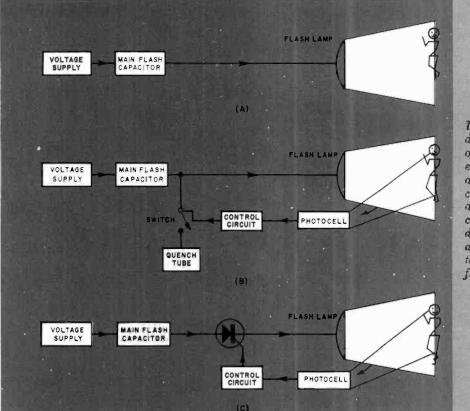
Three greatly simplified block diagrams show the major components of the various types of electronic flashers. At (A), a manual unit is the least complex. Diagram (B) shows how a photocell is added with control circuit and quench tube to dump surplus energy. At (C), a thyristor unit adds an SCR to trap voltage from the main flash capacitor.
