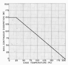
Fig. 3. Temperature vs power dissipation for 2N3789 transistor.
