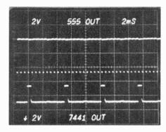
Fig. 3, 555 clock pulses and single output from the 7441.
