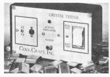
on the front of the tester and an LED indicates whether it is oscillating or not. An output socket is also available for connecting to a scope or meter for frequency check. No tuning is necessary. Operates from a 9-V battery and has a battery check position. Measures 61/4" × 33/4" × 21/4" (16 × 10 × 6 cm). \$56.
