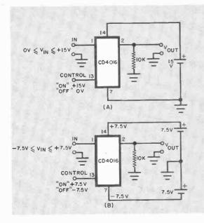
Fig. 2. The TG can switch positive dc signals (A) or bipolar signals (B), depending on power supply used.
