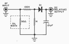
Power is dissipated by resistor in oil bath, while other components form a dc sampling circuit.
