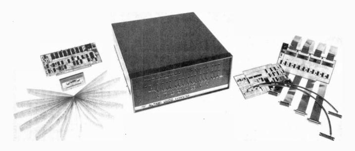
Computer. The Altair 8800 is the best-selling general-purpose computer in the world today. It is a parallel 8-bit word/16-bit address computer with an instruction cycle time of 2 microseconds. It was designed for almost unlimited peripheral and memory expansion, using a bus system where all input/output connections merge into a common line. The Altair 8800 is capable of addressing up to 65,536 words (bytes) of memory. Regularly priced at \$439 for a kit and \$621 assembled
