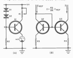
Fig. 1. In (A) reference voltage at X produces constant current in Q1. In (B) output I depends on reference current, R3, and R4.
