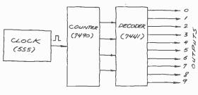
Fig. 1. Block diagram of sequence generator.
