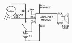
Fig. 1. Schematic diagram of a simple Photophone receiver.
