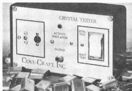
on the front of the tester and an LED indicates whether it is oscillating or not. An output socket is also available for connecting to a scope or meter for frequency check. No tuning is necessary. Operates from a 9-V battery and has a battery check position. Measures  $6\frac{1}{4}$ "  $\times$   $3\frac{3}{4}$ "  $\times$   $2\frac{1}{4}$ " (16  $\times$  10  $\times$  6 cm). \$56.
