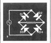
8. Which of the diodes in this full-wave bridge has been wired incorrectly.
