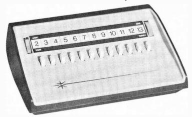
TRC-12 accessory provides TV receiver owners with an opportunity to add remote control of power, channel selection (vhf TV channels 2 through 13 only), and fine tuning without making internal circuit modifications or connections. The solid-state accessory operates without motors, gears, cams, belts, or any other mechanical parts at distances up to 25 ft (6.4 m) from any monochrome or color TV receiver to which it is connected.
