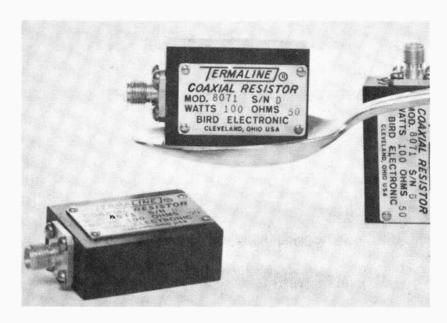
Bird's small dummy load can handle up to 100 watts from dc to 2 GHz, when heat-sinked to equipment panel.
