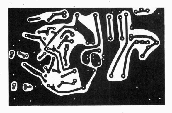
Fig. 3. Actual-size etching and drilling guide for pc board is shown above with component layout at right.
