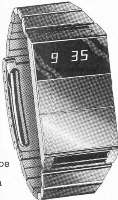
The Black Watch by Sinclair is unique. Controlled by a quartz crystal . . . powered by two hearing aid batteries . . . it's also styled in the cool prestige Sinclair fashion: no knobs, no buttons, no flash . . . just touch the front of the case to show hours and minutes and minutes and seconds in bright red LEDs.
