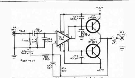
Fig. 2. First stage of amplifier is an integrated circuit.
