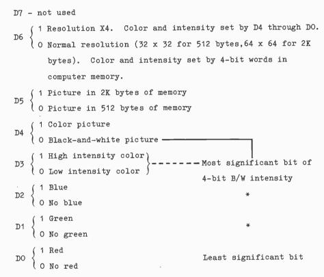
Fig. 3. The states of seven data bits at output port 017 determine resolution of TV picture and either chroma or monochrome parameters.
