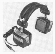
include: frequency range, 16 to 22,000 Hz; THD, less than 0.2% at 100 dB SPL; power handling capability, 400 mW per channel. Weighs 12 oz. \$50.00.
