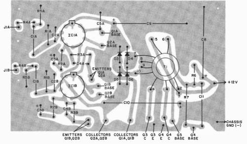
on the opposite side of the core from the primary leads 1 and 4 to facilitate matching the leads with their pads on the pc board. Label the ends of the feedback winding 5 and 6, taking careful note that current flowing from 5 to 6 should pass through the hole in the core in the same direction as current flowing from 1 to 2 or from 3 to 4 in the primary winding.
