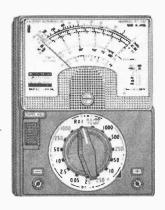
scales include 10/50/250/500/1000 V ac; 2.5/10/50/250/1000 V dc; .05/25/250 mA dc; 4000 and 400,000 ohms with 35-ohm midscale; and -20 to +62 dB. Sensitivity is 20,000 ohms/V dc and 10,000 ohms/V ac. Includes fuse, battery and test leads. Measures  $434^{\prime\prime}\text{H}\times314^{\prime\prime}\text{W}\times11^{11}/_{16}^{\prime\prime}\text{D}$  (12  $\times$  8  $\times$  4 cm) and weighs 9 oz.
