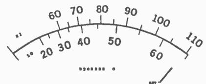
Fig. 2. Use this scale with the meter specified in Parts List to obtain an accuracy within 5°C.
