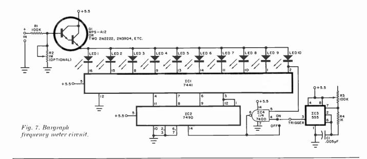
tary switch and several fixed precision resistors for *R1*, you can make a calibrated voltmeter which doubles as a resistance meter. In the resistance sensing mode, the circuit can be adjusted to indicate up to 10 megohms per LED.
