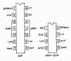
Fig. 1. Pin configurations for standard and miniature LM380.
