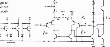
Fig. 1. The equivalent circuit diagram for the LM389 shows its versatility.
