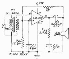
Fig. 5. An audio amplifier circuit with gain of 200.
