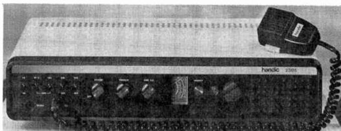
**T**HE Handic Model 2305 AM CB base-station transceiver features a striking low-silhouette packaging design. This gives it a long, lean look and allows all controls, meter, and channel indicator to be arranged in a functional horizontal line. Another feature that makes this transceiver "different" from most others on the market is that it has a built-in priority receiver that operates separately from
