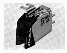
said to be 30 dB, and channel balance within 2 dB. Load resistance is 47,000 ohms, and load capacitance is 275 pF. The cartridge's stylus is a 0.4 mil × 0.7 mil elliptical diamond. Tracking force is from 2 to 5 grams, and cartridge weight is 5.5 grams. The Stanton 680EL comes with a replacement stylus. \$90.00
