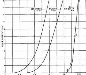
Fig 3. Curves show dependence of resistance on applied voltage, as well as temperature for diodes.
