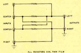
Fig. 3. Passive mixer uses six 33,000-ohm resistors, utility box and six line jacks.
