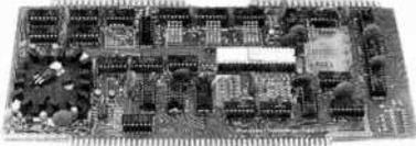
The **3P+S** module from **Processor Technology** is the most versatile input-output card for your Sol, IMSAI, or Altair system. It has **two 8-bit parallel I/O ports**, with full handshaking logic, **and a serial I/O port**. All on a single card.
