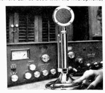
which is wired with an open audio line on receive. Its coiled cable has one shielded conductor and four unshielded. All external parts, including the base, are chrome plated.
