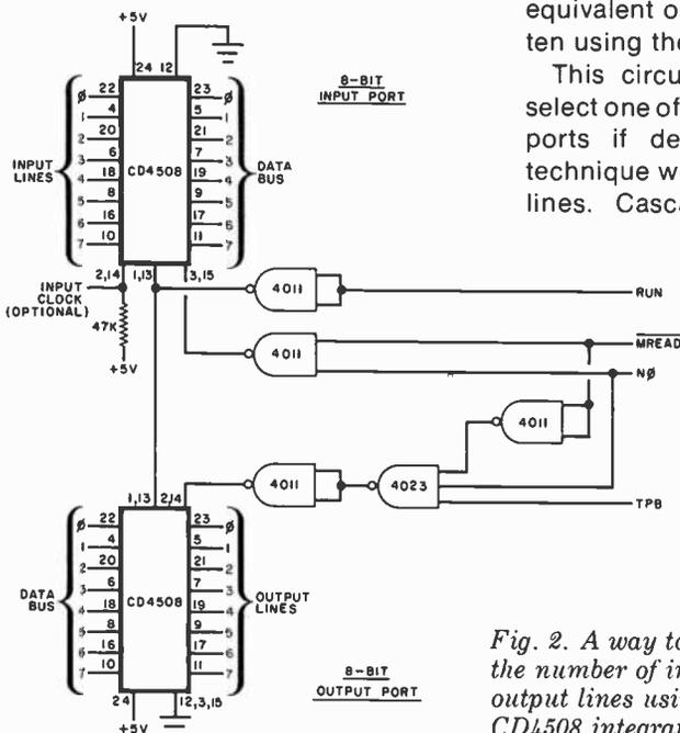
Fig. 2. A way to expand the number of input and output lines using two CD4508 integrated circuits.
