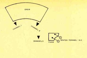
Fig. 2. Miking techniques used for recording a choir include piano at right.
