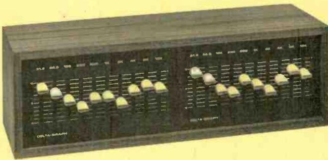
*\$130 stereo kit features modular design, artificial inductors, and 10-octave control.*
