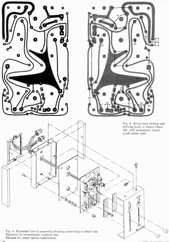
The triac (Q3) specified in the Parts List has an electrically isolated heatsink tab that can be bolted to the metal cover to provide good heat sinking. If you use any other type of triac, an insulating mounting kit will be required.
