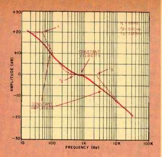
Fig. 4. RIAA playback equalization compensates for the recording characteristic that was shown in Fig. 1.
