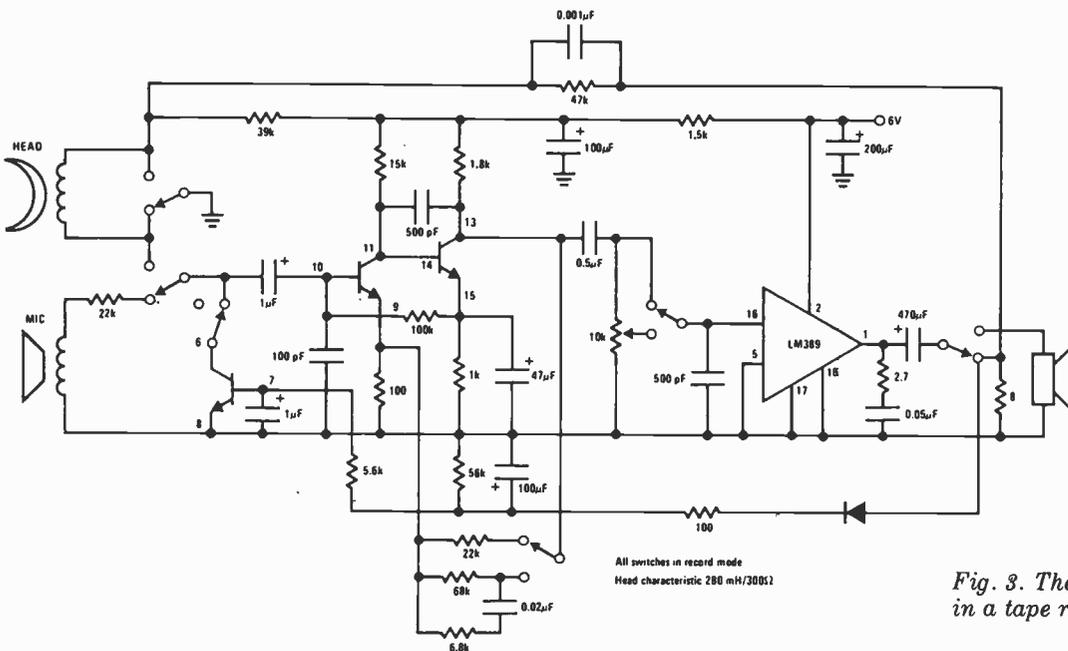
Fig. 3. The LM389 used in a tape recorder circuit.
