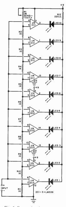
Fig. 5. Bargraph using comparator voltage and resistance-sensitive circuit.
