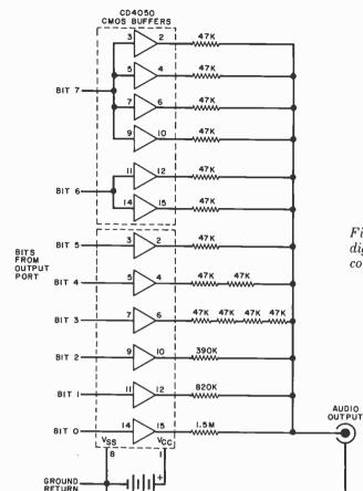
Fig. 4. Simple 8-bit digital-to-analog converter.
