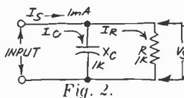
required that the output voltage be down by only a very small amount? In this case,  $X_c$  would have to be no more than  $0.1R$ . Hence, a ten-fold increase in the value of  $R$ , to 265,000 ohms, is indicated.
