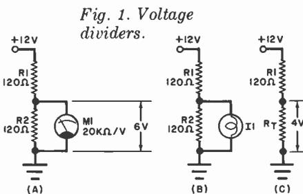
stantially less than 6 V. What has happened, of course, is that the effective resistance of the lamp in parallel with  $R_2$  has dropped so that the voltage across the combination is not sufficient to light the lamp. The lamp is rated at 6 volts and 50 mA, which means a resistance of 120 ohms. The combination of the lamp and  $R_2$  thus gives a total resistance of 60 ohms and the voltage across the combination is 4 V (Fig. 1C).
