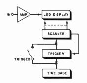
Fig. 6. Block diagram for bargraph frequency meter.
