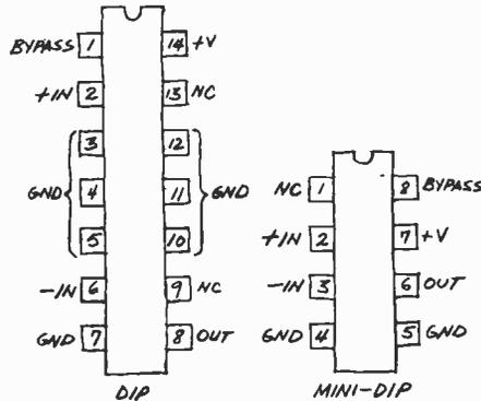
Fig. 1. Pin configurations for standard and miniature LM380.
