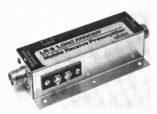
inserted in the transmission line between transceiver and antenna, a carrier detection circuit isolates the preamp on transmit. Requires 12 V dc, positive or negative ground. \$29.95
