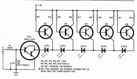
Fig. 4. Transistors can be used to switch on a series string of LED's in succession as in this circuit.
