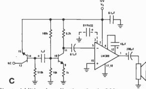
Fig. 4. Additional applications for the LM389 include: (A) a siren circuit; (B) a voltage-controlled amplifier with tremolo; and (C) a noise generator circuit.
