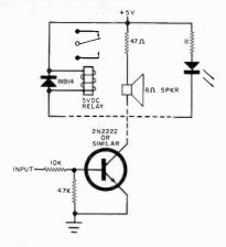
Fig. 5. Circuit to provide outputs used for testing.
