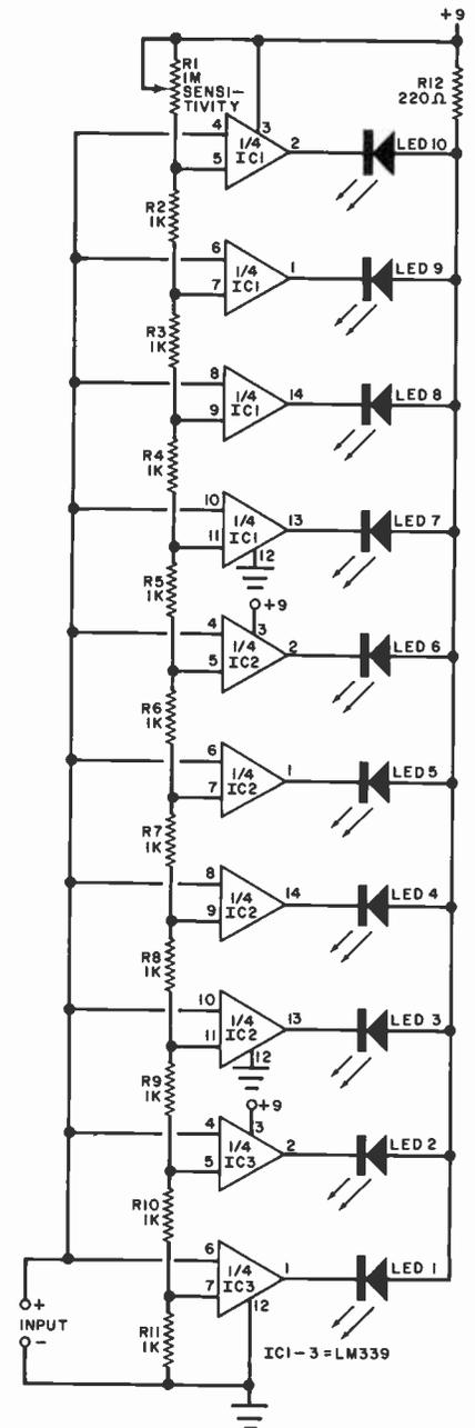
Fig. 5. Bargraph using comparator voltage and resistance-sensitive circuit.
