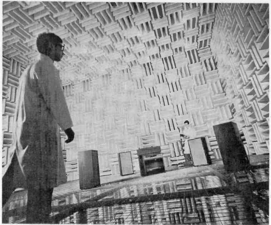
Fig. 2. JVC's unusually large anechoic chamber.
