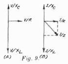
gram can be simplified as in Fig. 9B. Hence, the impedance formula is  $Z=1/\sqrt{(1/R)^2+(1/X_{\rm C}-1/X_{\rm L})^2}$ . Now you can calculate Z for the Fig. 10 circuit:
