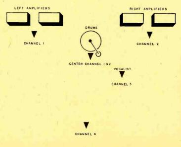
Fig. 1. Typical setup for recording a band.
