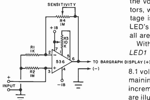
Fig. 2. Bargraph readout with op amp input.
