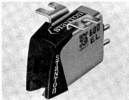
said to be 30 dB, and channel balance within 2 dB. Load resistance is 47,000 ohms, and load capacitance is 275 pF. The cartridge's stylus is a 0.4 mil  $\times$  0.7 mil elliptical diamond. Tracking force is from 2 to 5 grams, and cartridge weight is 5.5 grams. The Stanton 680EL comes with a replacement stylus. \$90.00
