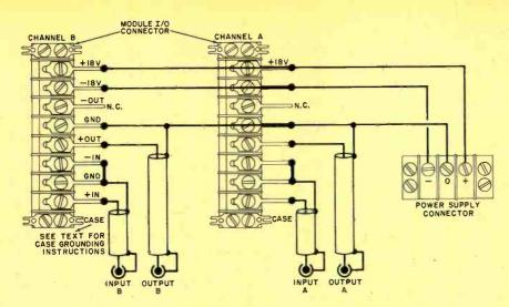
Fig. 4. Wiring scheme for home audio system is shown here with stereo setup. For mono, eliminate channel B; for 4-channel add channels C and D in same manner as shown for channel B to channel A.
