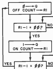
This program will flash the Q LED and put a square wave on the Q line at a rate determined by the contents of memory M (0002) from a 10 to some other number. By referring back to the Instruction Subset Table in last month's article, you should be able to interpret the above program.
