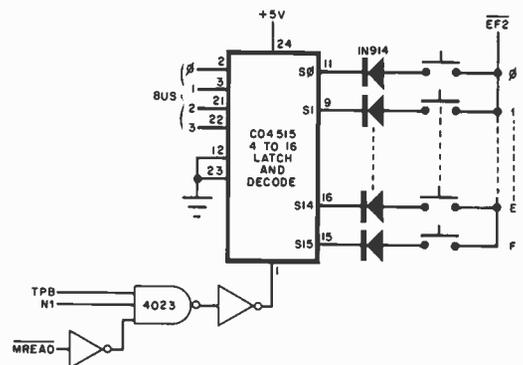
Fig. 3. A method of controlling up to 16 outputs.
