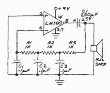
Fig. 4. LM380 phase-shift oscillator produces shrill tone.
