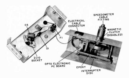
Fig. 5. Assembly of the speedometer and optoelectronic unit.
