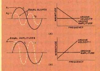
Fig. 3. In constant-velocity recording (A), groove amplitude varies with frequency. In constant-amplitude recording (B), groove velocity varies with frequency.
