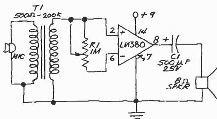
Fig. 2. Simple audio amplifier circuit using an LM380.
