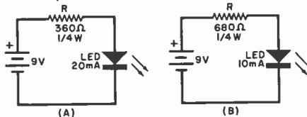
Fig. 2. LED circuits.
