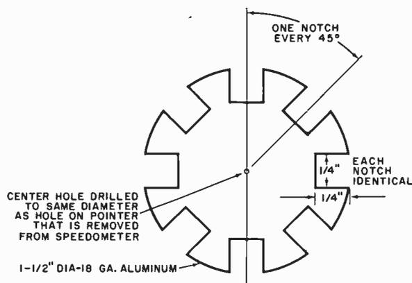
Fig. 4. Use this diagram to make interrupter disc.
