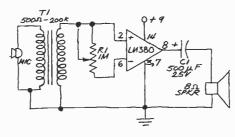
Fig. 2. Simple audio amplifier circuit using an LM380.
