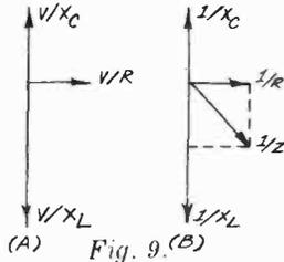
gram can be simplified as in Fig. 9B. Hence, the impedance formula is  $Z = 1/\sqrt{(1/R)^2 + (1/X_C - 1/X_L)^2}$ . Now you can calculate Z for the Fig. 10 circuit:
