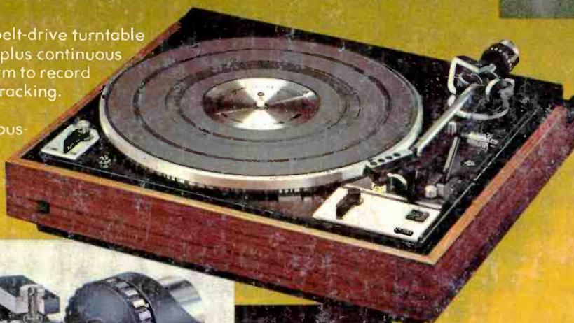
True, four-point gimbal centers and pivots the effective mass at intersection of horizontal and vertical axes. Tonearm is dynamically balanced in all planes. The four needle-point pivots are first hardened, then honed, a process which produces microscopically smooth surfaces. The precision ball-bearing races are only 0.157 inch diameter.
