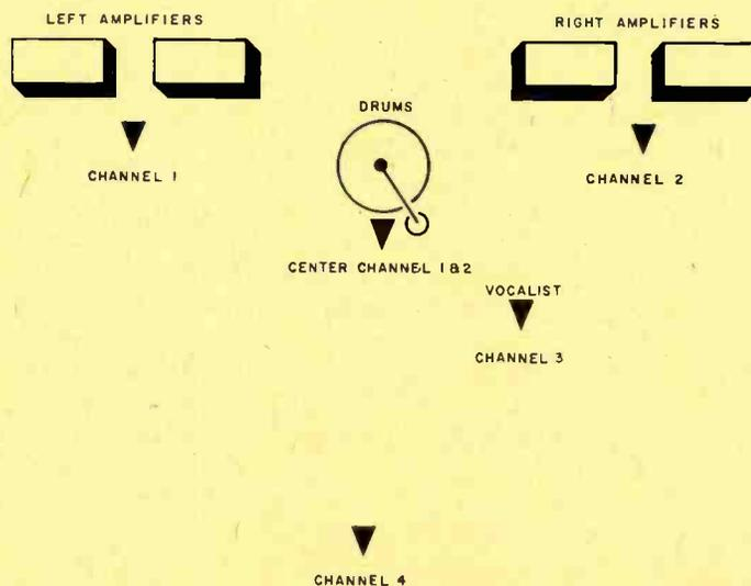
Fig. 1. Typical setup for recording a band.
