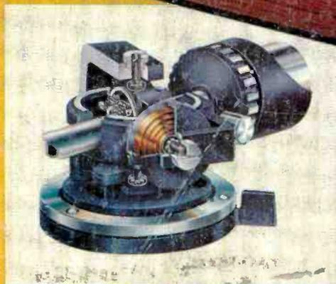
Unique "Vario-pulley" used in Dual's three belt-drive models is precision-machined for perfect concentricity and balance. Speeds are adjusted by expansion and contraction of pulley circumference; belt is never twisted or distorted.
