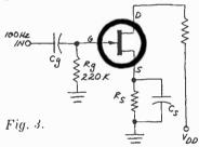
capacitor  $C_{\rm s}$  prevents feedback that could cause a loss of gain in the stage.
