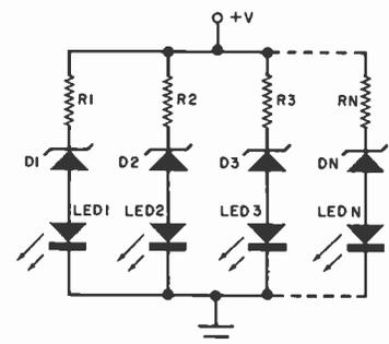
Fig. 3. Zener diode voltage-sensitive bargraph.
