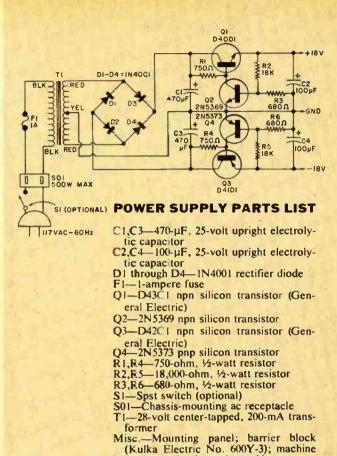
Fig. 2. Power supply accommodates up to four equalizer modules.
