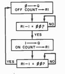
This program will flash the Q LED and put a square wave on the Q line at a rate determined by the contents of memory M (0002) from a 10 to some other number. By referring back to the Instruction Subset Table in last month's article, you should be able to interpret the above program.
