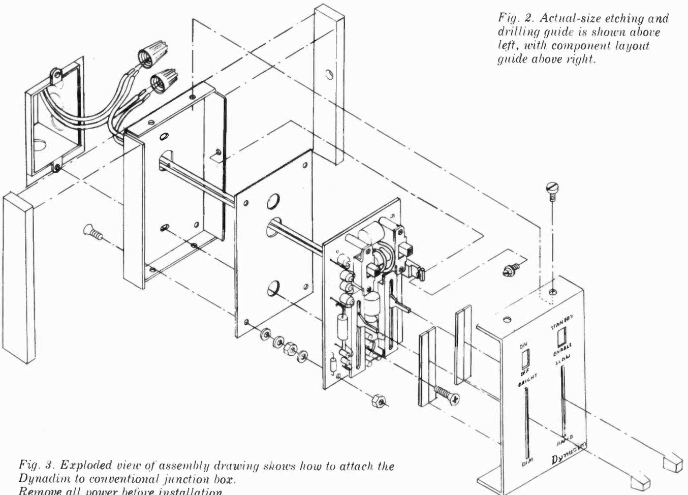
Fig. 3. Exploded view of assembly drawing shows how to attach the Dynadim to conventional junction box. Remove all power before installation.
