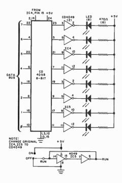
Fig. 1. Circuit for a discrete LED display.
