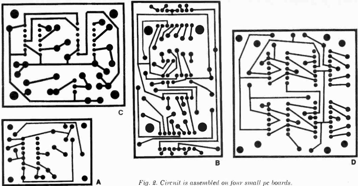
Fig. 2. Circuit is assembled on four small pc boards. Etching and drilling guides are shown above. Optoelectronic board (A) is fitted to the speedometer chassis. Display board (B) is mounted on front panel of display chassis with other two boards (C & D) inside the display chassis. Component layouts are shown below. Solid lines between solder pads are jumpers.
