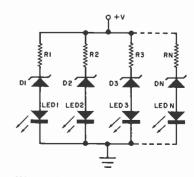
Fig. 3. Zener diode voltage-sensitive bargraph.
