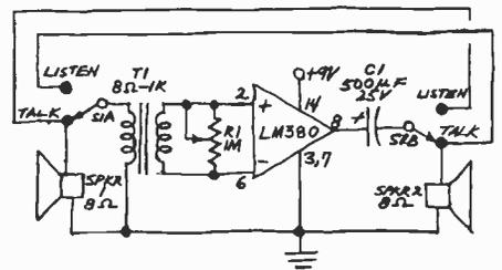
Fig. 3. Circuit for elementary two-way intercom system.
