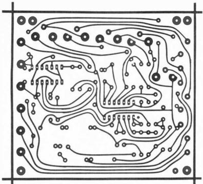
Fig. 2. Actual-size etching and drilling guide (above) and component placement guide (below) for printed circuit board.
