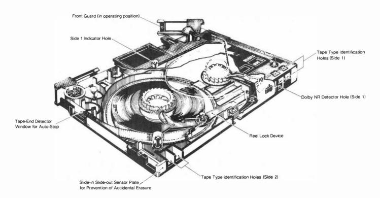
Fig. 3. Structural features of the new Elcaset. Format includes provisions for automatic switching of bias, etc.
