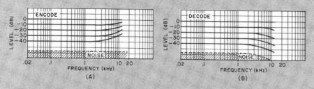
Fig. 1. Dolby-B noise reduction uses level-sensitive pre-emphasis on record (A) and complementary de-emphasis on playback (B).
