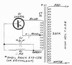
Fig. 1. Simple dc/dc converter.
