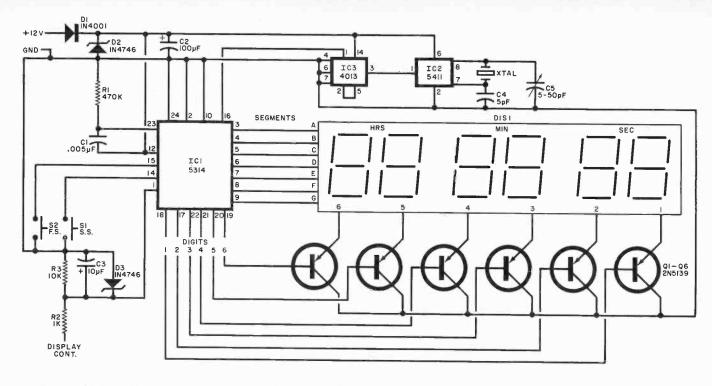
Fig. 1. Crystal oscillator is counted down by IC2 and IC3 to drive clock circuit in IC1.
