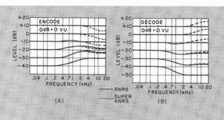
Fig. 2. Record (A) and playback (B) characteristics for JVC's new Super ANRS, It has high-level treble compression to avoid tape saturation.
