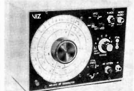
positions for 455 kHz and 10.7 MHz sweep outputs for AM and FM radio i-f alignment. R-f output is rated at 75 mV minimum. The generator has a built-in modulator and a crystal controlled oscillator circuit with front-panel crystal socket for markers or calibration. A two-step 10:1 attenuator switch is included, as are a vernier attenuation control for sweep output, and a two-position 7:1 attenuator switch for crystal oscillator output. Measures 7¾" x 5⅞" x 4⅞" (19.7 x 14.9 x 10.5 cm). \$117.00.
