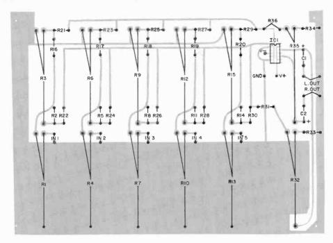
Fig. 2. The actual size etching and drilling guide for the printed circuit board is shown on the opposite page. Layout of componants on the board is above.
