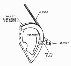
Fig. 3. Metal flag, % in. by ¼ in. is attached to rim of harmonic balancer pulley to pass through slot in sensor interrupting light beam.
