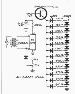
potentiometer and diode between the transformer and rectifier assembly are optional. If used, however, they will compensate for the initial forward drop of the diode junctions.
