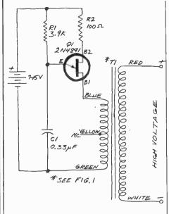
Fig. 3. UJT dc/dc converter.
