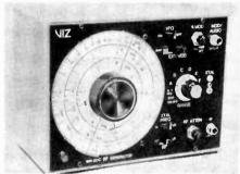
positions for 455 kHz and 10.7 MHz sweep outputs for AM and FM radio i-f alignment. R-f output is rated at 75 mV minimum. The generator has a built-in modulator and a crystal controlled oscillator circuit with front-panel crystal socket for markers or calibration. A two-step 10:1 attenuator switch is included, as are a vernier attenuation control for sweep output, and a two-position 7:1 attenuator switch for crystal oscillator output. Measures 7¾" × 5½" × 4½" (19.7 × 14.9 × 10.5 cm). \$117.00.
