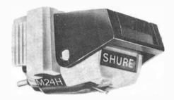
50,000 Hz, its output 3.0 mV per channel at 1000 Hz with a 5 cm/sec peak recorded velocity, and channel balance within 2 dB. Channel separation is rated at a minimum of 22 dB at 1000 Hz. Typical trackability at 1¼ grams in a Shure/SME tone arm is 20 cm/sec at 400 Hz and 25 cm/sec at 30,000 Hz, with a peak of 50 cm/sec at 10,000 Hz. Tracking force ranges from 1 gram minimum to 1½ grams maximum, with an optimum figure of 1¼ grams. Net weight is 6 grams. \$74.95.
