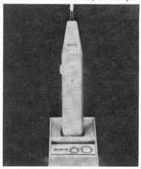
a LED indicator lights. The iron can be kept in its recharging stand, where it will be trickle-charged if the battery is not discharged or fast-charged if it is low. The standard cordless soldering kit, Model 7800, includes the Iso-Tip 60 soldering iron, recharging stand, a fine tip, a chisel tip, and an instruction booklet. The iron will also accommodate any of Wahl's 16 snap-in soldering tips.
