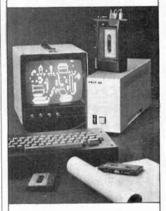
The POLY 88 System uses a video monitor for display, a keyboard for input and cassette tape for storage. The system will also connect to a hard-copy terminal. Poly 88 hardware consists of an 8080 based CPU circuit card with onboard memory and I/O, video display circuit card with keyboard input port and graphics capability, and mini-cards that connect to the CPU board via ribbon cable for cassette or serial interface.
