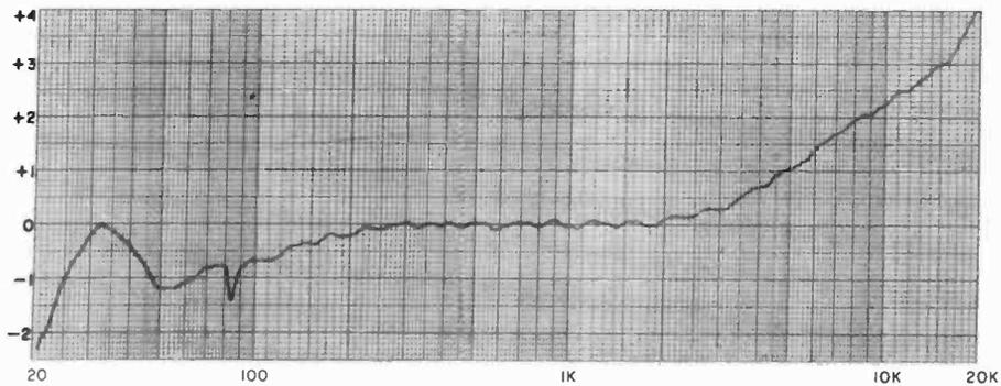
Fig. 9. Scotch Classic at 15 ips and minimum equalization.
