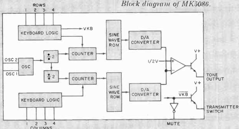
Each sine-wave synthesizer is formed by a 5-bit, 32-state counter, decode ROM, and R-2R ladder network D/A converter. The output of each D/A converter
