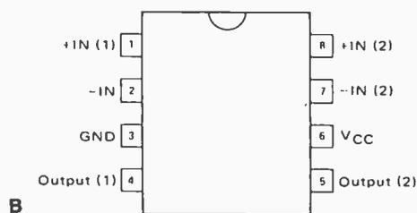
Fig. 5. Equivalent schematic (A) and pin connections (B) for LM387.
