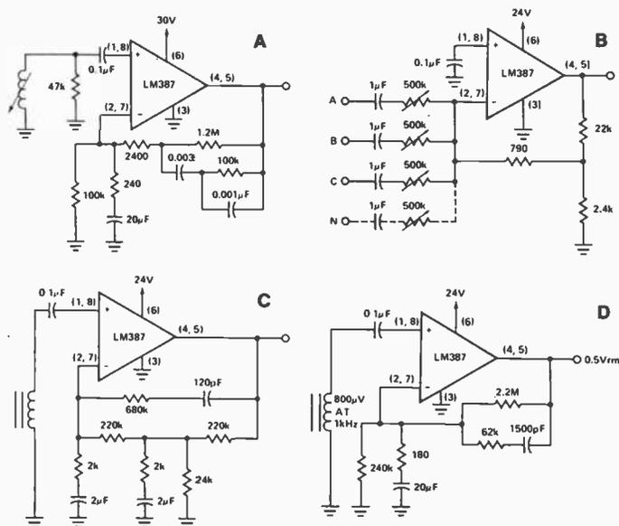
Fig. 6. Applications for the LM387 preamplifier.
