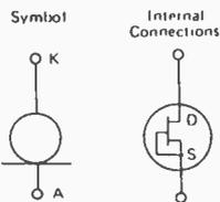
Fig. 1. The constant-current diode.
