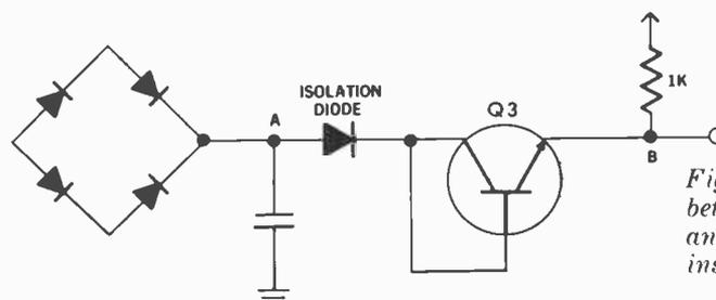
Fig. 3. Isolation diode between filter capacitor and transistor permits instantaneous reset.
