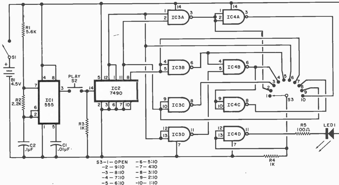
In the circuit, IC1 operates at 1000 Hz, S2 starts the play, and S3 determines the odds.
