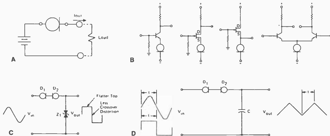
Fig. 2. Some applications for the constant-current diode.
