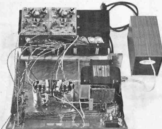
*The "Double 400" is an augmentation of Dynaco's Stereo 400 power amplifier.*
