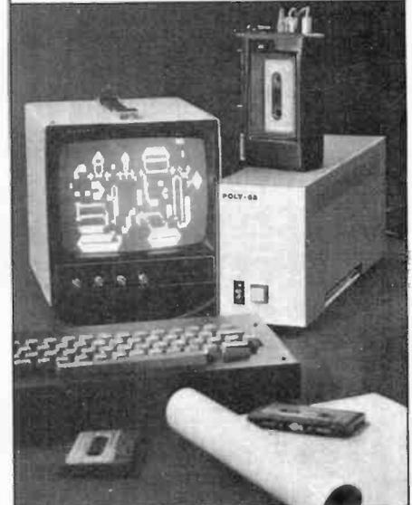
The POLY 88 System uses a video monitor for display, a keyboard for input and cassette tape for storage. The system will also connect to a hard-copy terminal. Poly 88 hardware consists of an 8080 based CPU circuit card with on-board memory and I/O, video display circuit card with keyboard input port and graphics capability, and mini-cards that connect to the CPU board via ribbon cable for cassette or serial interface.
