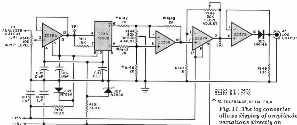
Fig. 11. The log converter allows display of amplitude variations directly on the scope in decibels.
