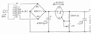
Fig. 2. Five-volt TTL power supply.
