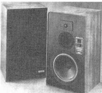
4½" (11.4-cm) midrange driver, and 1" (2.54-cm) tweeter. The system is housed in a lacquer-finished walnut-veneer cabinet that measures 24¾" x 13¾" x 11¾" (61.9 x 34.9 x 30 cm) and weighs 47 lb (21.3 kg). Behind the removable black fabric grille are three-position midrange and high-frequency controls that provide nine different contour setting combinations.
