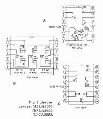
and a differential cascode amplifier using super-beta devices. It is especially useful as a high impedance transducer amplifier or in long-interval timer applications.
