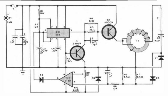
Fig. 1. The 555 oscillator drives Q2 which causes a high voltage across the lamp through T1. The IC2 circuit is a form of voltage regulator.
