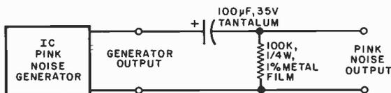
Fig. 13. Modifying the IC pink noise generator for use with the RTA.
