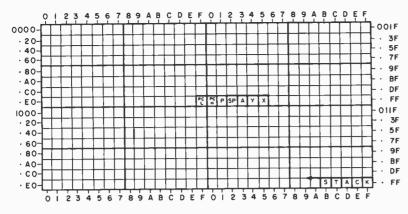
Fig. 5. Overlay mask for the KIM-1. All internal registers are displayed simultaneously with the entire stack.
