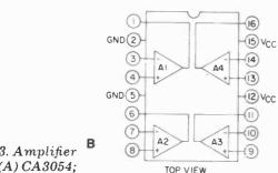
Fig. 3. Amplifier arrays: (A) CA3054; (B) CA3048/CA3052.
