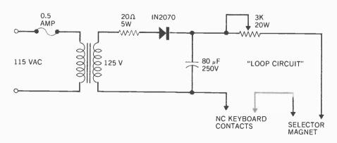
Fig. 6. Local copy can be obtained using the loop circuit shown here.
