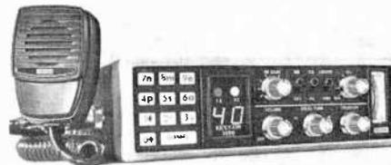
SBE Key-Com 1000 has built-in microprocessor and a calculator type keyboard channel selector.
