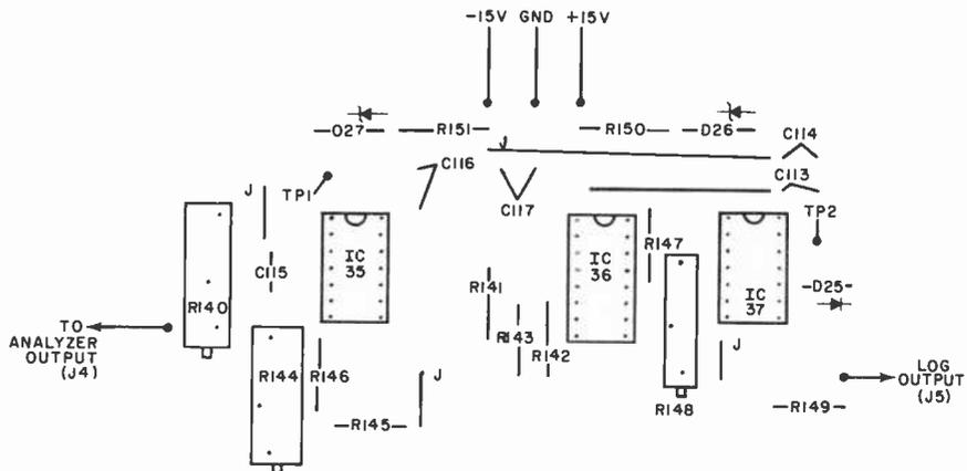
Fig. 12. Etching and drilling guide for the pc board is at right. Component layout shown above.
