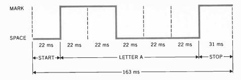
Fig. 1. Waveform showing the pulse sequences that make up the letter "A".
