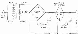
Fig. 3. Variable 0-5-volt power supply.
