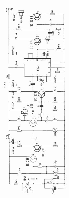
Fig. 4. The Siemens FM infrared receiver uses a 4046 integrated circuit as a wide-band FM demodulator.
