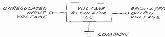
Fig. 1. Basic 3-terminal IC voltage-regulator power supply circuit.
