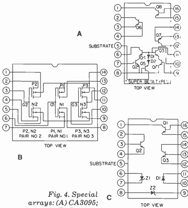
Fig. 4. Special arrays: (A) CA3095; (B) CA3600; (C) CA3093.
