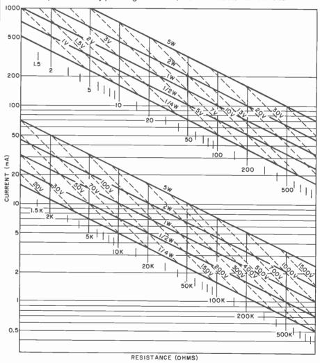
current as well as the minimum resistance required for a given voltage drop to be applied safely across it. In addition, the nomograph tells what the wattage rating for a given resistor should
