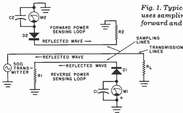
Fig. 1. Typical SWR meter uses sampling lines to detect forward and reflected waves.
