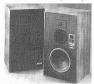
4 %'' (11.4-cm) midrange driver, and 1" (2.54-cm) tweeter. The system is housed in a lacquer-finished walnut-veneer cabinet that measures  $24 \%'' \times 13 \%'' \times 11 \%''$  (61.9  $\times$  34.9  $\times$  30 cm) and weighs 47 lb (21.3 kg). Behind the removable black fabric grille are three-position midrange and high-frequency controls that provide nine different contour setting combinations.
