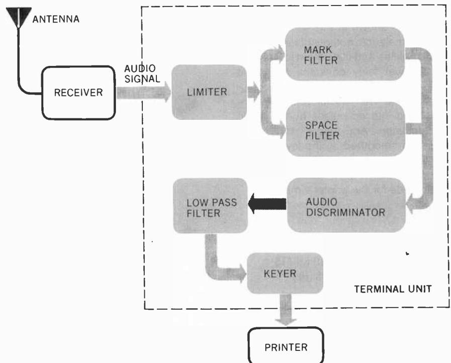
Fig. 4. Block diagram of typical audio terminal unit.
