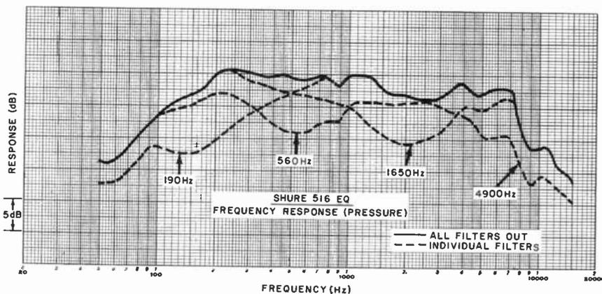
*Frequency response (pressure) with all filters out and with individual filters in.*
