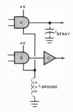
Fig. 1. Common ground inductance and stray capacitance cause "glitch" at output gate of C.
