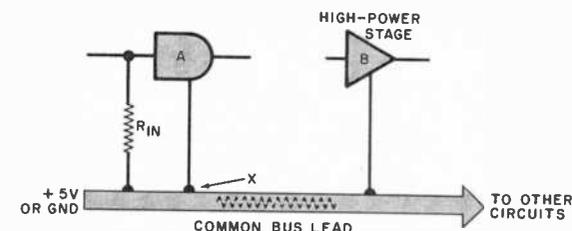
Fig. 2. Both glitch and voltage drop can occur along a common bus lead as shown here.
