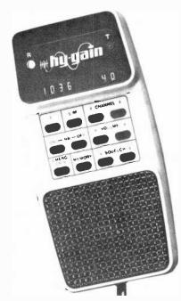
URING the past year or so, a number of mobile CB transceivers have been designed to be operated by remote control, with the transceiver itself located somewhere other than under the dashboard. The operating controls for such rigs are on the case of the microphone, which generally serves as the speaker, and is connected to the transceiver via a detachable cable. This type of setup permits the transceiver to be installed in a hidden location to minimize the possibility of theft.
