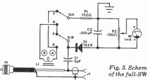
Fig. 3. Schematic diagram of the full-SWR meter.
