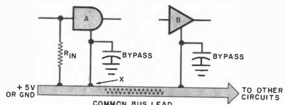
Fig. 3. Bypassing can eliminate glitch but not voltage change which produces erroneous signal.
