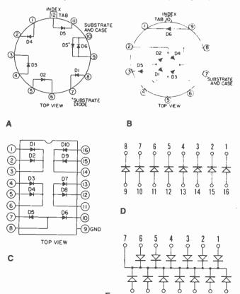
Fig. 1. Typical diode arrays: (A) CA3039; (B) CA3019; (C) CA3141; (D) FSA2619M; (E) FSA2565M.
