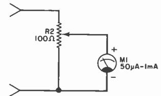
Fig. 5. Alternate meter wiring.
