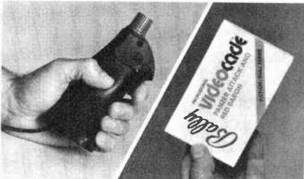
The cassette cartridges add between eight to thirty-two thousand additional bytes of computer power to the basic 12,000 byte system. The pistol grip arcade accessory can be used to play all the arcade games.
