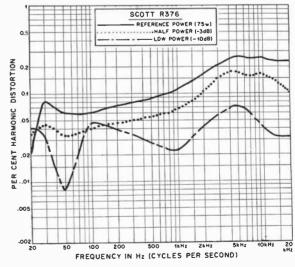
Harmonic distortion at three power levels.
