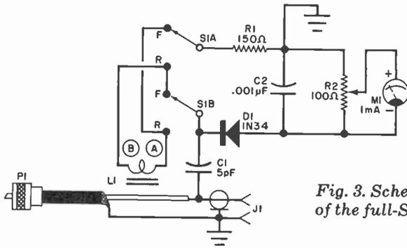
Fig. 3. Schematic diagram of the full-SWR meter.
