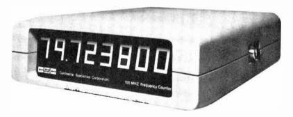
EW TEST instruments are as simple to operate as the Model MAX-100 frequency counter from Continental Specialties Corp. It is devoid of all controls except a power on/off switch. You simply turn on the power and connect the instrument's input cable to the circuit under test. Unlike most other low-cost counters that have a frequency range of 30 MHz and a four- or six-digit numeric display, the MAX-100 goes out to 100 MHz and indicates the frequency directly on its eight-digit display.
