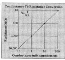
Beginner or pro, you'll find the meter you now have can't measure nanosiemens. So what? With the 8020A conductance function, you can measure the equivalent of 10,000 megohms in nanosiemens. Like capacitor, circuit board and insulation leakage. And, you can check transistor gain with a simple, homemade adapter. Only with the 8020A, a 13-oz. heavyweight that goes where you go, with confidence.
