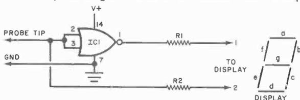
Fig. 8. Reader's logic probe circuit.
