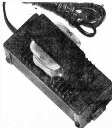
Fig. 4. Photo of assembled prototype shows transformer mounted on heat sink.
