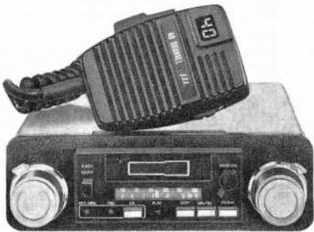
trol. The latter monitors CB while listening to cassettes or radio. Whenever a message comes through on a selected CB channel the circuit interprets the program then returns to it automatically at the end of the CB transmission. The cassette section includes controls for fast forward/eject and tape play indicator. The audio section delivers 5 W/ch rms power output at a frequency range of 50-10,000 Hz. \$369.95.
