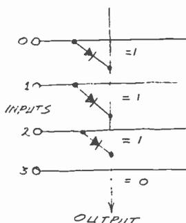
Fig. 2. 4X1 PROM programmed for 2-input NAND gate.
