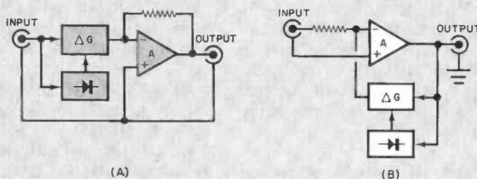
Fig. 3. Using the NE570 as an expander (A) and compressor (B).
