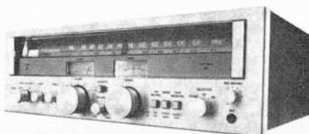
ultrasonic carrier. Harmonic distortion is rated a 0.18% monaural, 0.25% stereo. The phono preamp uses low-noise pnp Darlington transistors. Other features include microphone mixing with level control, signal strength and zero-center tuning meters, AM beat filter, loudness switch, tape monitor, FM muting, headphone jack, and a speaker selector switch. Measures 17 1/16" W x 13 15/16" D x 6 1/16" H (43.3 x 35.4 x 15.4 cm). \$280.
