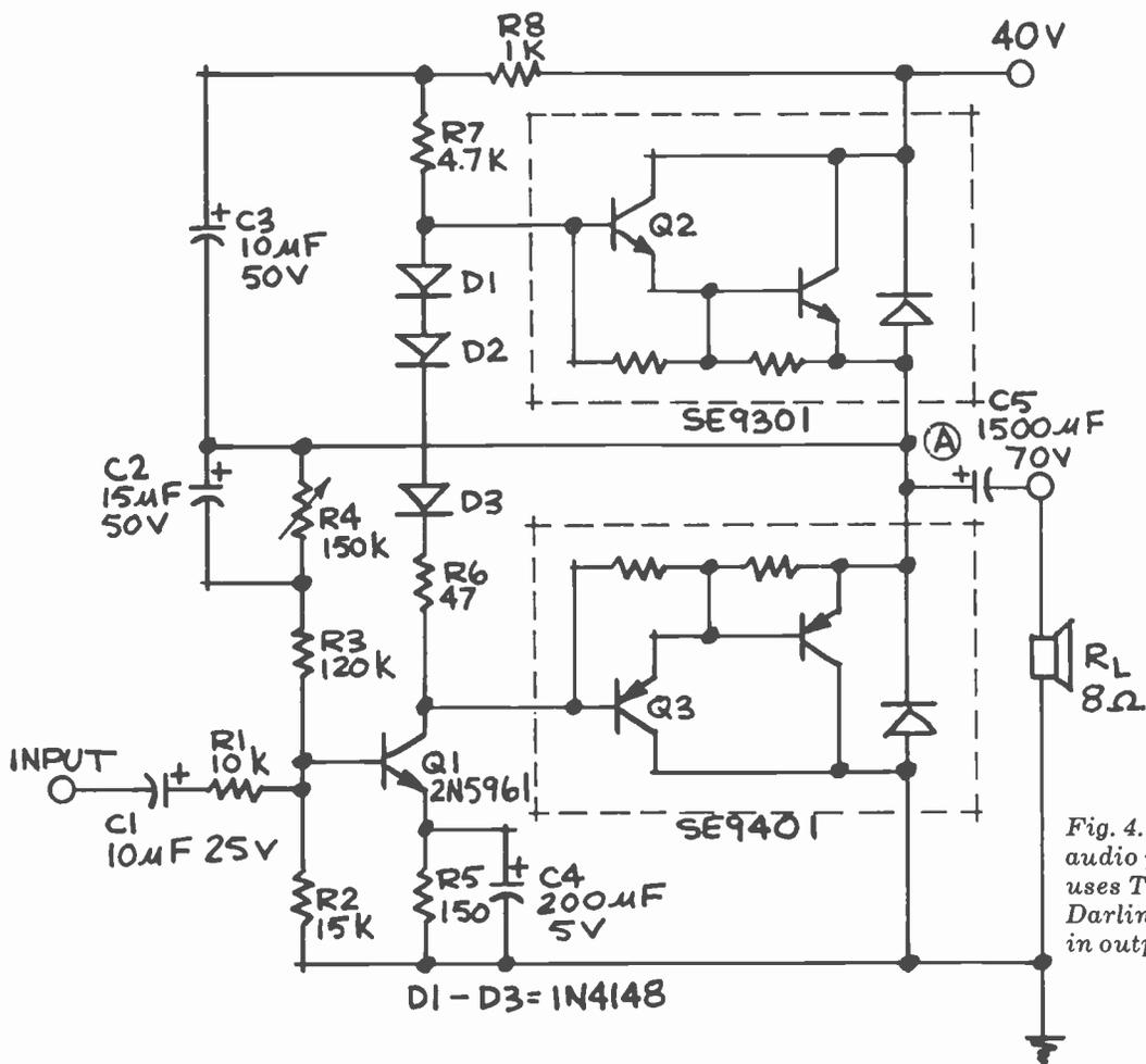
Fig. 4. Complementary audio power amplifier uses TO-220 monolithic Darlington transistors in output stage.
