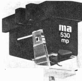
response is 5 to 20,000 Hz  $\pm$  1 1/4 dB. Tracking force range is 0.7 to 1.4 grams, and cartridge weight is 4 grams. Claimed channel separation is 30 dB at 1000 Hz, 15 dB at 10,000 Hz. Output voltage is 3.5 mV each channel at 5 cm/s peak recorded velocity. Load requirements and cable capacitance are specified at 10,000 to 100,000 ohms and 100 to 1500 pF, respectively. Each stylus is light-beam oriented under a microscope. \$200.
