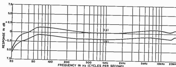
*Fig. 2a and b. In (a), at top, Maxell gave its new UD XL-I tape (A) more output than older UD (B), but same response. In (b), below, new TDK AD tape has more high-end response (A) than earlier Audua (B).*
