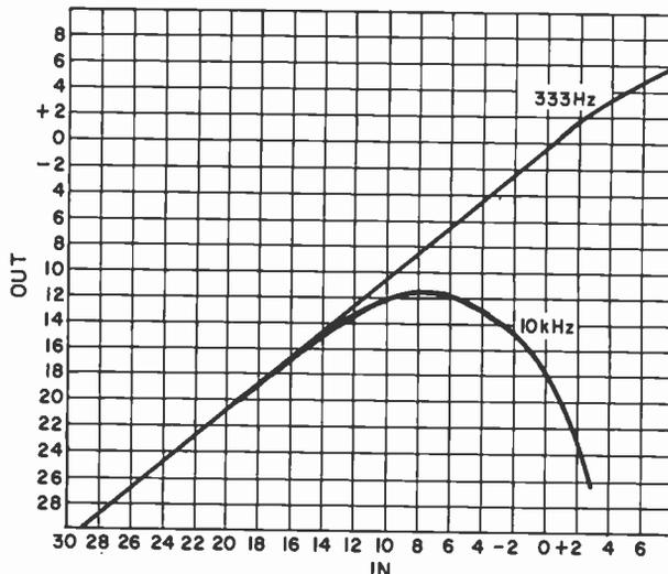
a few moments of it, flipping between "source" and "tape;" see which tape comes closest to matching the original sound. If you try this, however, remember to maintain the record level 10 to 20 dB below 0 VU on your recording meters. The high-frequency energy in the hiss signal would otherwise drive the
