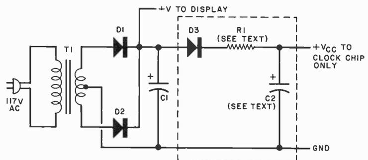
*This circuit provides power to a clock chip to prevent flicker.*
