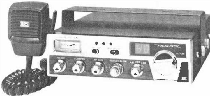
**T**HE Realistic Model TRC-449 from Radio Shack is an AM/SSB transceiver designed for mobile communication on the Citizens Band. Its 40-channel coverage is obtained from the now-familiar phase-locked-loop (PLL) digital frequency-synthesis system. Large red LED-type seven-segment numeric indicators are used to identify the channel selected.
