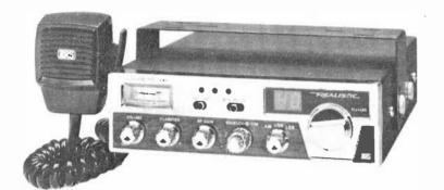
THE Realistic Model TRC-449 from Radio Shack is an AM/SSB transceiver designed for mobile communication on the Citizens Band. Its 40-channel coverage is obtained from the nowfamiliar phase-locked-loop (PLL) digital frequency-synthesis system. Large red LED-type seven-segment numeric indicators are used to identify the channel selected.
