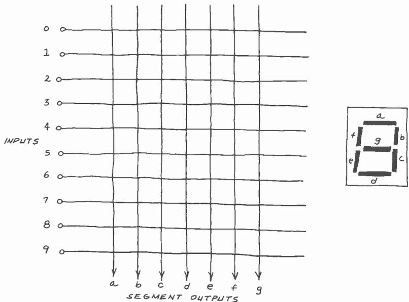
Fig. 5. Seven-segment display character generator diode PROM.
