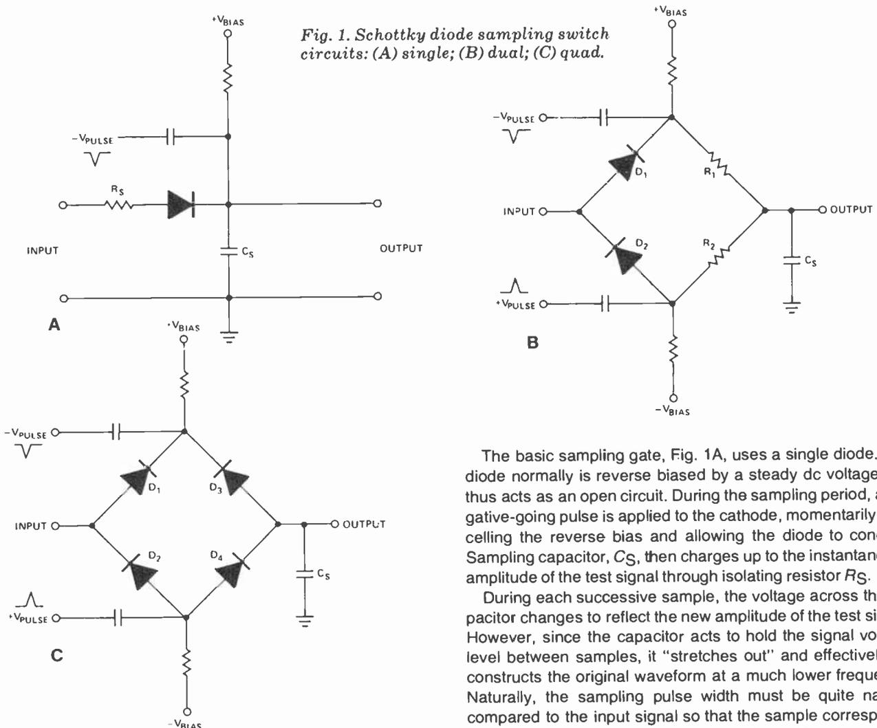
The basic sampling gate, Fig. 1A, uses a single diode. The diode normally is reverse biased by a steady dc voltage and thus acts as an open circuit. During the sampling period, a negative-going pulse is applied to the cathode, momentarily cancelling the reverse bias and allowing the diode to conduct. Sampling capacitor,  $C_S$ , then charges up to the instantaneous amplitude of the test signal through isolating resistor  $R_S$ .
