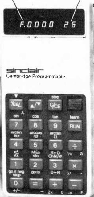
it means that  $\square$  is programmed as step 26. If step 26 should have been  $\oplus$ , all you have to do is press
