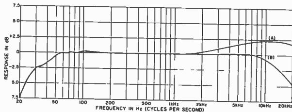
*Fig. 1. Results of improper bias vary: (A) DIN bias settings used with typical Japanese ferric tape over-emphasize highs due to underbiasing. (B) Correct bias for same tapes over-biases DIN ferric tapes.*
