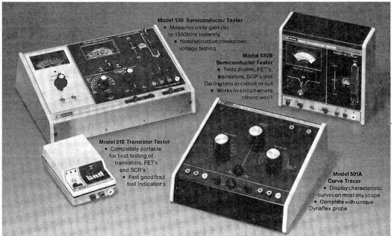
The B&K-PRECISION Model 530 is one of the most versatile semiconductor testers available and can actually perform more tests on more devices than any instrument in its price class. Features include: Exclusive patented  $f_T$  measurement circuit... Non-destructive breakdown voltage testing... Automatic lead and polarity identification, in- or out-of circuit... Measurement of beta and gm... Aural and visual test indications... Testing of new power FET's. CSA listed. **\$310**
