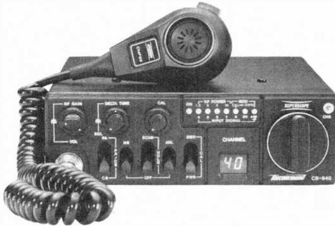
**T**HE Superscope Aircommand 40-channel mobile AM CB transceiver departs from convention, as do a few others, by indicating relative signal strength, output power, etc., with a row of LED's instead of a meter. Another special feature is channel 9 scanning with individual squelch control and an audible alarm that sounds whenever a signal appears on channel 9.
