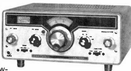
An excellent, low-cost choice for your first receiver is the HR-1680. With it you'll find total solid-state construction, no-instrument alignment, and a sensitivity figure of less than 0.5  $\mu$ V. It covers 80, 40, 20, 15 and the lower 1 MHz of 10 meters. And with a MOSFET "front end" and preselector tuning — you'll be digging out the "rare" ones in no time!
