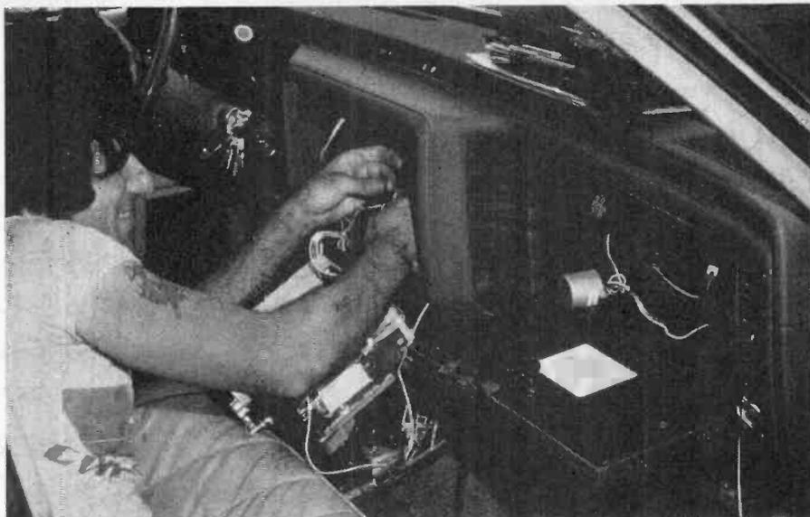
Installing a mobile CB rig is not usually a major undertaking. It can be challenging, though, when an AM/FM electric-powered antenna is replaced by a CB/AM/FM one since auto radio must be removed to make power connections.
