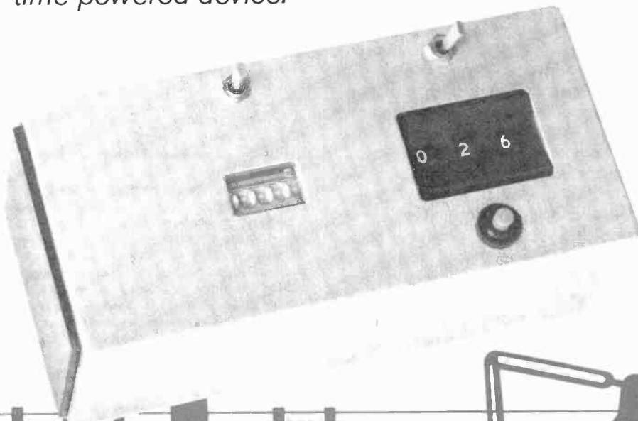
**A** DARKROOM or other precision-application timer should possess the following attributes: accuracy; precise repeatability; provisions for setting the timing interval in minutes and seconds or hours and minutes; and a method of displaying elapsed time clearly in low ambient light levels. Most commercially available timers are electromechanical devices which fall short in one or more of the cited areas. The "Digital Darkroom Timer" described here, however, offers all of these features.
