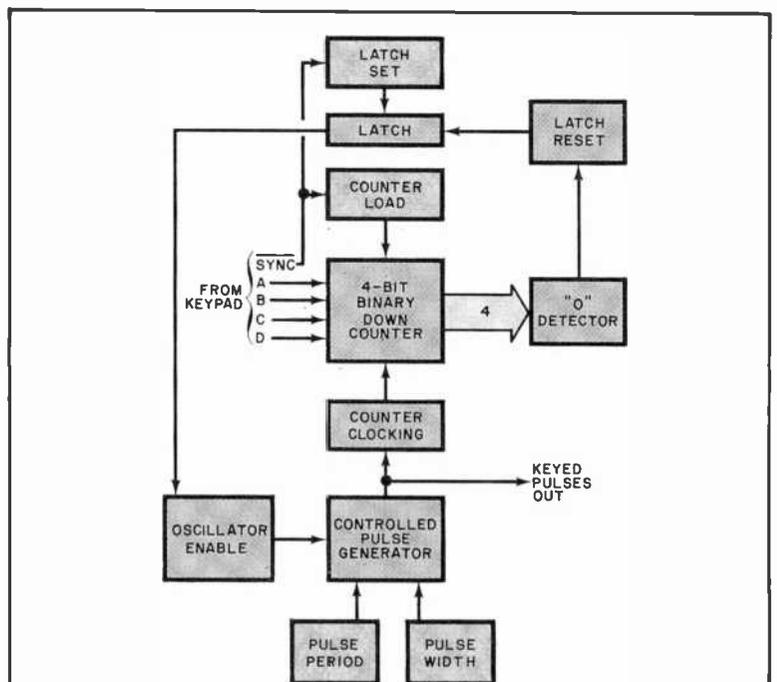
Fig. 5. Function diagram for a controlled-pulse generator.
