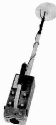
"Cointracker," has been introduced by Heath Company. It features adjustable discrimination, pushbutton tuning, waterproof search coil, and the length of its collapsible shaft is adjustable. Metal detection is signaled to the user via a built-in meter and through an adjustable-volume headphone output. A battery recharging jack is also provided. Weight is 3.5 lb (1.6 kg). \$149.95.
