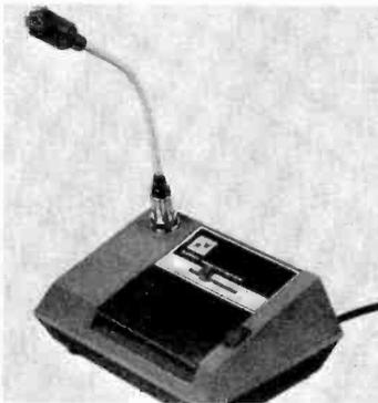
Power for the M-611 is provided by a self-contained "C" cell. The interchangeable microphone stem allows use of lapel microphone and acoustic tube microphone headset plug-in modules. Frequency response of the new Superex microphone is claimed to be 250-8000 Hz; sensitivity is rated at -45 dB. Comes with a 6' (1.8 m) unterminated six-conductor cable. \$44.95.
