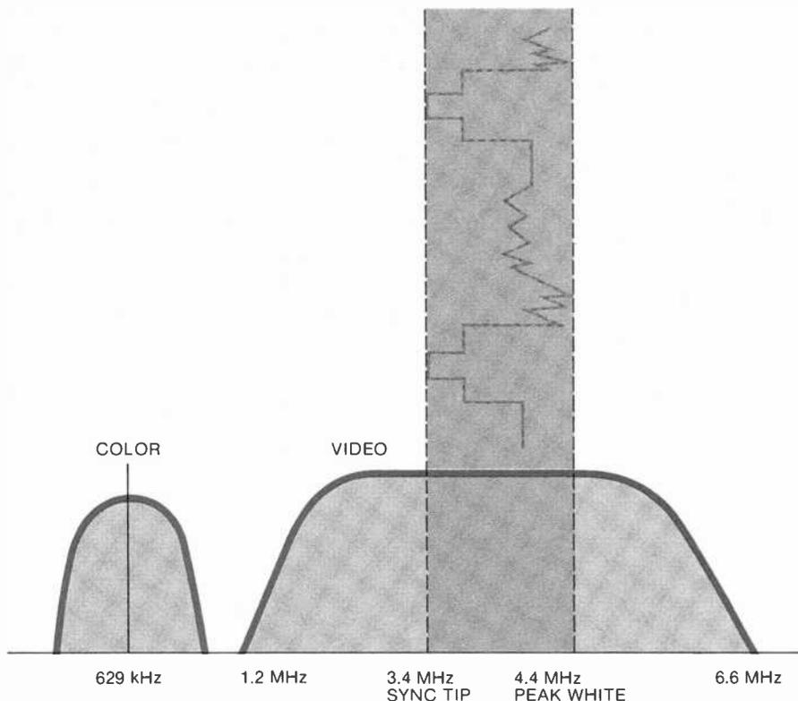
Fig. 1. Video signal spectrum of typical VCR. Luminance signal is recorded as constant-amplitude AM.
