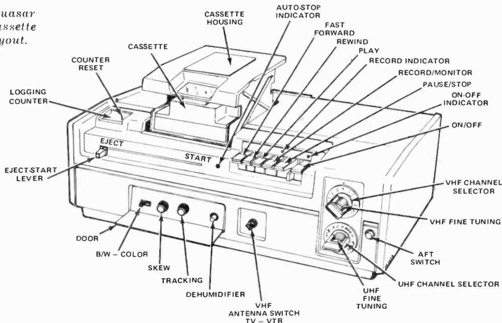
these times at slow speed. The single-speed Model VR-1000's cartridge offers either 60- or 120-minute lengths.
