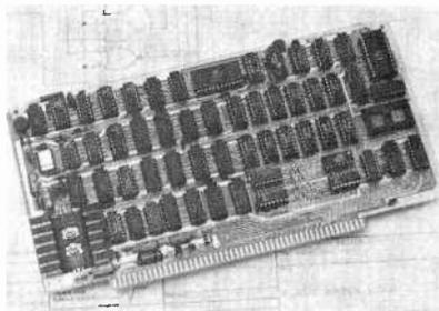
ics. It has its own screen-refresh memory and latched eight-bit parallel port, is S-100 compatible, and video output is available as composite video or separate video and sync. \$195 kit, \$235 assembled.
