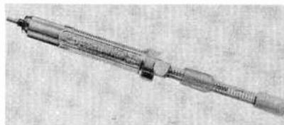
sensitive FET and MOSFET semiconductor devices from damage due to static electricity discharge. The device has a fully enclosed loading shaft, high-low vacuum adjustment, and bayonet-type disassembly.
