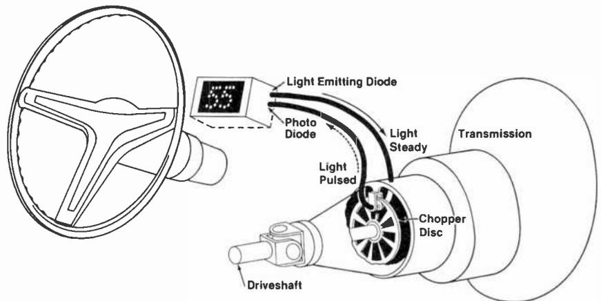
ple, has developed a photo-cybernetic system to monitor vehicle speed, eliminating less reliable mechanical linkages. Readout is by digital LED's. And just imagine what the potential clock rate of a computer would be with no impedance in inter-connecting circuitry! Clearly, it's a technology whose time has come.
