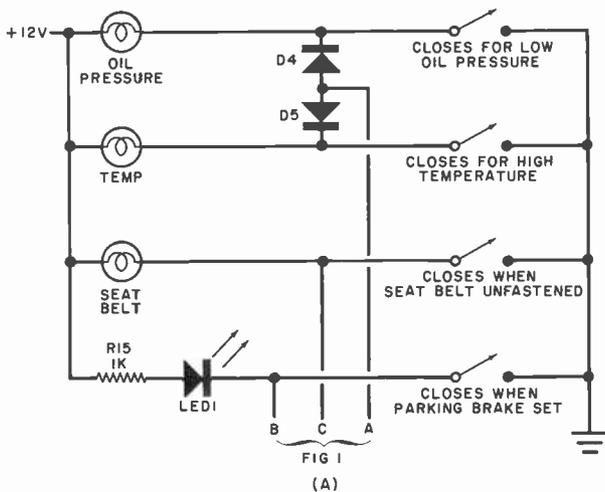
Fig. 2 Function sensing is shown at (A) while (B) shows how dc power is applied to the alarm circuit.
