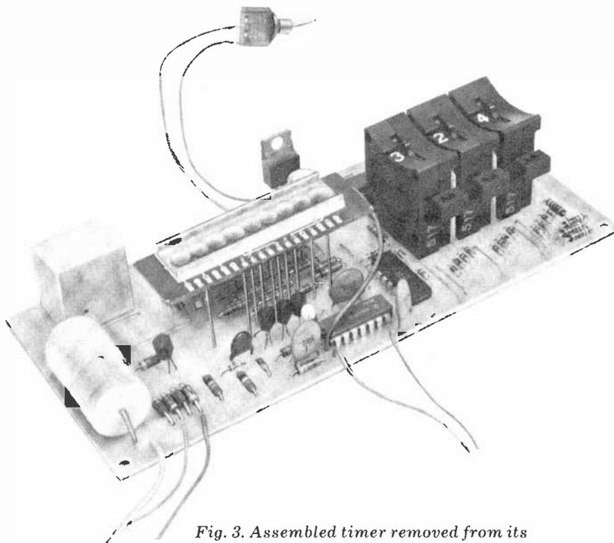
Fig. 3. Assembled timer removed from its enclosure shows how the display board mounts above main board. Cube at left rear is relay.
