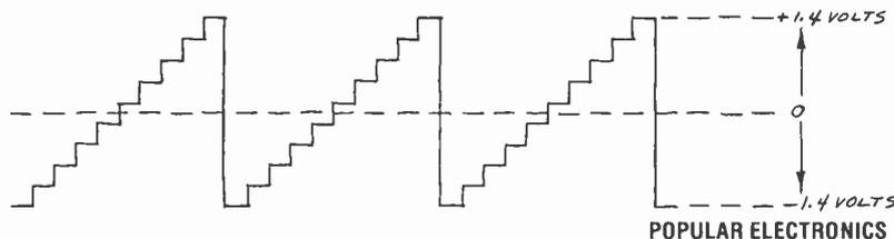
Fig. 3. Ramp voltage output from D/A converter in Fig. 2.
