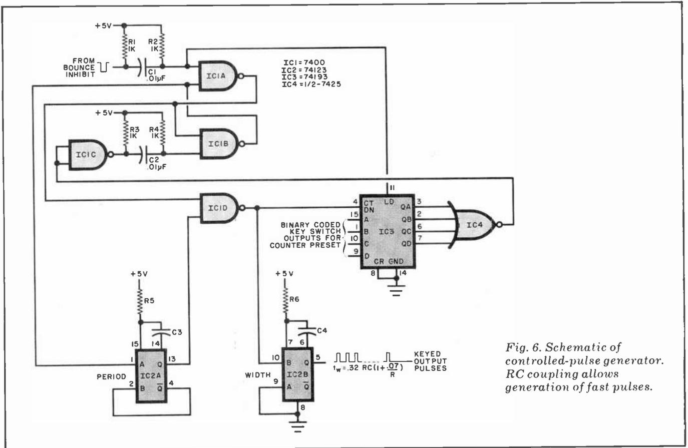
Fig. 6. Schematic of controlled-pulse generator. RC coupling allows generation of fast pulses.
