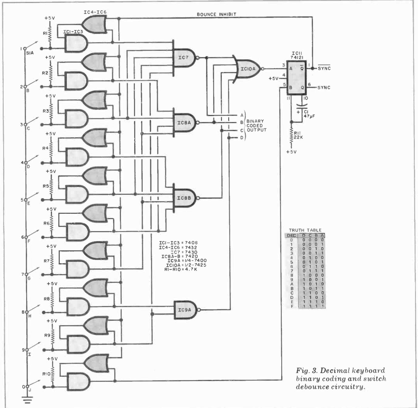
Fig. 3. Decimal keyboard binary coding and switch debounce circuitry.
