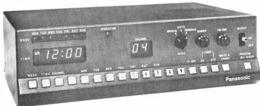
Programmers are available (Panasonic shown) that can be set to automatically select channels and times for a week's recordings.
