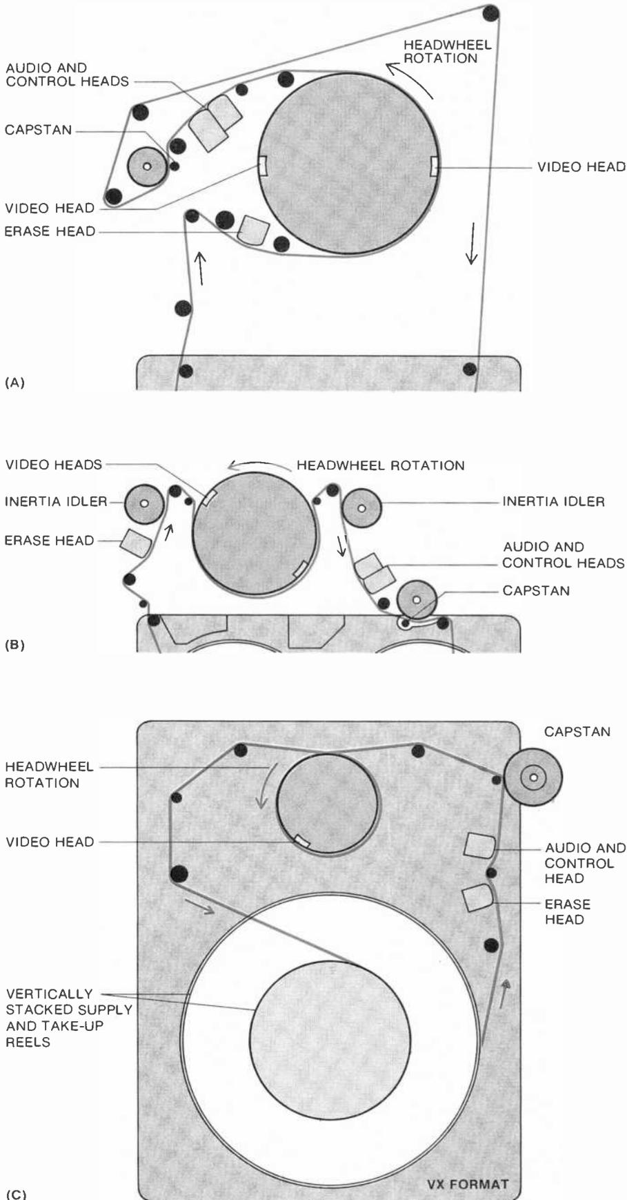
Fig. 7. Various ways of video-tape passage through VCR machine: (A) Betamax's modified "U-load;" (B) simpler "M-load" used by VHS; (C) "Alpha-wrap" on Quasar's VR-1000.
