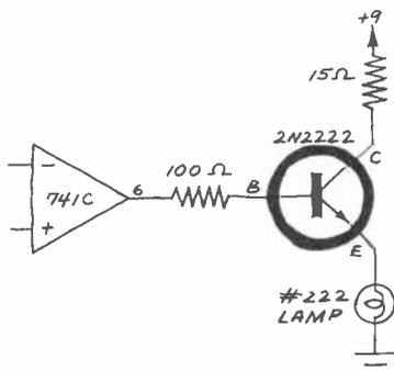
Fig. 5. Driver added to converter.
