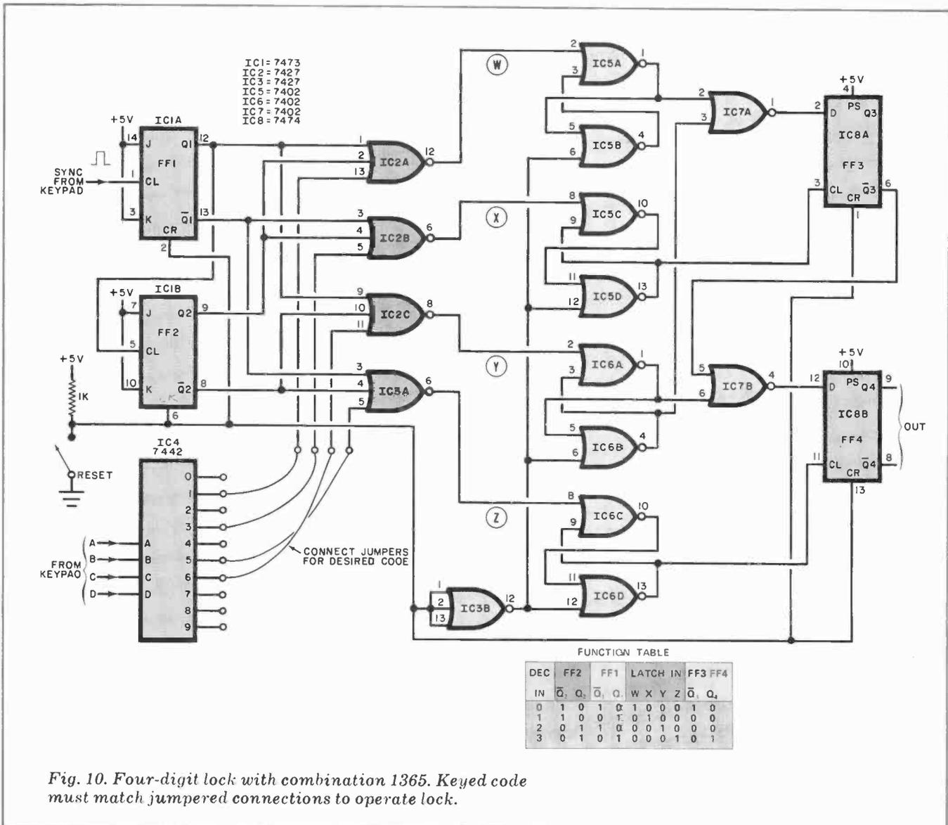
Fig. 10. Four-digit lock with combination 1365. Keyed code must match jumpered connections to operate lock.
