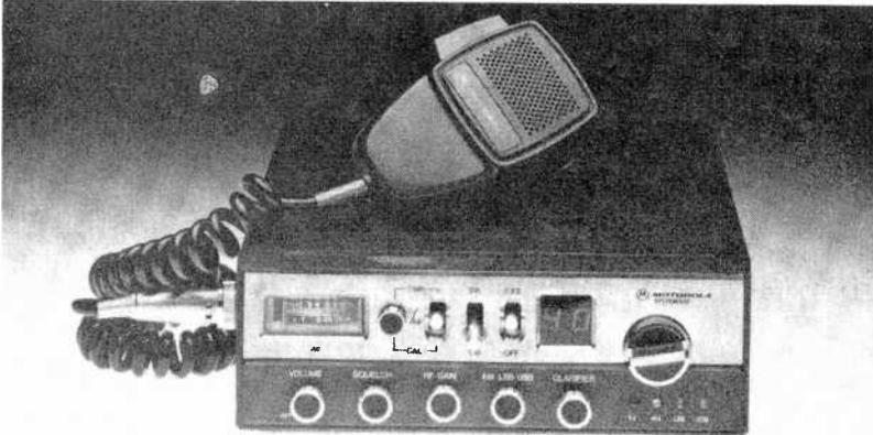
**T**HE Motorola Model CM550 is a mobile AM/SSB 40-channel transceiver for Citizens Band communications. Full-band operation is accomplished with the aid of the usual phase-locked-loop (PLL) frequency synthesis system.
