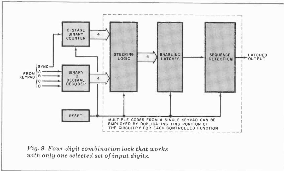
Fig. 9. Four-digit combination lock that works with only one selected set of input digits.
