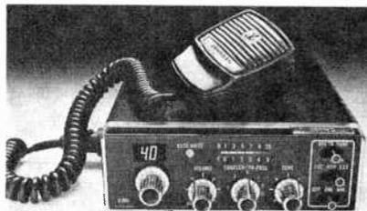
through the use of twin ceramic selectivity filters, switchable noise-blanker/ANL system. Controls include three-position range switch, delta tune switch, tone, CB/PA switch, and calibrated squelch. The Viking 260's cabinet is covered with leather-textured black vinyl (other colors available). \$199.95.
