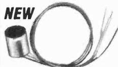
Condenser mike element for new or replacement use. Built-in FET preamp. 30-15,000 Hz audio response. Requires 2 to 10VDC. 270-092 ..... 2.49
