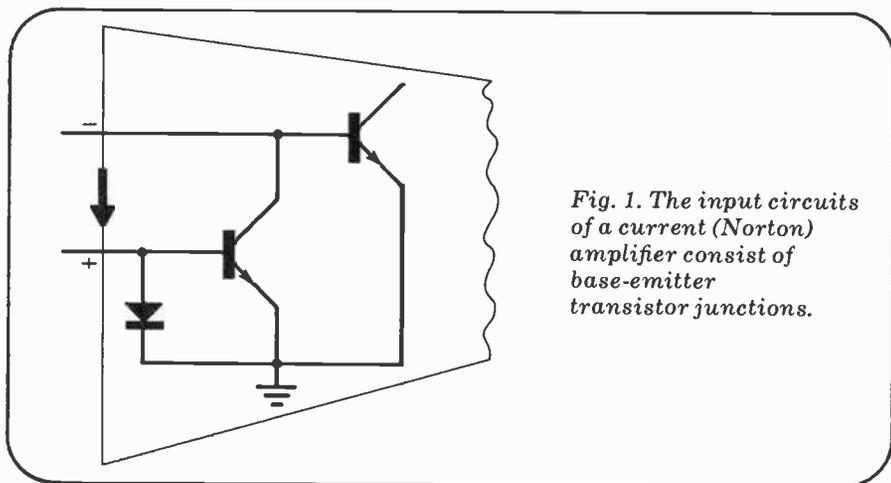
Fig. 1. The input circuits of a current (Norton) amplifier consist of base-emitter transistor junctions.
