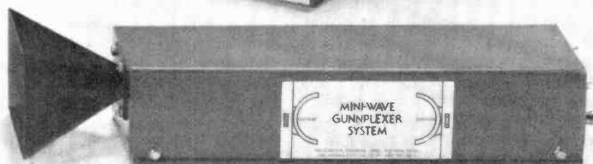
the cavity to heterodyne, resulting in sum and difference mixer products. A Schottky diode is employed. (Noise generated in the receiver can reduce range dramatically, so care must be taken to minimize it. One way to do this is to use low-noise components such as the Schottky diode.)
