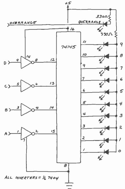
Fig. 4. Ten-position moving-dot readout circuit.
