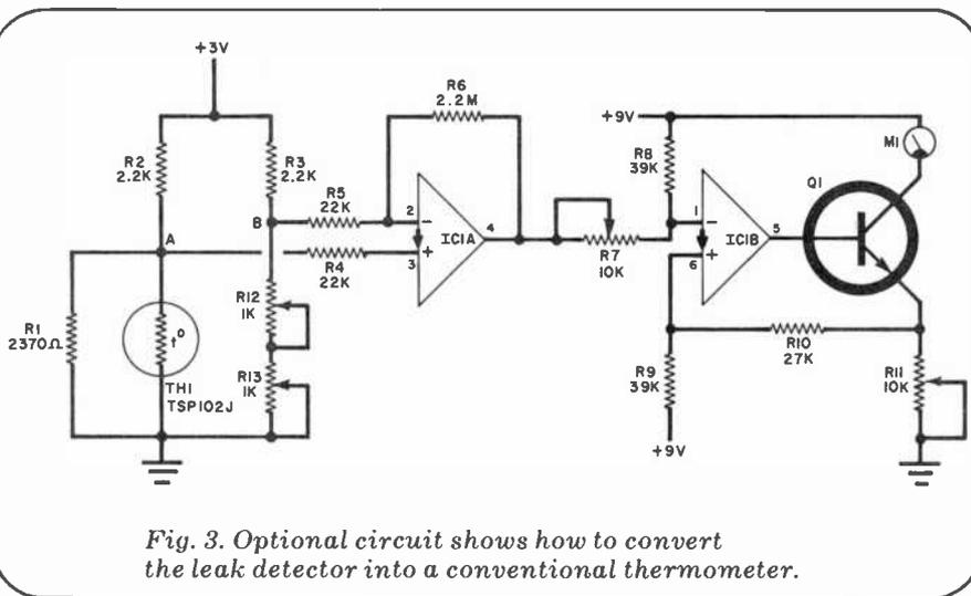
Fig. 3. Optional circuit shows how to convert the leak detector into a conventional thermometer.
