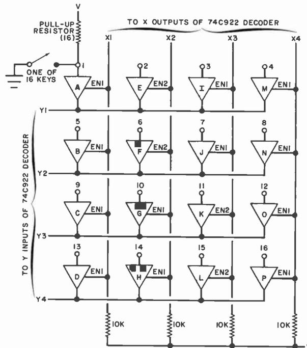
Buffers A through F are on one IC (DM8097, DM7097, or SN74367); G-L on second; and M-P on third.
