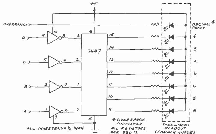
Fig. 3. Adding a digital readout to the A/D converter.
