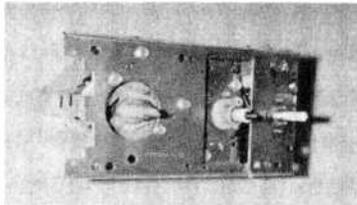
This is a wired and tested combination VHF/UHF tuner sub unit that has its own AC power supply and works equally well on color or b/w...tube or transistor sets...The VHF tunes channels 2 thru 13...The UHF is a detent (the kind that clicks for each channel) and tunes 14 thru 83.
