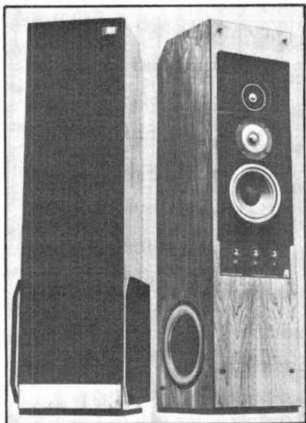
The Model AR-9 is a tall, column-shaped four-way speaker system with five drivers. It's rated to handle up to 400 watts of continuous power, with each channel driven to clipping 10% of the time on normal music material. Since
