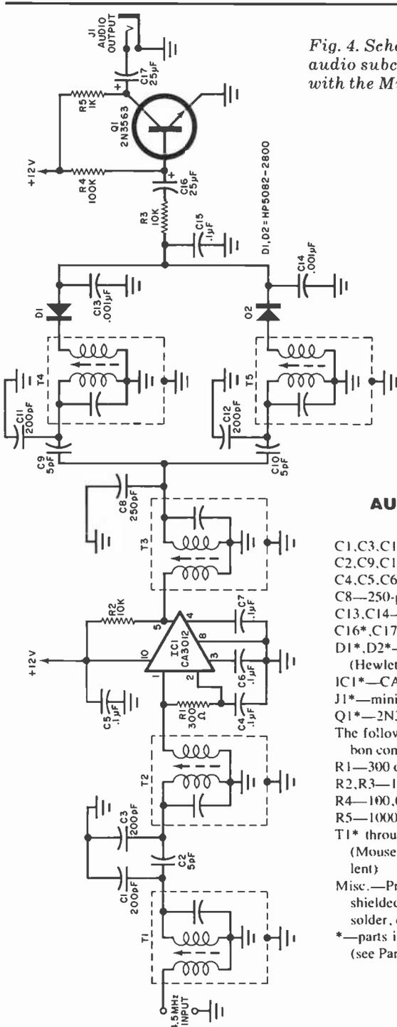
Fig. 4. Schematic of the optional audio subcarrier demodulator for use with the Mini-Wave video receiver.
