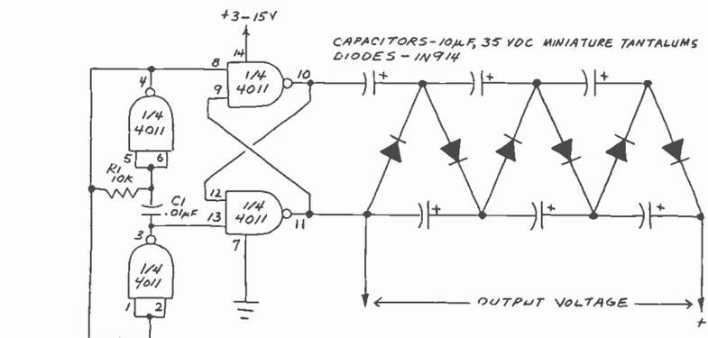
Fig. B. Miniature dc-dc upconverter circuit.
