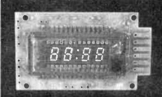
Needs only 12V DC and 3 time-setting switches for operation in boat, truck, van, car, or home. 4 digit, 0.3" green fluorescent display with blinking colon. When wired in car, display turns off when ignition is off. Accurate to ± 1/2 second a day thanks to built-in crystal timebase.
