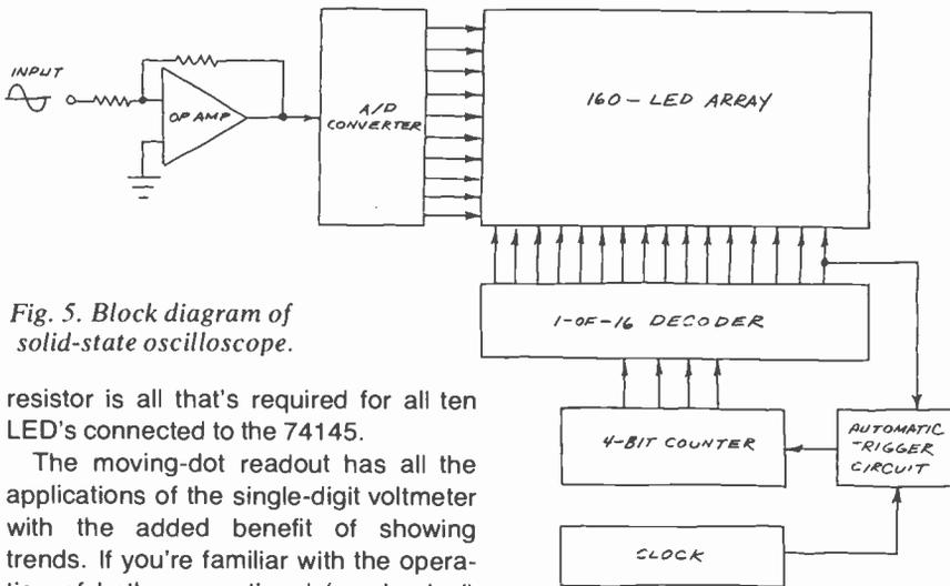
Fig. 5. Block diagram of solid-state oscilloscope.
