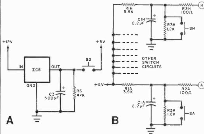
Fig. 7. Five-volt supply (A) and key
