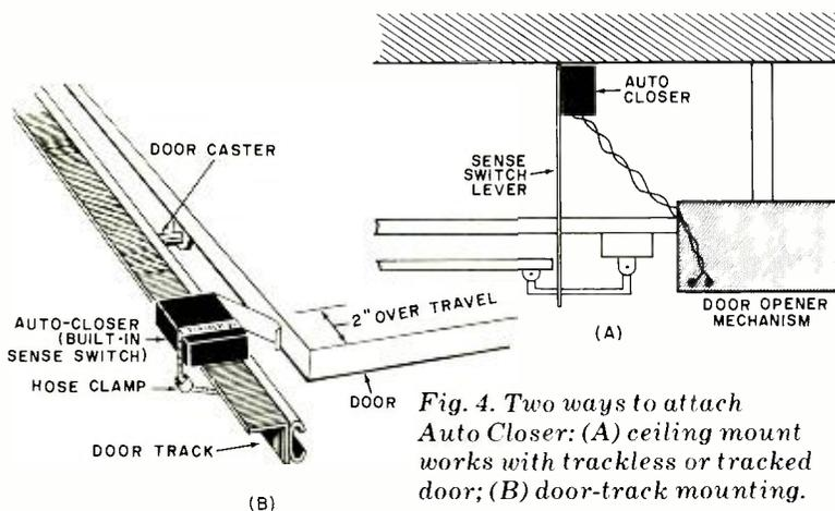
Fig. 4. Two ways to attach Auto Closer: (A) ceiling mount works with trackless or tracked door; (B) door-track mounting.
