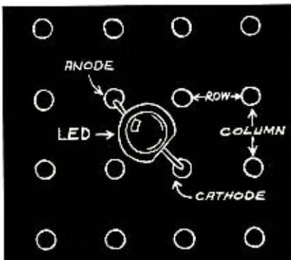
Fig. C. Orientation of individual LED in array.
