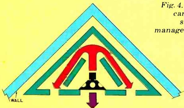
Fig. 4. Large bass horn can be folded into a structure of more manageable dimensions. Walls of room act as extensions of the horn.
