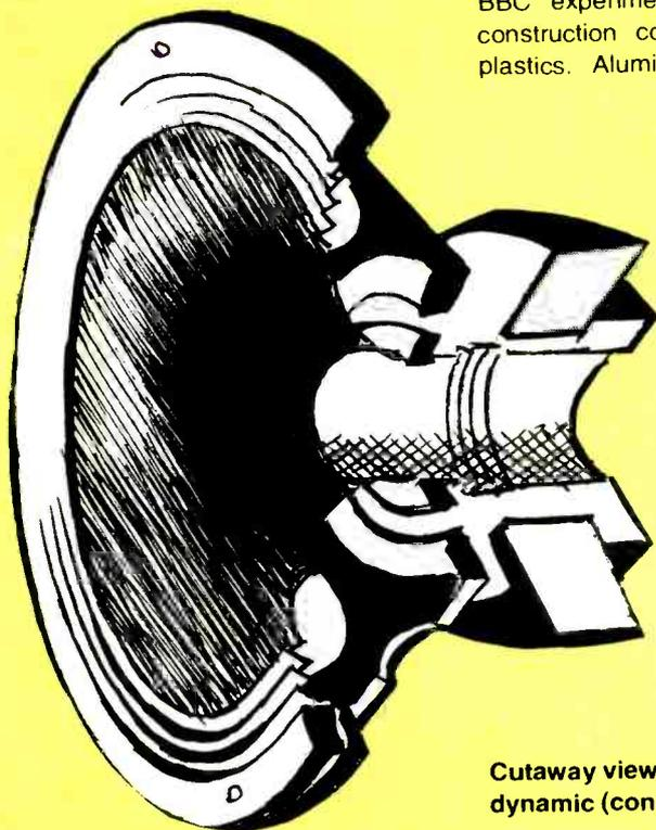
Cutaway view of dynamic (cone) driver.
