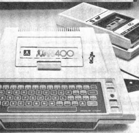
The Atari-400 personal computer uses a 6502 CPU, 8K of RM and 8K of ROM. Keyboard is a 56-key Monopanel with touch-control points.
