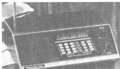
Service Band (five vhf-uhf) and AM Aircraft Band reception in a single unit. The crystal-less ac/dc receiver employs pushbut-
