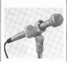
clamp from Electro-Voice was designed to hold a mike with an approximate ¾" barrel diameter. A hinged metal latch is provided to hold the microphone in four replaceable urethane bands for temporary shock mounting. When used with a set screw, the 313A becomes a semipermanent shock mount for applications that don't require frequent mike changes. \$23.
