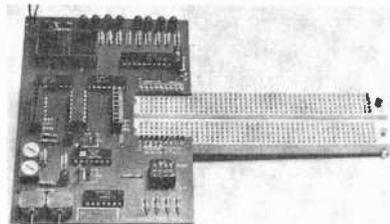
Instruments. Powered by a 6-volt battery, it contains two bounceless pushbuttons, two readouts with BCD inputs, four switch outputs, eight LED monitors, two variable clock generators, and two decade counters. \$35, kit; \$45, assembled.
