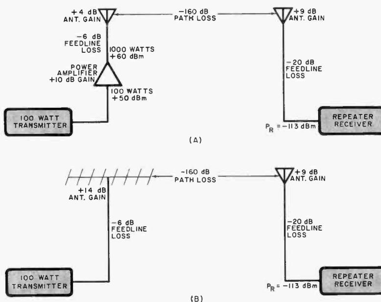
Fig. 6. To achieve full quieting, the transmitted power can be increased (A) or a different type of antenna can be used (B).
