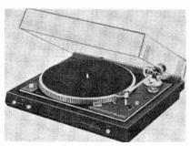
then higher.) The platter is directly coupled to the motor, whose speed is controlled by a quartz oscillator system that allows up to 11% variation in pitch on command. The turntable also incorporates a front-panel, solenoid-operated cue control, four-point gimbal tonearm suspension, lead-in groove sensing, and a spring-operated stylus force mechanism. It is supplied with base and dust cover, but without cartridge. \$480.
