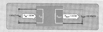
Fig. 3. Simple network illustrates voltage and power relationships.
