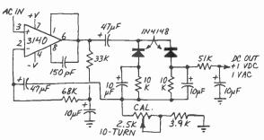
The 47- $\mu$ F capacitors are not critical, but they should be fairly large and equal in value. The 1- $\mu$ F capacitor on the output can be considerably reduced in value, especially at higher frequencies. This will help the output to settle faster. The CAL potentiometer should be a 10-turn brecision device.
