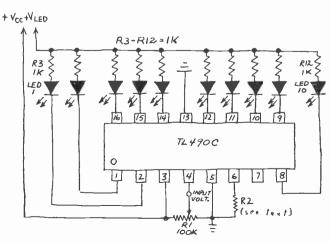
Fig. 3. Basic 10-element bargraph readout using TL490C.
