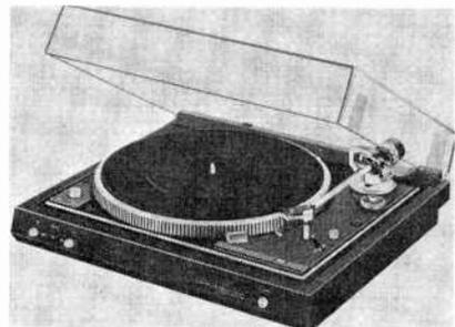
then higher.) The platter is directly coupled to the motor, whose speed is controlled by a quartz oscillator system that allows up to 11% variation in pitch on command. The turntable also incorporates a front-panel, solenoid-operated cue control, four-point gimbal tonearm suspension, lead-in groove sensing, and a spring-operated stylus force mechanism. It is supplied with base and dust cover, but without cartridge. \$480.
