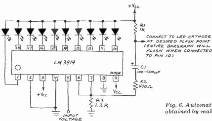
Fig. 6. Automatic bargraph flashing can be obtained by making connection suggested.
