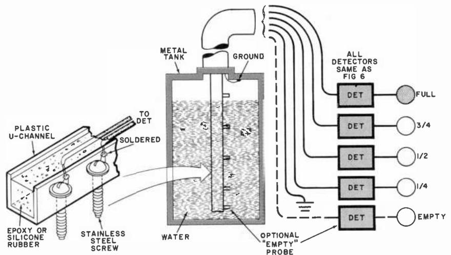
Fig. 5. Fresh water tank guage that displays liquid level on a set of LED readouts.
