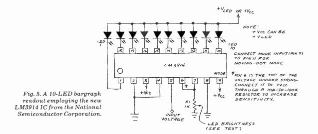
The current passing from pin 7 through *R1* to ground is approximately one-tenth of the current passing through each illuminated LED. Since the voltage reference output is typically 1.3 volts, the LEDs will receive 13 mA of current when the resistance of *R1* is 1000 ohms. (Why? Ohm's law says that the current flowing through a resistor equals the voltage across it divided by its resistance. In this case, the current is 1.3/1000 or 0.0013 A. The LED current is ten times greater or 13 mA.)
