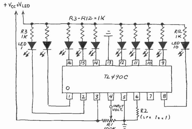
Fig. 3. Basic 10-element bargraph readout using TL490C.
