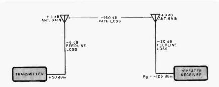
Fig. 5. Diagram showing the various gains and losses encountered in a communications system.
