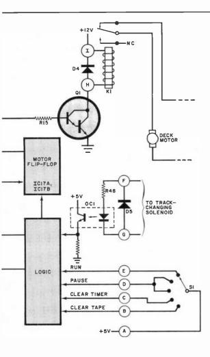
Fig. 1. Five major functional sections of the 8TT are shown in block diagram. The motor flip-flop is actually two cross-coupled NOR gates.
