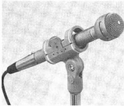
clamp from Electro-Voice was designed to hold a mike with an approximate  $\frac{3}{4}$ " barrel diameter. A hinged metal latch is provided to hold the microphone in four replaceable urethane bands for temporary shock mounting. When used with a set screw, the 313A becomes a semipermanent shock mount for applications that don't require frequent mike changes. \$23.
