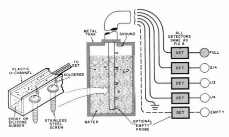
Fig. 5. Fresh water tank guage that displays liquid level on a set of LED readouts.
