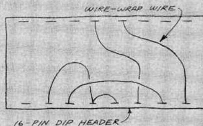
Fig. 2. Connections for LED pulser.
