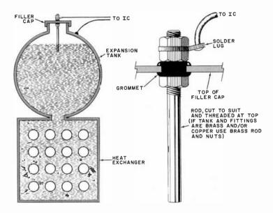
Fig. 4. Low-level warning device for closed system.
