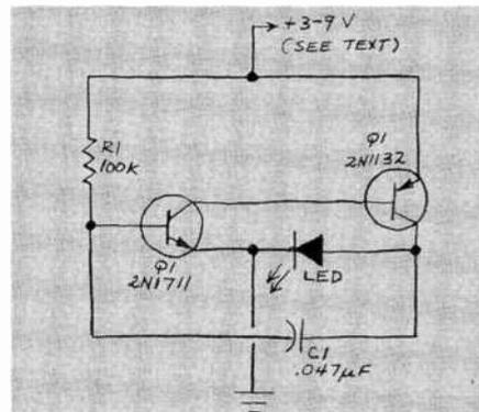
Fig. 1. High-current LED pulser.
