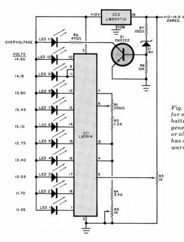
Fig. 1. Circuit for monitoring battery, generator or alternator has overvoltage warning feature.
