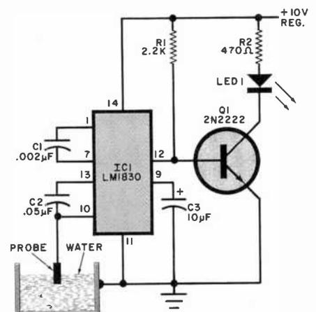
Fig. 6. High-water detector for grounded metal tank.
