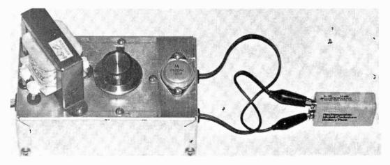
Photo of author's prototype shows components mounted on top of enclosure with clip leads used to connect battery to charger.
