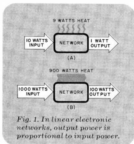
the attenuator,  $P_O$ , is related to the input power  $P_I$  by the equation  $P_O = (K) (P_I)$  with  $K = 1/10$ ; where  $K$  is a ratio called the gain factor. Of course, it is possible to cascade two or more such networks to obtain a cumulative effect, as shown in Fig. 2. Here two attenuating networks are used. Their total effect is identical to that produced by a single attenuator with a gain factor of  $1/100$ :  $P_O = (1/10) (1/10) (P_I) = (1/100) (P_I)$ .
