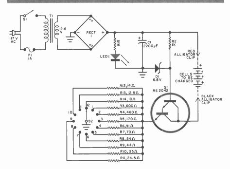
Fig. 1. Schematic shows how zener D1, Darlington Q1, and resistors R3 through R14 form constant-current source which regulates battery charging.
