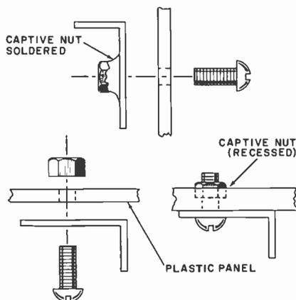
machine nuts can be soldered to steel chassis and the foil pattern on printed circuit boards or they can be imbedded into acrylic plastic panels to be held captive. You start by drilling a hole just large enough to pass the threads of a machine screw, insert the screw, and screw on the nut until it is comfortably tight.
