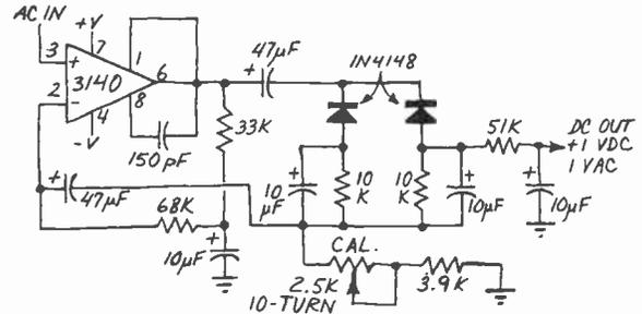
The 47-µF capacitors are not critical, but they should be fairly large and equal in value. The 1-µF capacitor on the output can be considerably reduced in value, especially at higher frequencies. This will help the output to settle faster. The CAL potentiometer should be a 10-turn precision device.
