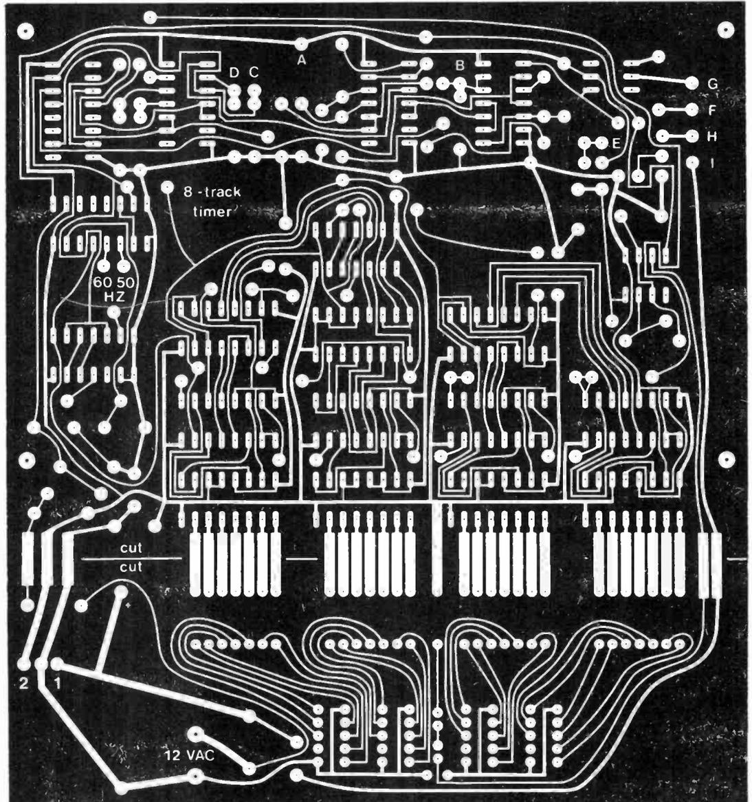
Fig. 3. Actual-size foil pattern for the 8TT's single pc board.
