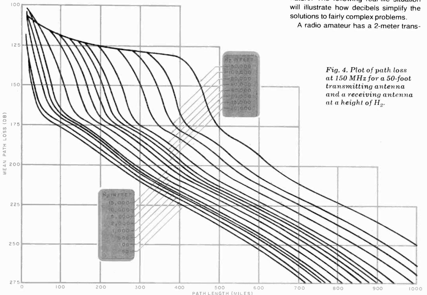
Fig. 4. Plot of path loss at 150 MHz for a 50-foot transmitting antenna and a receiving antenna at a height of  $H_2$ .
