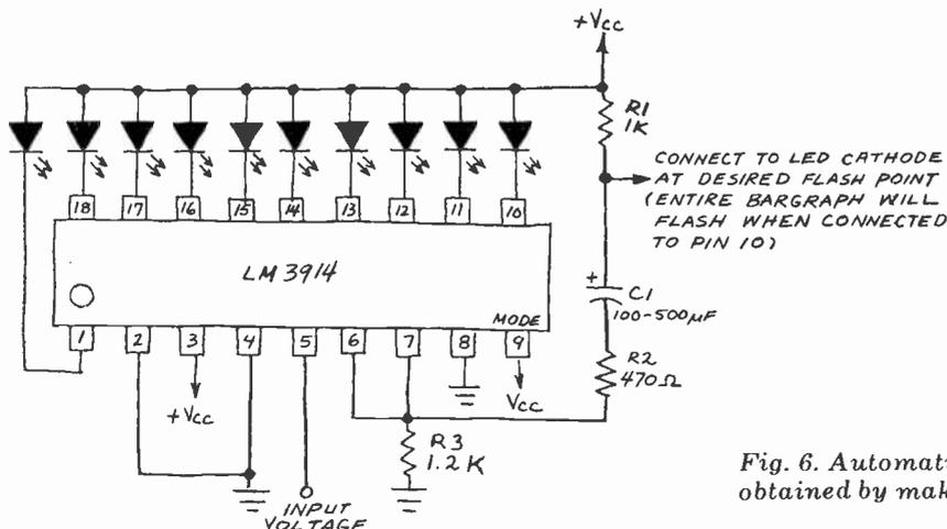
Fig. 6. Automatic bargraph flashing can be obtained by making connection suggested.
