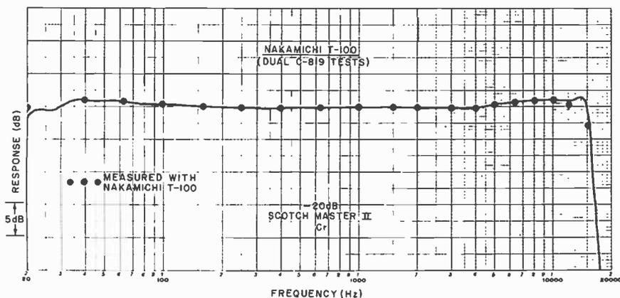
Chart shows use of the T-100 in making record/playback response tests of a Dual tape deck. Continuous line was made with General Radio plotter.
