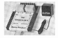
logic signals. Two inputs are opto-isolated. Inputs and outputs of the Interfacer 2, which plug directly into the 40-pin edge connector on the rear of the TRS-80 interface, are controlled by level II Basic INP and OUT statements. \$88. Address: Alpha Product Co., 85071 79th St., Woodhaven, NY 11421.
