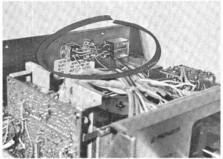
cable connected to both units. As long as the 8TT's power switch is in its OFF position, the deck will behave as if the 8TT were not connected to it. Also, because the interface between the deck and timer consists of a relay and optoelectronic coupler, there is no possibility that hum will be introduced into the deck by the 8TT.
