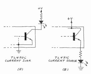
Fig. 2. LEDs connected to current sink (A) and current source (B).
