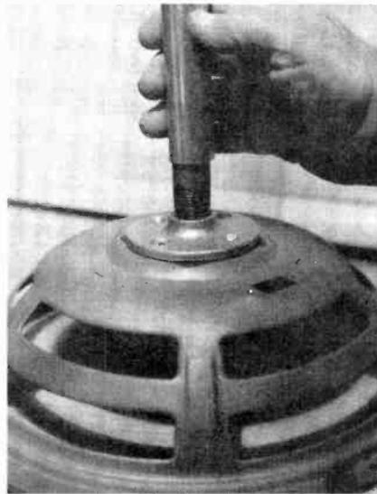
latter for use in your shop to mount tools on a wall, keep machine hardware in one place, etc. Now, substitute a 1/2" (12.7-mm) diameter pipe fitting for the magnet, using a threaded flange, as shown in the photo. Fasten the speaker basket to the roof with pan-head sheet-metal screws. Assemble the antenna, fasten it to the mast, and slip the mast over the pipe fitting. Aim the antenna in the desired direction and clamp and guy the mast.—Glen Stillwell, Manhattan Beach, CA.
