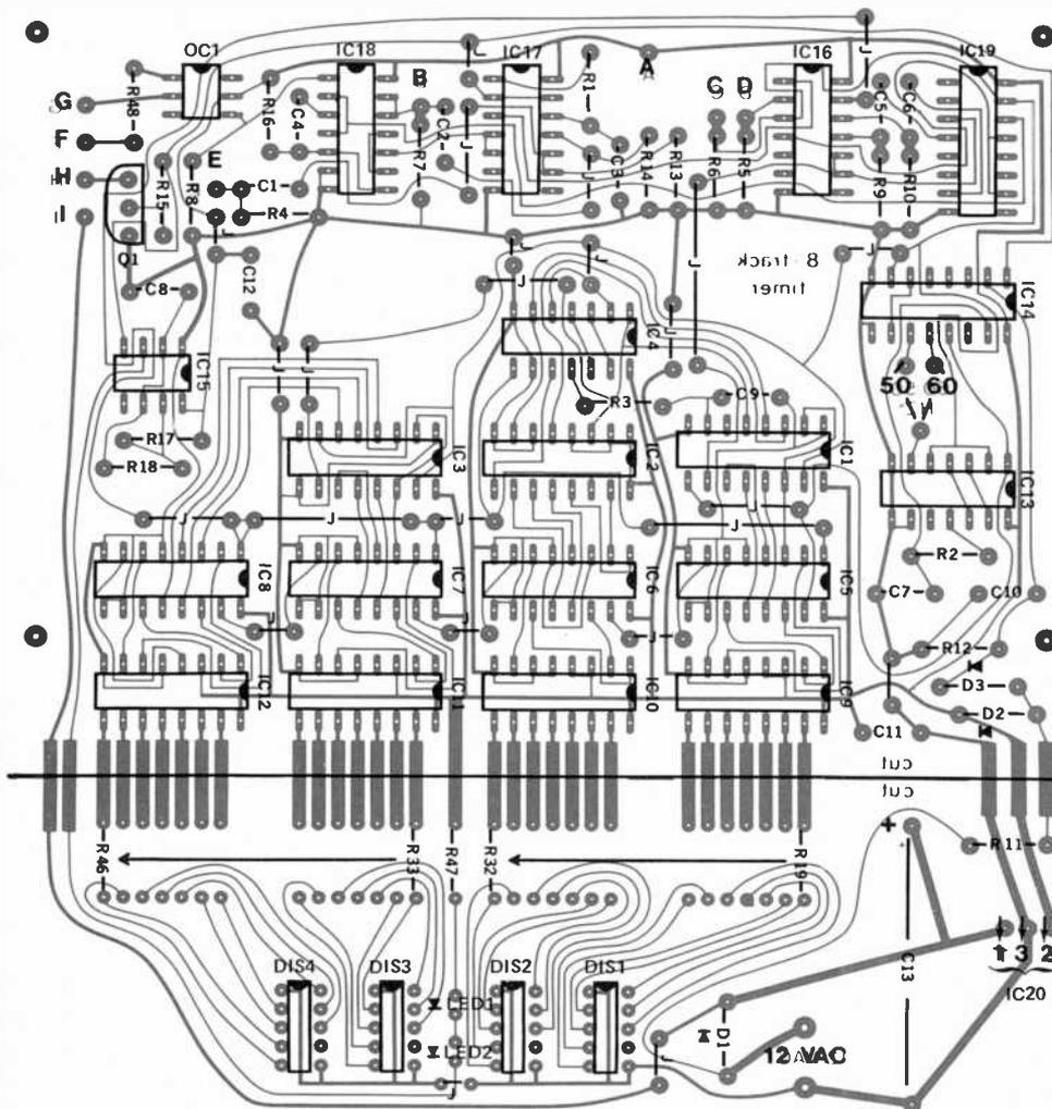
Fig. 4. Component placement guide for the 8-Track Timer.
