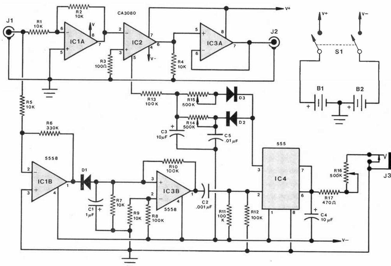
Fig. 1. Transconductance amplifier  $IC2$  has its input and output buffered by  $IC1A$  and  $IC3A$  respectively. Gain of  $IC2$  is varied by circuit containing  $IC4$ , which is triggered by  $IC3B$  and  $IC1B$ .
