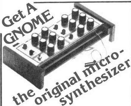
John Simonton's time-proven design provides two envelope generators VCA, VCO & VCF in a low cost, easy to use package.
