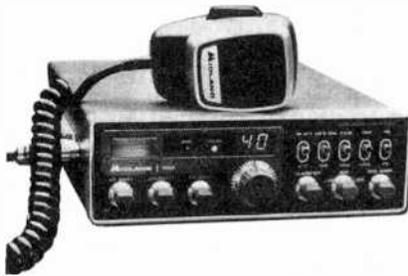
0.7  $\mu$ V for 10 dB (S + N)/N sensitivity; 60-dB adjacent-channel selectivity and desensitization; 3 watts at 10% distortion audio output power into 8 ohms; 4 watts maximum, 3.6 watts minimum carrier power with no modulation; -65-dB spurious emissions; -40-dB transmitter, -45-dB receiver hum and noise. \$319.95.
