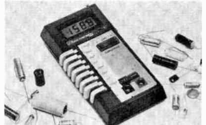
ing for stray capacitance of test leads. Measurements appear on a 0.5" (12.7-mm) high liquid crystal display. An internal fuse prevents instrument damage from charged capacitors and should the test leads be inadvertently connected across a voltage source. Uses a single 9-volt alkaline battery. \$149.00
