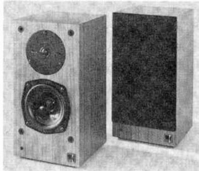
drivers—a 25-mm (1") tweeter and a 110-mm (4¼") woofer—and the crossover network as well. The speaker is rated to accept the output of an amplifier up to 100 watts and has an automatic protection system to prevent overdriving. Maximum output level is said to be 98 dB SPL. Sold in matched pairs with teak or walnut finish and a brown fabric grille.
