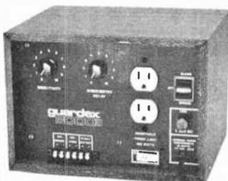
*The rear control panel contains two standard AC plug receptacles for a table lamp, spot lights, radio, etc.; terminals for connecting optional outside siren and back-up battery (not included); entry delay time control and sensitivity control.*
