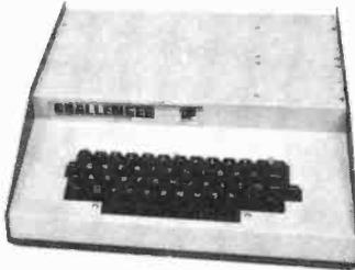
**The Challenger 1P.** The best bargain in personal computer anywhere! 8K BASIC-in-ROM. 4K RAM. Cassette based with 53-key keyboard. B&W video display, 30 rows x 30 columns. Upper and lower case. **\$349.** C1P with 8K RAM **\$399.**
