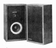
be able to produce 107 dB SPL at 1 meter. The tweeter is designed to withstand repeated 1-kW pulses and, with the rest of the system, carries a lifetime warranty to the original owner. The manufacturer states that the enclosure, constructed of walnut-veneered 3/4" particleboard, is optimized to work with the woofer. \$116.
