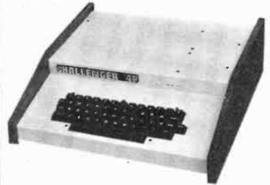
**The Challenger 4P.** A 4-slot computer with one open slot. Highly sophisticated 16 color video display. 32 rows x 64 columns, upper and lower case. 8K BASIC-in-ROM 8K RAM. 200-20KHz programmable tone generator. AC remote interface. Expandable to 32K RAM and two mini-floppy drives. **\$698.**
