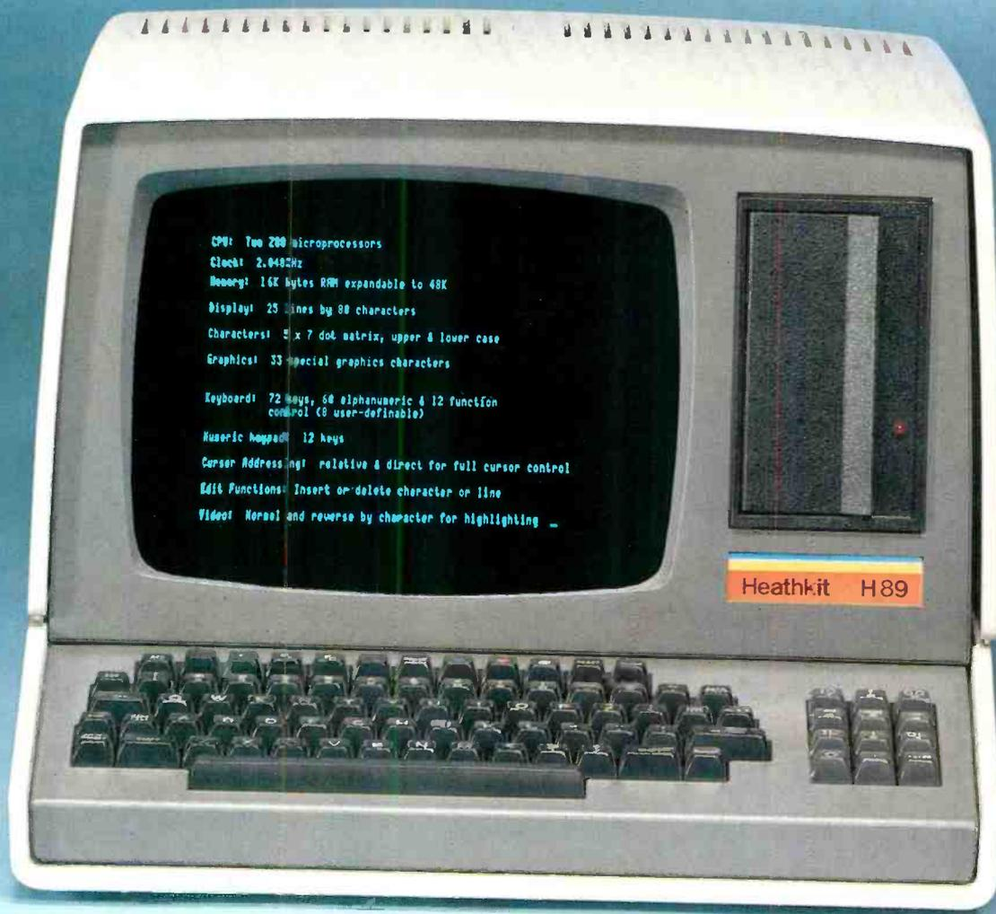
CPU: Two Z80 microprocessors
