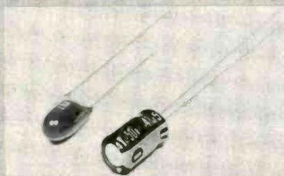
**ULTRAMINIATURE ALUMINUM ELECTROLYTICS**, comparable in size to tantalum capacitors of the same capacity, have been developed by Panasonic. The K series capacitors come in 17 values ranging from 0.1 to 100  $\mu$ F and have dc ratings from 6.3 to 63 volts. Maximum length is only 7 mm (0.28"), while diameters are 4, 5, and 6.3 mm (0.157", 0.177", and 0.248"). Currently available with radial leads only, the new capacitors are priced to start at less than 10¢ in production lots.
