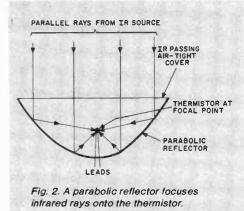
at the "focal point" previously recorded. Use a dab of epoxy at each lead to secure the two leads to the board. Make sure bare leads do not make contact with the metal reflector.
