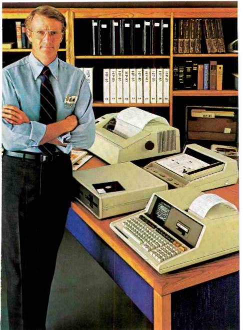
The Personal Computer For Professionals: HP-85 specifications: Memory-16K RAM expands to 32K, 32K ROM expands to 80K; CRT-32 chars./line, 16 lines; graphics-256 X 192 dots; thermal printer-2 lines/sec.; magnetic cartridge capacity -200K; 1/O-HP-IB (IEEE 488), RS-232, 16-bit GP-IO, BCD; Application Pacs include Statistics & Regression Analysis, Finance, Math, Linear Programming, Text Editing, Waveform Analysis, Circuit Analysis, BASIC Training, & Games.
