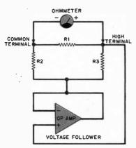
Fig. 3. Here, the voltage follower prevents shunting components from influencing theohmmeter reading.
