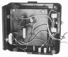
Since the temperature of the sensor is now approximately  $37^{\circ}$ F (the usual temperature that a refrigerator is set to), adjust R7 until the LED just turns on. The system is now set up to sound off when the sensor "sees" a temperature below  $37^{\circ}$ F.
