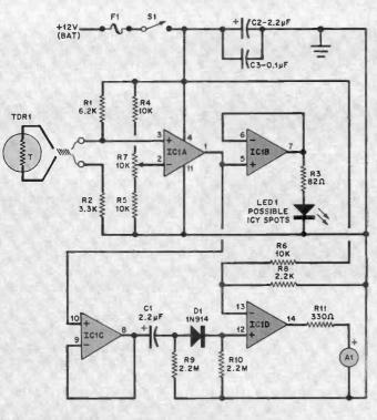
Fig. 4. The thermistor is part of a bridge that drives comparator IC1A. When this comparator tums on (detected temperature below preset), it activates a LED and an audible alarm.
