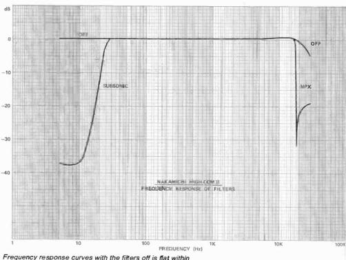
Frequency response curves with the filters off is flat within  $\pm$  0.6 dB from 5 to 20,000 Hz. The subsonic filter cuts off below 30 Hz, and the MPX filter notches at 19 kHz.
