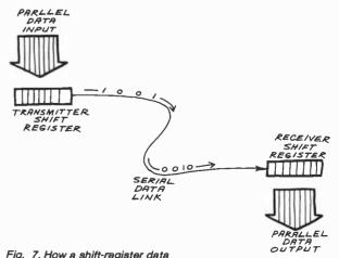
Fig. 7. How a shift-register data transmission system operates. parallel so that up to four 4-bit data words or nibbles (half of an 8-bit byte) can be stored. The clock (shift) lines of all four registers are tied together so that a 4-bit nibble can be loaded into the stack in one operation. The nibble can then be pushed down into the stack as more are loaded.
