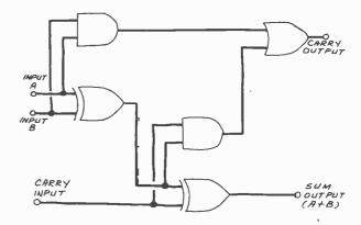
Fig. 5. Logic diagram of a binary full adder.
