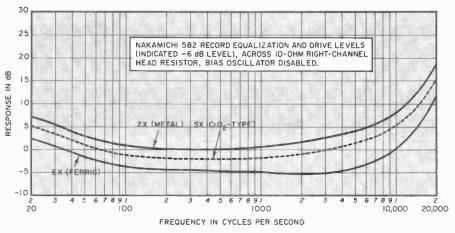
Fig. 2. Record equalization curves for Nakamichi 582 with three different tapes.
