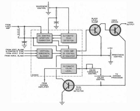
Fig. 4. Diagram showing operation of the IC900, the video clamp/processor and color amplitude noise limiter.
