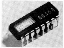
Fig. 6. Epson's programmable clock-pulse generator contains a quartz crystal oscillator.
