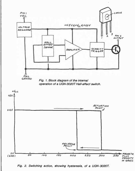
the Schmitt trigger turns off only when the intensity of the magnetic field falls well below the level required initially to turn the Schmitt trigger on. Figure 2 summarizes the circuit's operation.
