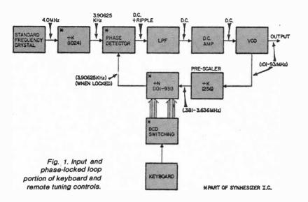
tems without channel scan have 10 keyboard command buttons for selecting any vhf or uhf channel. (Single-digit channel numbers must be keyed in preceded by zero, such as 02,03,04, etc.) Receivers with up/ down channel scan have 12 buttons. Neither type of channel-selection system has receiver or remote programming for channel scan; stations must be sequenced in strict up or down numerical order.
