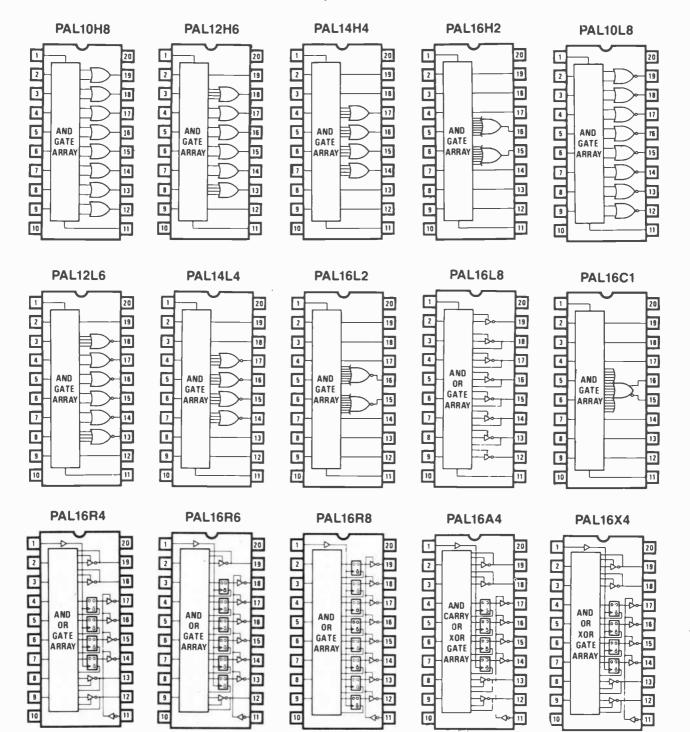
Fig. 4. Pin outlines and internal block diagrams of the PAL family of chips.
