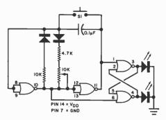
(Note that IC pin numbers in the diagram apply for both the 4001 and 4011.) With this circuit, it is necessary to adjust for a 50% clock duty cycle, using the potentiometer. If you don't have an oscilloscope to do this, simply measure the direct current flowing through each LED while adjusting the pot. When the same current level flows through each LED, the clock will be adjusted for a 50% duty cycle. —Ed Johnston, Oshawa, Ontario, Canada.
