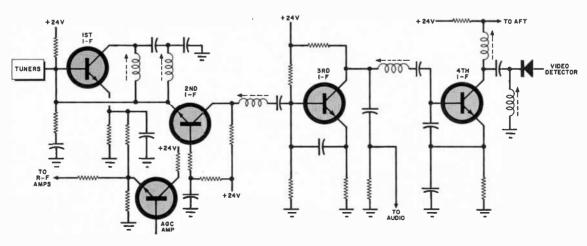
Fig. 2. Partial schematic of the automatic gain control circuit and four-stage video i-f strip.
