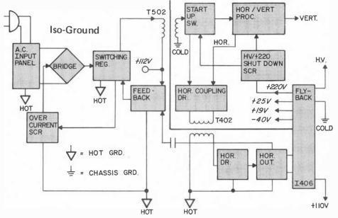
Fig. 3. Block diagram of the power supply system showing how two ground points (hot and chassis) are used.
