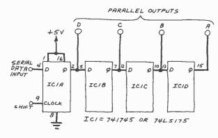
Fig. 3. A four-bit shift register made from a single quad D flip-flop.
