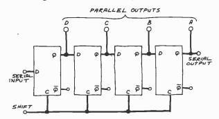
Fig. 1. Basic block diagram of a D flip-flop shift register.
