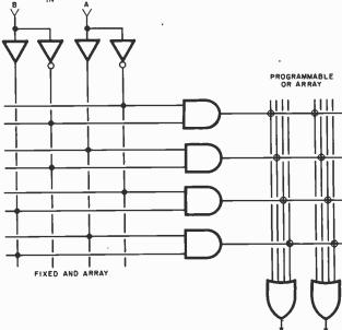
Fig. 1. A PROM of four two-bit words The AND array is fixed; the OR is programmable.
