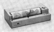
Strobe's Model 100 combined alphanumerics and graphics plotter is a drum-type system that uses 4-phase stepping motors to achieve 0.004-inch (0.1 mm) motions on each axis. It accepts any 8'/2'' by 11'' paper and a variety of conventional pens. An interactive digitizing mode enters pen data
