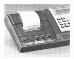
manual. A paper-advance button and papercutter edge are also provided. It uses the computer's PRINT and LIST commands to print a 16-column alphanumeric array. The printer operates at one line per second, and about 8000 lines per battery charge. An indicator alerts to low battery. Several options are available. \$149.95. Address: Radio Shack stores and Computer Centers.
