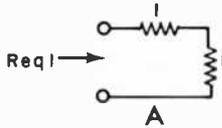
sistance of the basic circuit, is 2 ohms. This equivalent resistance can replace two resistors in the problem. (It might be helpful to think of  $Req_1$  as replacing the two resistors that are located at infinity.) We can thus reduce a 4-resistor network to just 3 resistors. The resistance of the 4-resistor network can then be found and substituted into a 6-resistor network, reducing the number of resistors in this network from 6 to 3. At B, we see how an
