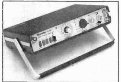
The TG102 is the newest product in the Thandar line of test instruments. Ac operated, it has a frequency range from 0.2 Hz to 2 MHz. It produces sine, square, and triangle waveforms plus dc from a variable-amplitude 50-ohm output. TTL output is also provided. External sweep facility is available, too, permitting a greater than 1000:1 frequency change within a selected range. \$300.
