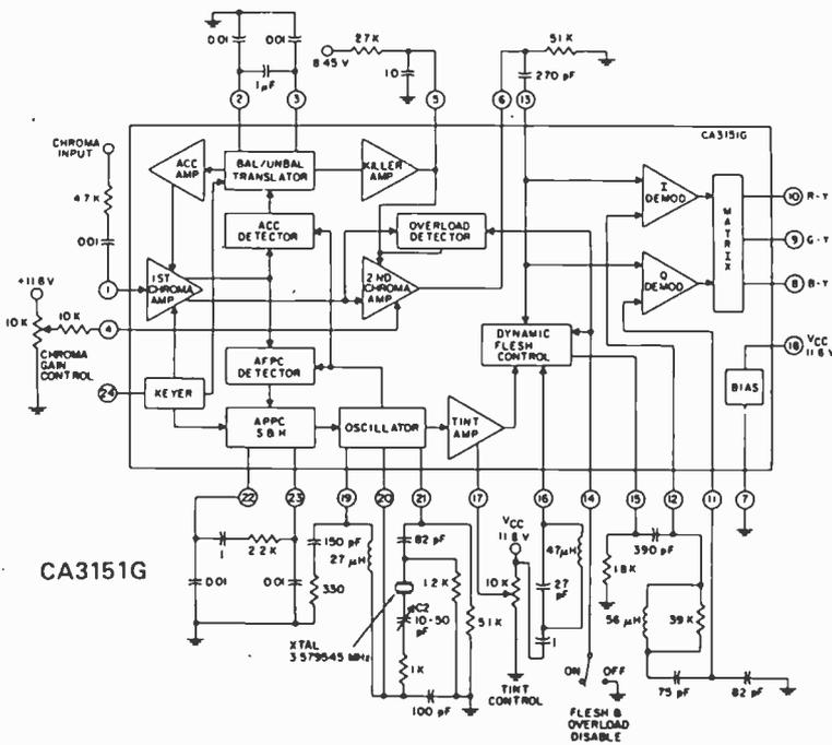
Fig. 3. The CA3151G single-chip chroma processor and demodulator.
