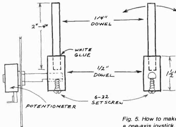
Fig. 5. How to make a one-axis joystick.
