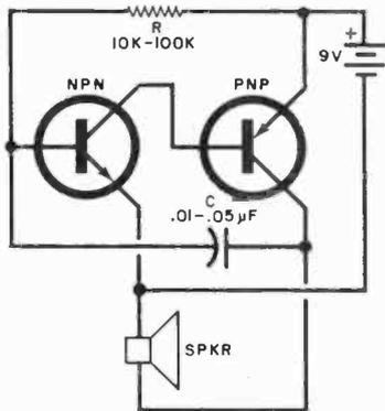
tuting the unknowns. If the oscillator sounds off, you know the unknown transistor's type (npn or pnp), that it works at audio frequencies, and the pinout. Use the other socket for identifying the other types of transistors.
