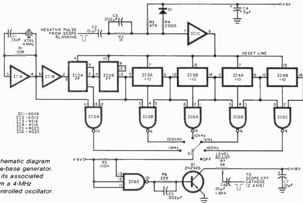
Fig. 1. Schematic diagram of the time-base generator. IC1A and its associated circuit form a 4-MHz crystal-controlled oscillator.
