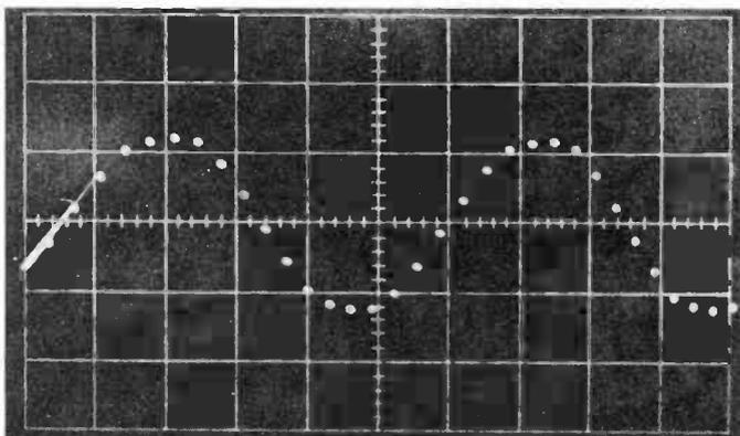
The generator circuit provides 16.7 dot intervals of one full sine wave as shown here.
