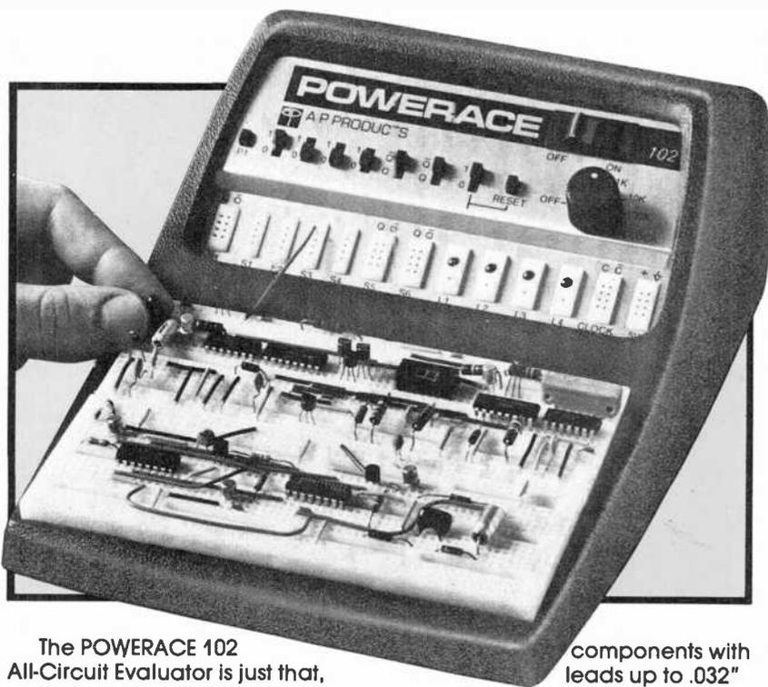
The POWERACE 102 All-Circuit Evaluator is just that, and at a remarkably low price. And its pulse detection with memory plus logic indicators constitute a built-in logic probe.
