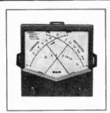
The Daiwa CN-520 uses a cross-needle configuration to measure forward power, reflected power, and resultant SWR on one meter. The unit plugs into an existing antenna system via the included SO-239 connectors. Specs: frequency, 1.8 to 60 MHz; power range, forward 200 W to 2 kW, reflected 40 W to 400 W; accuracy, 10%; detection sensitivity, 40 W, \$70.
