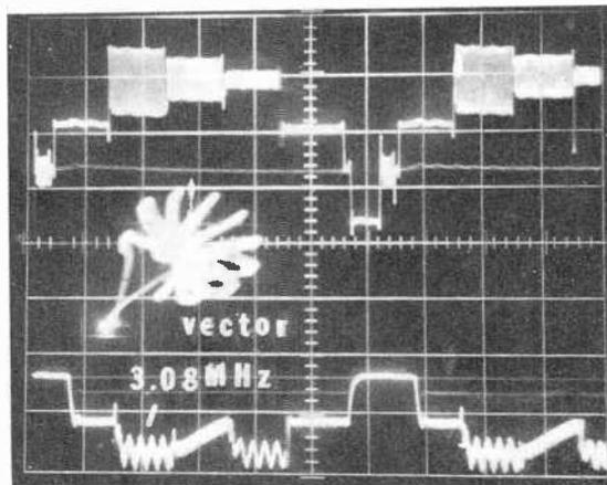
Fig. 6. Swept chroma test at video detector and cathode ray tube. Vector is somewhat irregular.
