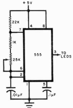
If you wish, substitute a photoresistor for the two resistors between pins 7 and 6-2. The circuit then automatically controls the LED brightness depending on room lighting.
