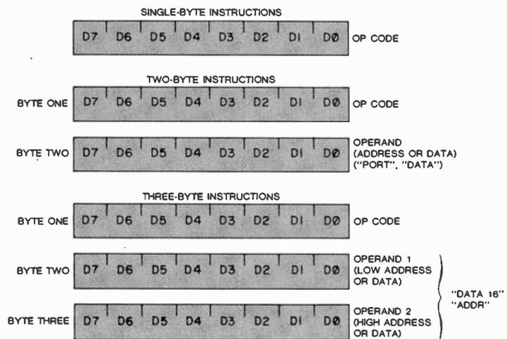
**Fig. 17. 8080 instruction formats.** Typical instructions for single-byte (top) are register-to-register, return, push, and pop; for two-byte: immediate mode and I/O; for three-byte: jump, call, and direct load. D0 is least significant bit; D7, most significant.
