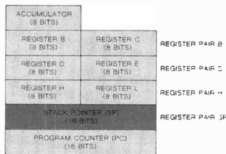
Fig. 18. The 8080 has seven 8-bit general-purpose registers and two 16-bit registers.
