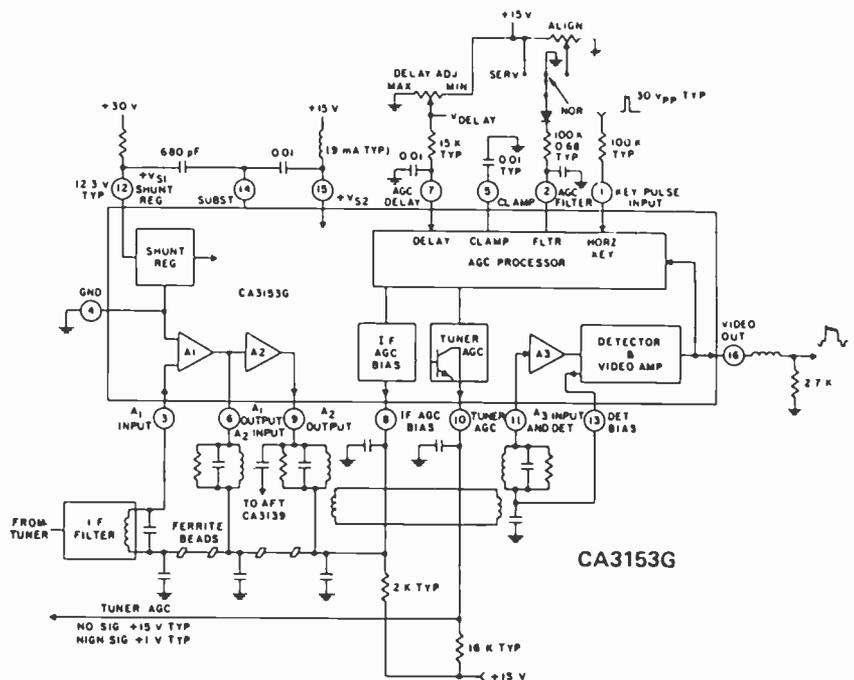
Fig. 2. Functional diagram of the CA3153G video i-f, agc and detector.
