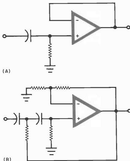
Fig. 2. Simplified active filters: (A) first order and (B) second order.
