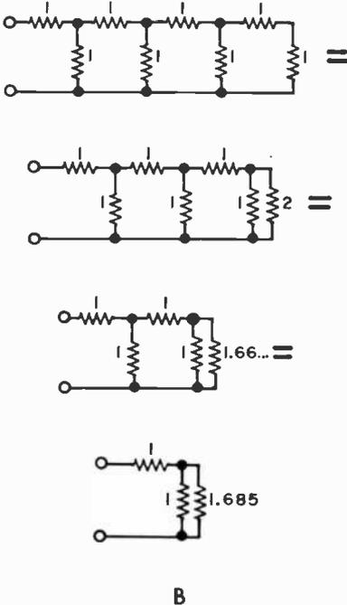
8-resistor network is reduced to just 3 resistors. We can continue this procedure and reduce a network with any number of resistors (even a million or
