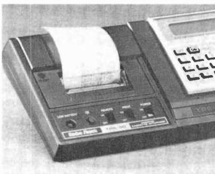
manual. A paper-advance button and papercutter edge are also provided. It uses the computer's PRINT and LIST commands to print a 16-column alphanumeric array. The printer operates at one line per second, and about 8000 lines per battery charge. An indicator alerts to low battery. Several options are available. \$149.95. Address: Radio Shack stores and Computer Centers.
