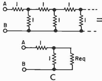
We already know  $Req_1 = 2$  ohms. In the circuit at D,  $Req_2 = 1 + (1 \times 2) / (1 + 2) = 1 + 2/3 = 5/3$ . Then substitute this equivalent resistance in a
