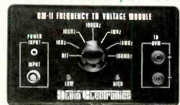
Measure frequencies from 5Hz to 100MHz on your digital voltmeter with a resolution of 312 digits — easy to use — perfect for field service — lab testing — home hobbyist! Connect the DM-11 to your DVM. Set the DVM to the 2VDC range, connect a signal to the DM-11 via a BNC cable (not included) and measure the frequency of any source. Hi Lo Range LED's insure fast accurate readings
