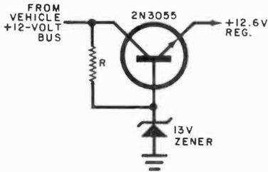
tor fails. Adjust the value of the resistor until the circuit produces +12 volts under load of the CB.
