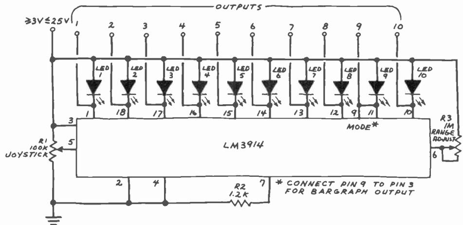
center sequentially activates LEDs 1-6. And moving the stick from lower right to upper right sequentially activates LEDs 1-9. Depending upon R3's adjustment (see Fig. 6), these results may vary by one or two LEDs.
