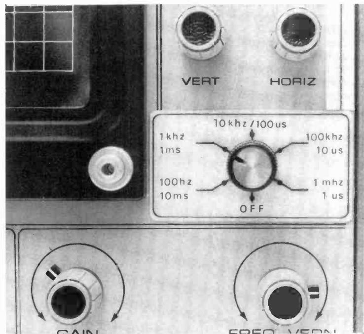
*The switch can be mounted on a vacant space on the scope's front panel, cutting an opening for the shaft, with the circuit board inside.*
