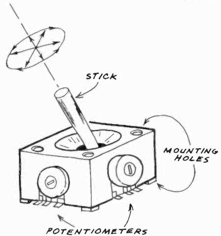
Fig. 1. Three-dimensional representation of a typical two-axis joystick.
