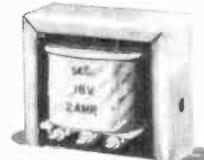
Steel frame. 120VAC primary. Center-tapped 18VAC secondary, rated 2A. 2 1/2" x 2 1/2" x 2". 273-1515 ..... 6.99
