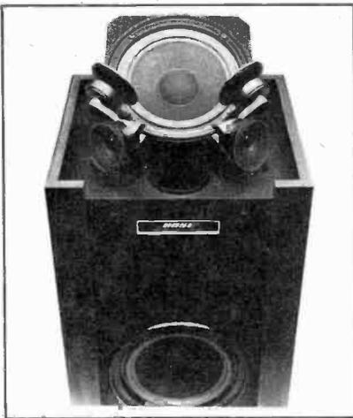
The 601 Series II floor-standing speaker has two 8" long-excursion woofers and four 3" tweeters. Each of the woofers is housed in a separate injection-molded compartment. The tweeters and one woofer are mounted above the main enclosure in a multidirectional array. This is claimed to spread stereo image and reduce mid-bass "boominess" caused by room boundary reflections. Also featured is a
