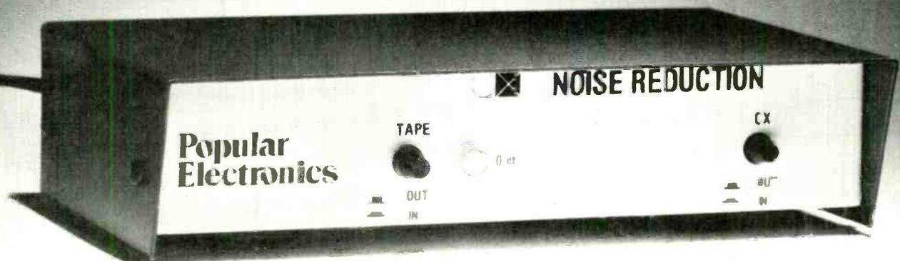
everything below  $-40$  dBV is boosted 20 dB. As the signal increases from  $-40$  dBV to 0 dBV, the gain reduces so that by 0 dBV there is 0 dB or unity gain. Above 0 dBV, the gain continues to fall so that a  $+12$ -dBV input is reduced by a  $-6$ -dB gain for a  $+6$ -dBV output.
