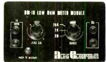
Measures resistance from 10 milliOhms to 20 Ohms. Now you can measure resistance down to 10 milliOhms with this low cost, easy to use DVM module. Check coil resistance, transformers, relays, chokes, printed circuit board copper paths and ground cables. Special zero balance control nulls out input cable resistance to insure accurate readings. Your DVM has to be set to 2V range during operation.
