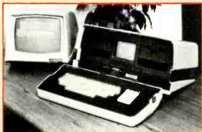
The Osborne 1 computer measures 20.5"W x 13"D x 9"H and weighs 23.5 lb. The main pc board uses the Z80A processor with a 4-MHz clock; memory size is 64K RAM, 4K ROM. Interfaces are RS-232 C and IEEE 488. User controls consist of a 69-key detachable keyboard with a 12-key numeric pad; brightness and con-
