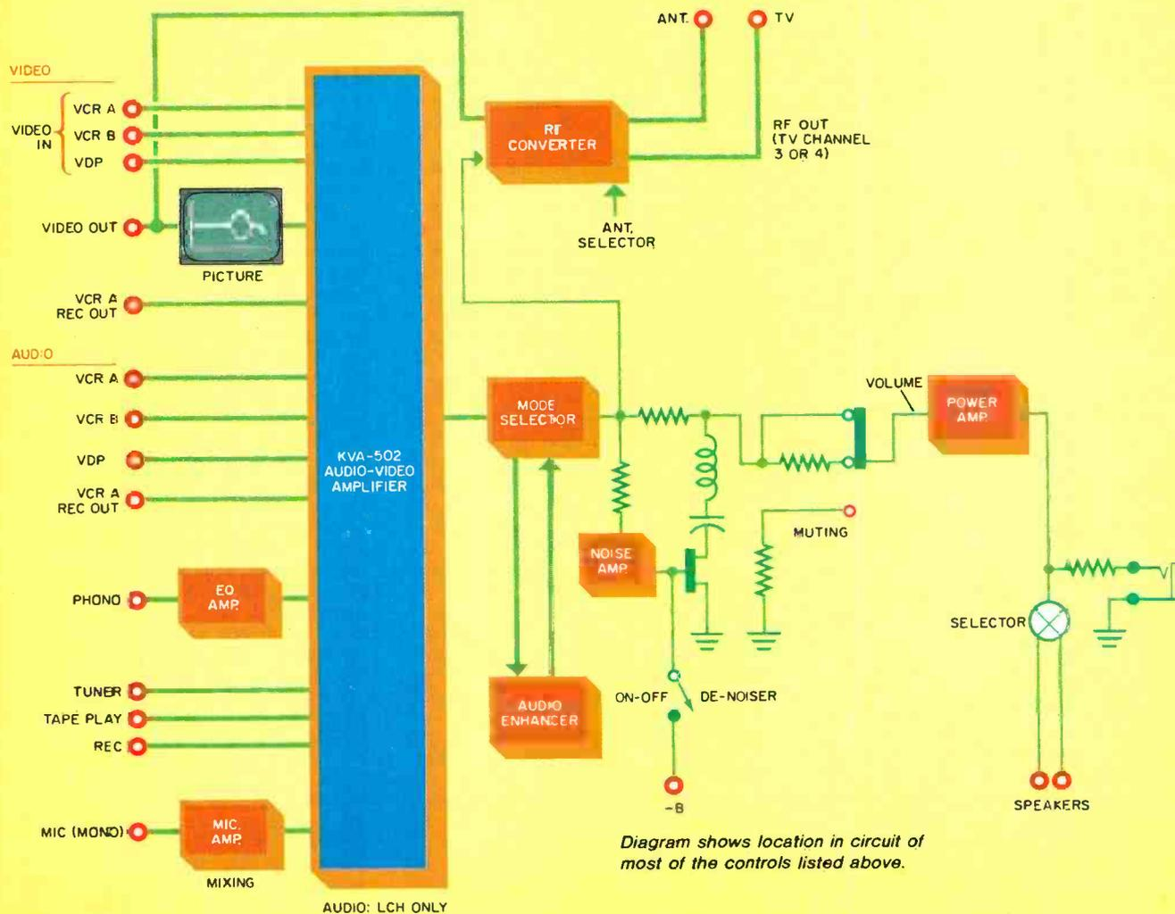
Diagram shows location in circuit of most of the controls listed above.
