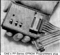
OAE's PP-Series EPROM Programmers plug directly into any vacant EPROM socket and allow you to transfer data directly from RAM to EPROMs. No additional power supplies are required. All timing & control sequences are handled by the programmer. Each unit includes internal DC to DC switching regulator, ZIF socket and 4 ft. ribbon cable terminated with a 24 pin plug. Programmers are available for all EPROMs from 2708's thru 2532's.
