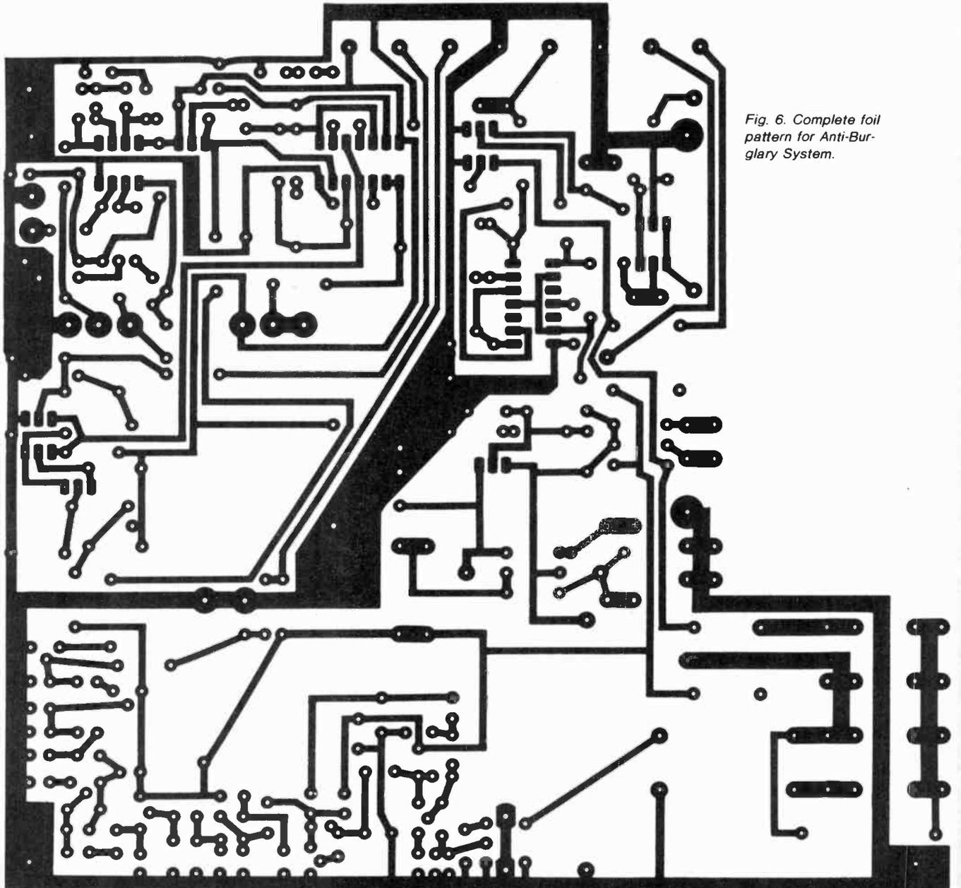
Fig. 6. Complete foil pattern for Anti-Burglary System.
