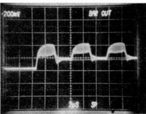
Fig. 4. Output signal from EP playback.
