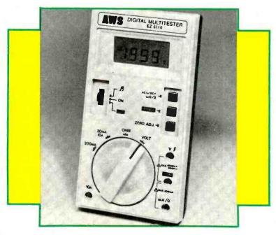
THE Model EZ-6110 Digital Multimeter from A. W. Sperry Instruments, Inc., is a compact, battery-powered, digital test instrument for general-purpose measurements on the workbench and in the field. It has a 3½-digit, 0.4"-tall, high-contrast LCD readout and 24 measurement ranges.
