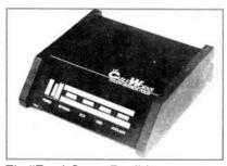
The "Touch Sensor Four" from the Cable Works is designed to maintain the integrity of the different video signals that can be used with a TV receiver. When a receiver is connected to a VCR, video disc, video game, cable TV, home computer, or
