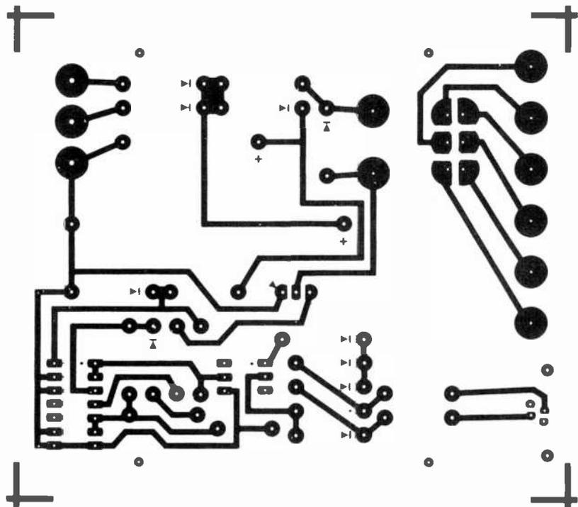
Fig. 4. Full-size etching and drilling guide for the project.
