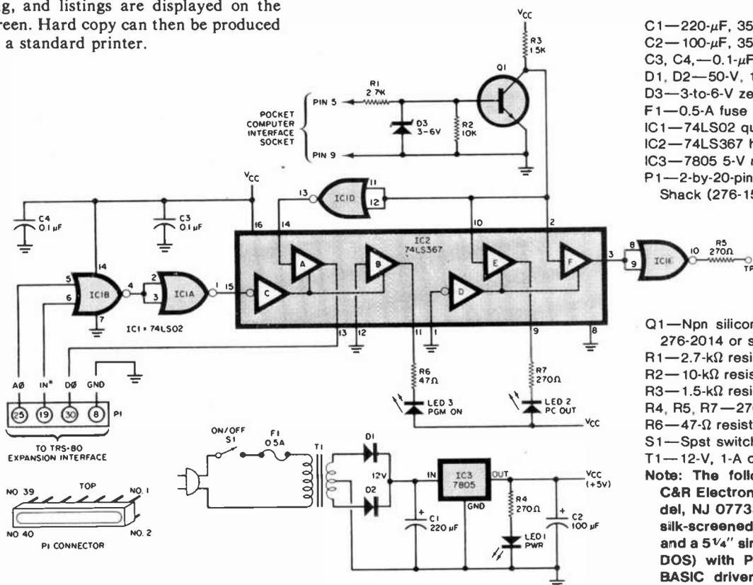
Fig. 2. Schematic of the interface circuit. Included is a regulated power supply.
