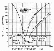
Fig. 5. Tonearm resonance should be between max. warp velocity and min. modulation limits.
