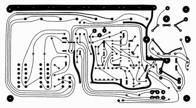
Fig. 4. Actualsize foil pattern for printed-circuit board.
