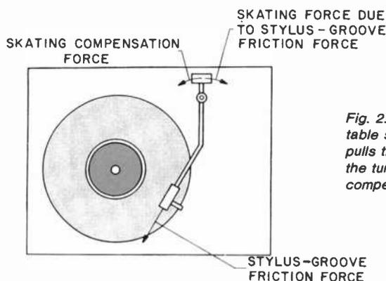
Fig. 2. The usual stylus/tonearm/turntable setup creates an inward force that pulls the tonearm toward the center of the turning platter. Antiskating compensation counteracts this effect.
