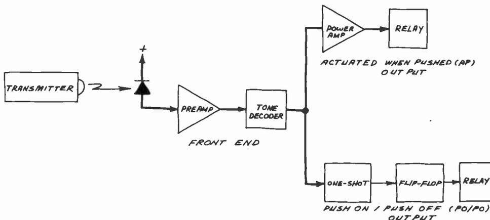
Fig. 1. Block diagram of a single-channel remote-control system.
