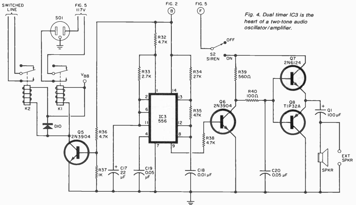
Fig. 4. Dual timer IC3 is the heart of a two-tone audio oscillator/amplifier.
