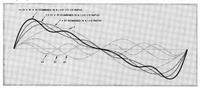
Fig. 5. Approximation by Fourier analysis of a 1-kHz sawtooth waveform.
