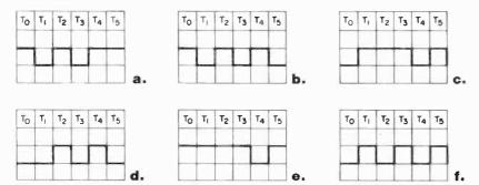
Answers: I. d (AND gate, all inputs high to get a high output.) 2. c (OR gate, any input high to get a high output.) 3. c (NAND gate, any input low to get a high output.) 4. b (NOR gate, all inputs low to get a high output.) 5. f (Exclusive-OR gate, either input high, but not both, to get a high output.) 5. f (Exclusive-OR gate, either input high, but not both, to high output.) 6. a (INVERTER, the output is the opposite of the input.)
