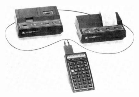
The HP-IL Interface Loop gives the HP-41 mass memory and printing capability with a Cassette Drive and Thermal Printer/Plotter.
