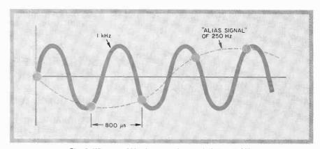
Fig. 2. When a 1-kHz sine wave is sampled at 1.25 kHz, the samples give an "alias signal" of 250 Hz.
