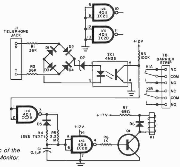
Fig. 1. Schematic of the Telephone Status Monitor.
