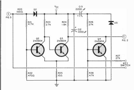
Fig. 3. Transistors Q2 and Q3 form a Schmitt trigger that prevents false activation under low voltage conditions.
