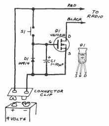
od of 70 minutes," he writes. "During the last few minutes the FET operates in its linear region, slowly pinches off the current to the radio and provides a built-in fade. Both the Radio Shack VN10KM and VN67AF VMOS FETs worked well, but if the radio has a large supply bypass capacitor, the higher power VN67AF is the one to use to avoid troubles with excessive capacitive loading. My friend says he has never slept better."
