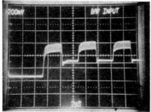
Fig. 2. Color-bar input signals.
