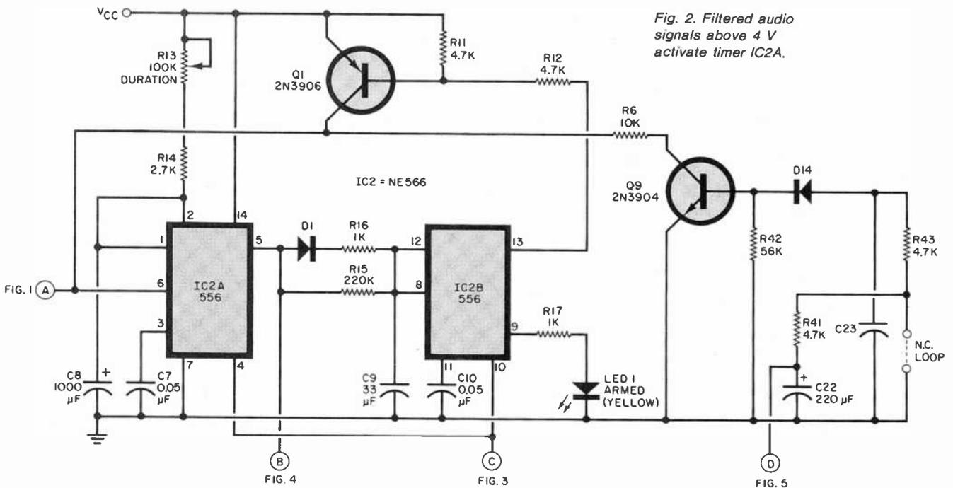
Fig. 2. Filtered audio signals above 4 V activate timer IC2A.
