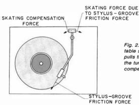
Fig. 2. The usual stylus/tonearm/turnpulls the tonearm toward the center of the turning platter. Antiskating
