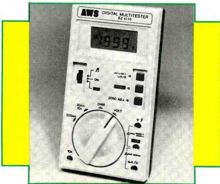
**T**HE Model EZ-6110 Digital Multimeter from A. W. Sperry Instruments, Inc., is a compact, battery-powered, digital test instrument for general-purpose measurements on the workbench and in the field. It has a 3½-digit, 0.4"-tall, high-contrast LCD readout and 24 measurement ranges.
