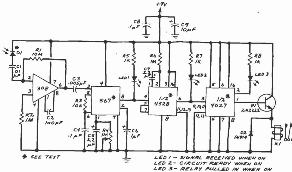
Fig. 4. Complete schematic for an infrared remote-control receiver.
