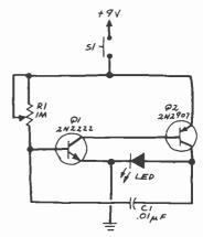
Fig. 3. Alternative infrared transmitter.
