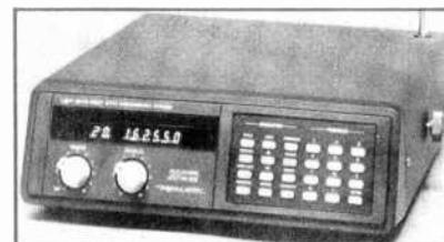
Radio Shack's 20-channel scanning receiver, Realistic PRO-2020, is an FM/AM direct entry programmable unit for home or mobile use. It covers six vhf and
