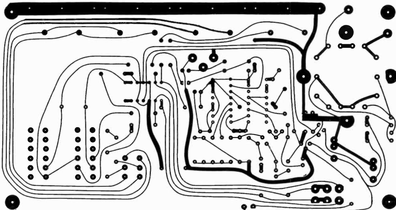
Fig. 4. Actual-size foil pattern for printed-circuit board.
