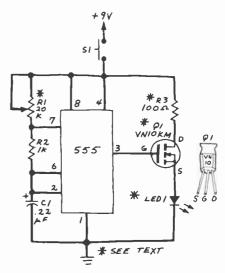
Fig. 2. Infrared remote-control transmitter.
