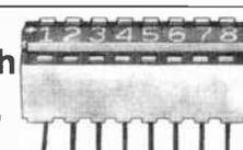
8-position switch for digital or low-current use. Mounts in a 16-pin DIP socket or on PC boards.
