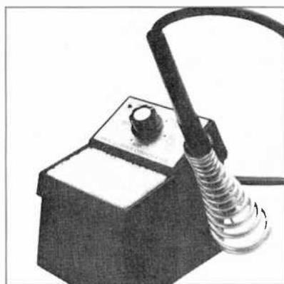
The Iso-Tip 7470 Micro Soldering Station is reported to eliminate continuous switching (and the voltage spikes that can damage electrical equipment) by maintaining an even tip temperature. The unit is totally grounded and can be adjusted to any temperature between 500° and 700°F. It comes with a sponge holder, tip-wiping sponge, soldering iron, and stand (which takes up 12 sq. in. of bench space).
