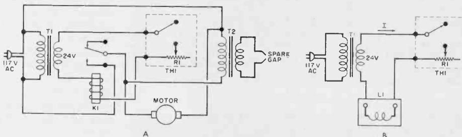
Most, but not all, oil and gas furnaces use low-voltage (24 V ac) thermostat control systems. Figure A shows a simplified wiring diagram of a typical oil-fired furnace. *T1* is a 24-V transformer and *TH1* is a low-voltage thermostat with an adjustable heat anticipator (resistance *R1*). Relay *K1* has normally open contacts and a 24-V ac coil. The oil-pump motor and ignition transformer *T2* lead to the spark gap. (Numerous safety-related circuits and com-
