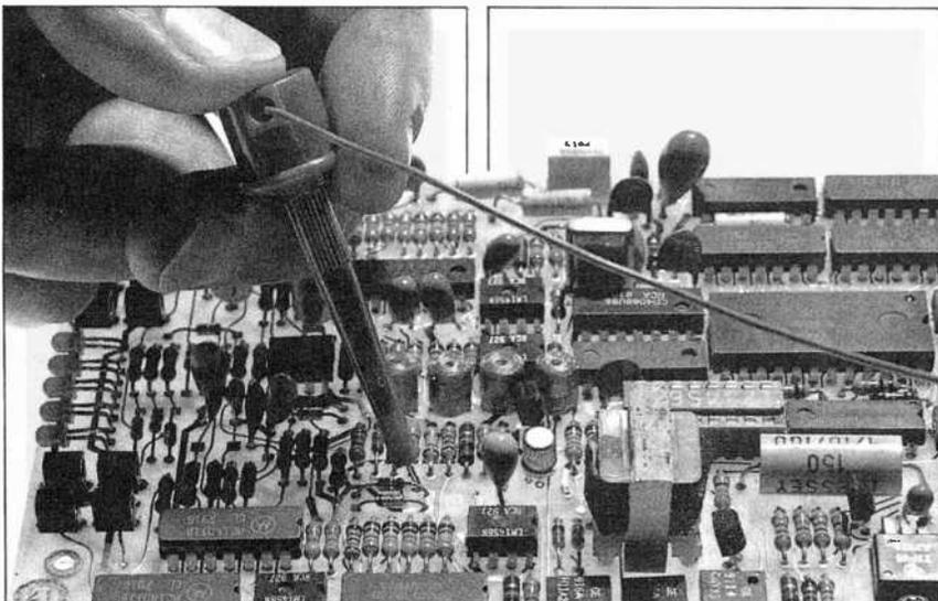
**P**robe-It™—the faster and easier way to test component leads. Just press the cap to extend the hook contact, place on the lead or wire and release for hands-free troubleshooting.
