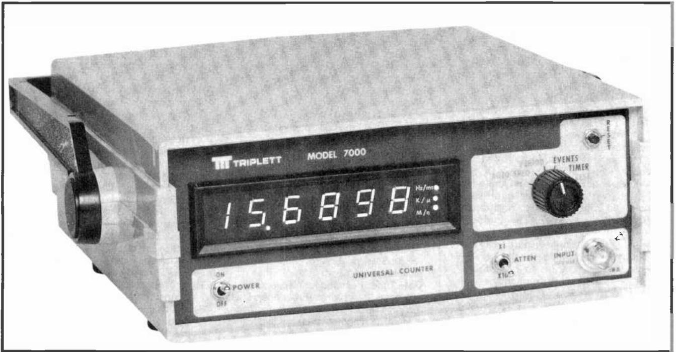
The Triplet Model 7000 Universal Counter is a microprocessor-based 5-Hz to 80-MHz autoranging counter having six-digit resolution. It also has two accumulating-type functions—EVENTS, which can total to one-billion at rates to 80 MHz, and TIMER, which can display elapsed time in hours, minutes, and seconds for 100 hours with up to 100  $\mu$ s resolution. A built-in TEST function verifies proper operation.
