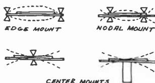
Fig. 2. Three mounting arrangements for piezoelectric alerter elements.
