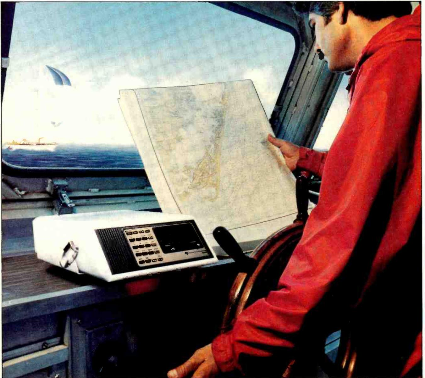
**M**IX the serious boating enthusiast's need for accurate navigation when out of sight of a coastline with today's electronics, and you get a minor miracle called Loran-C (Long Range Aid to Navigation). And with equipment prices down from \$20,000 to under \$1000, you don't have to be a wealthy yachtsman to enjoy its benefits.
