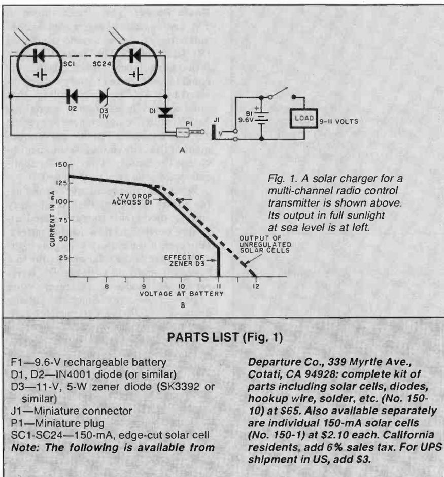
by 5-volt regulator *IC1*. Always include a blocking diode (like *D1*) to prevent discharge when the solar cells are in the dark. The charger is placed on the workbench close to a window, and receives about two hours of sunlight per day, about four days per week in winter.
