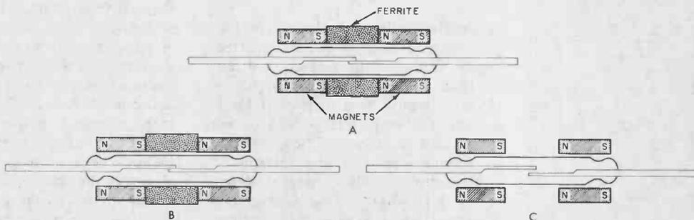
A temperature-sensing reed switch consists of a rhodium-contact reed switch hermetically sealed in glass, two permanent magnets that surround the glass, and a ferrite ring sandwiched between the magnets (Fig. A). The switch depends on the interaction of the magnets and the ferrite for its operation.
