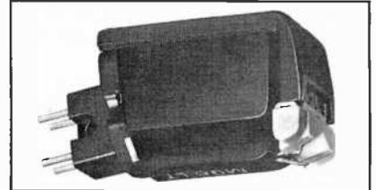
Shure Brothers has announced a new direct plug-in phono cartridge especially designed for use with linear-tracking turntables. Designated Model M96LT, it has a telescoped shank structure and a lightweight magnet reported to give a frequency response flat from 20 to 20,000 Hz. The cartridge has a bi-radial elliptical diamond stylus that tracks at 1.25 g. \$80.
