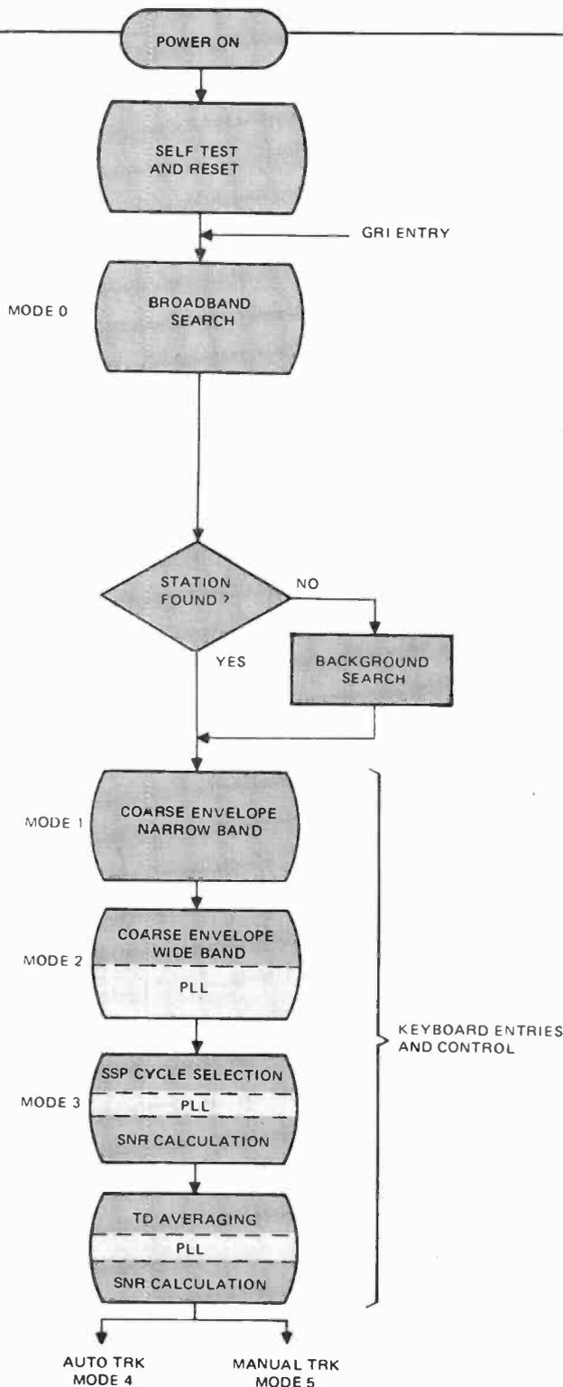
Fig. 6. At right is a flow chart showing the sequence of events taking place inside a receiver. A block diagram of the Texas Instruments TI-9000 receiver is shown on the opposite page.
