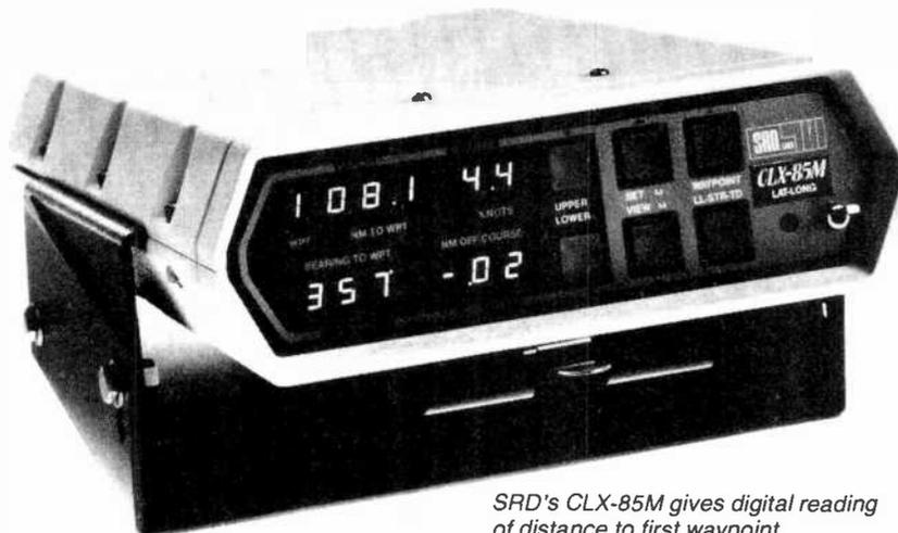
SRD's CLX-85M gives digital reading of distance to first waypoint, bearing, distance off course, and cruising speed.
