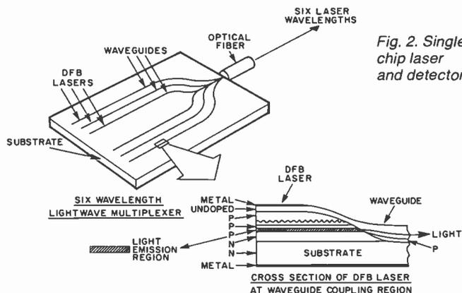
Fig. 2. Single-chip laser and detector.
