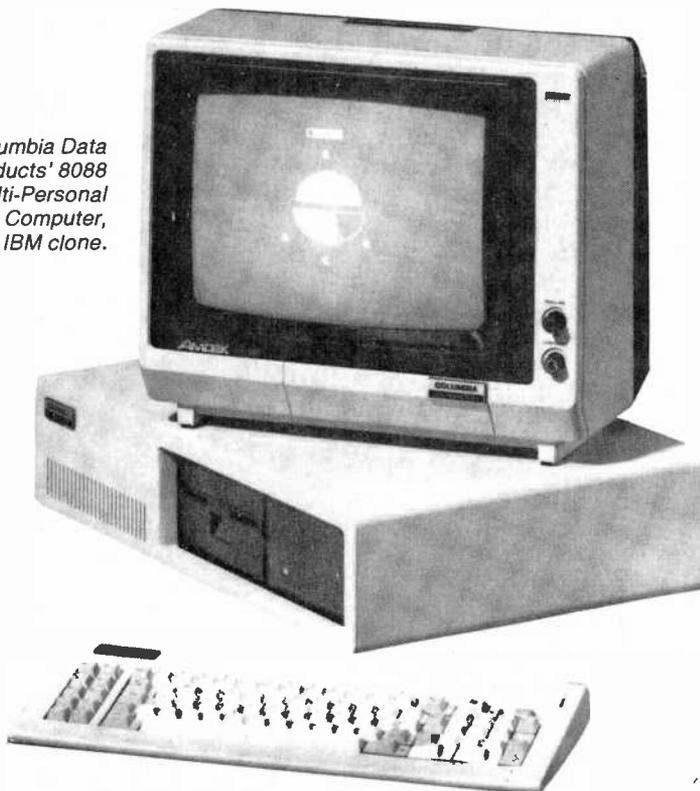
ing Greek, foreign language special characters, and mathematical symbols. The graphics display format is 640 dots wide by 250 (or 200) dots high, fully addressable array; or 320 dots wide by 250 (or 200) dots high, with 4-level grey scale. The I/O includes the RS-232C standard with an asynchronous 75-to-19.2K baud rate or synchronous 100K with bisync and bit-oriented protocols. The parallel port is compatible with IBM/Epson or Centronics printers.
