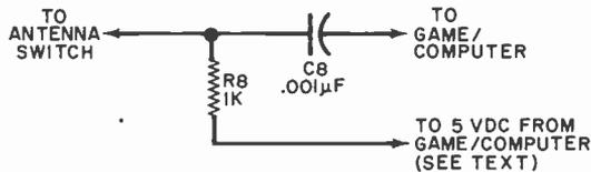
Fig. 6. Circuit for adapter box connected to game or TV.
