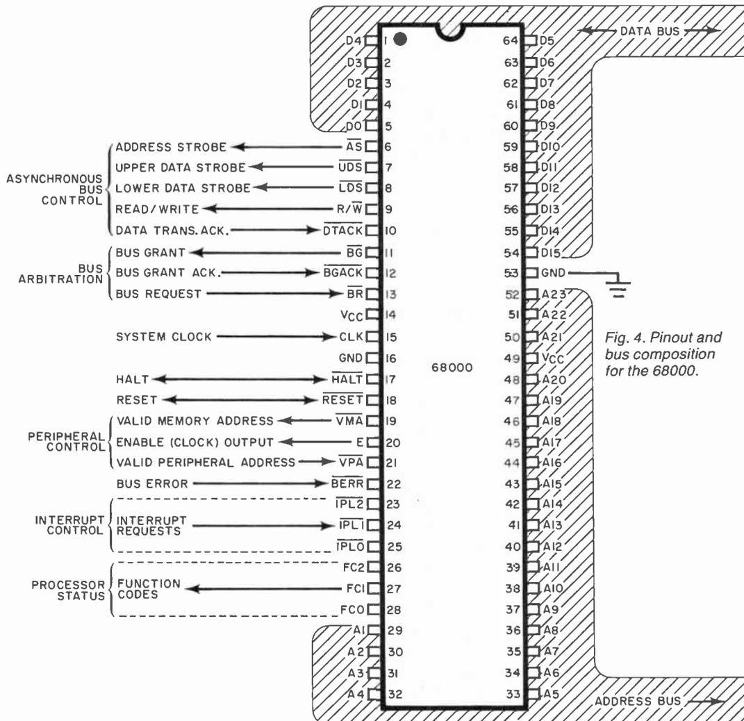
Fig. 4. Pinout and bus composition for the 68000.
