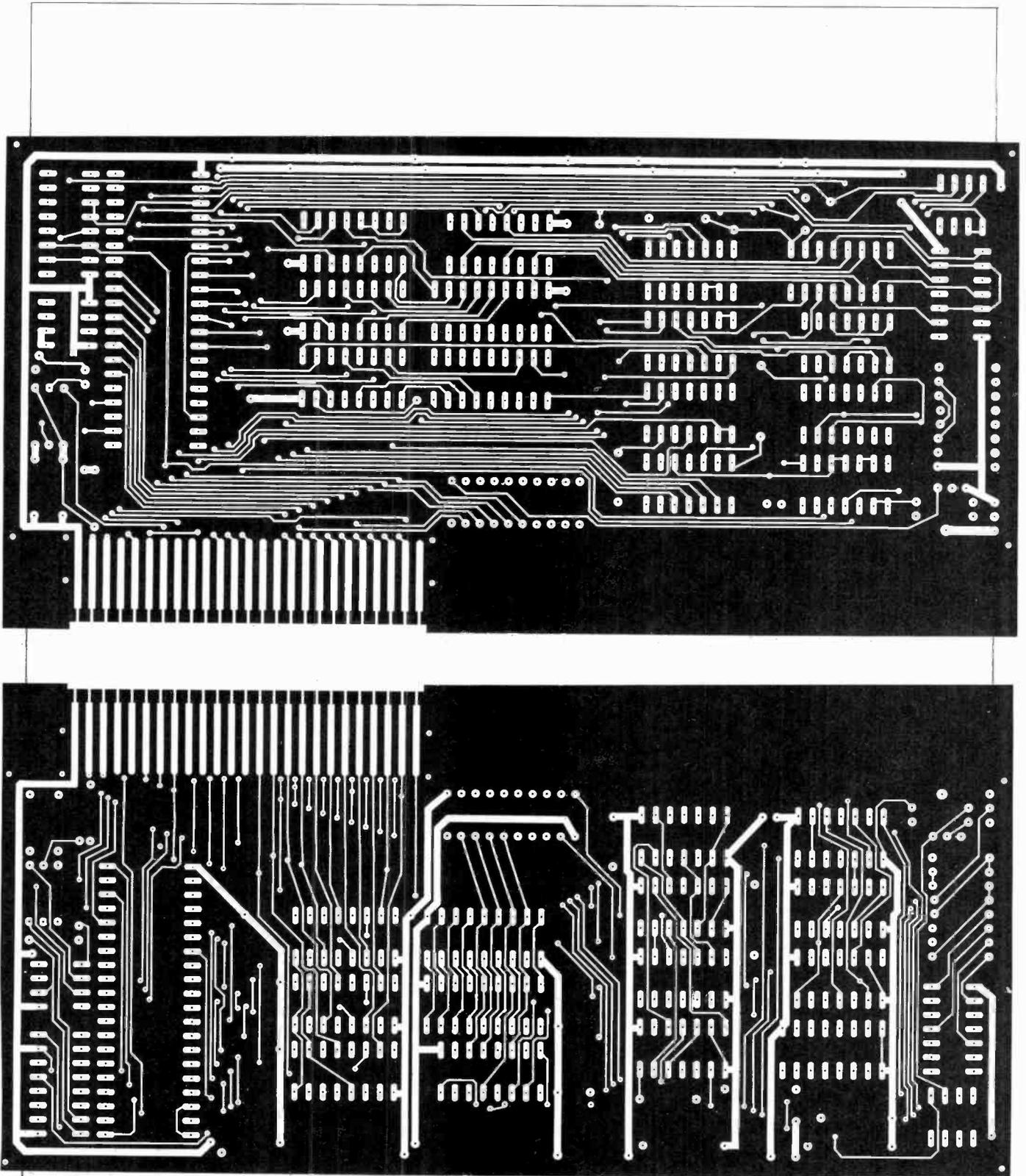
Fig. 6. Foil patterns for the double-sided printed circuit board.
