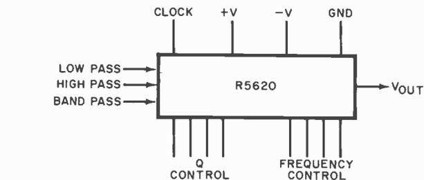
Fig. 2. External connections to R5620 Universal Active Filter.
