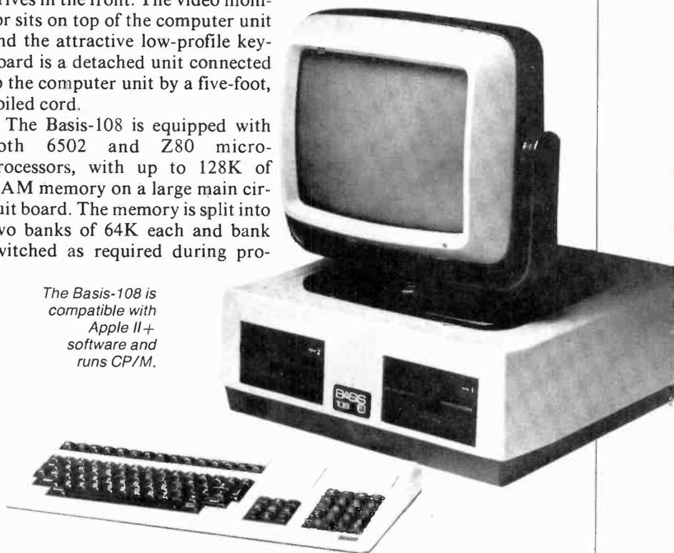
*The Basis-108 is compatible with Apple II+ software and runs CP/M.*
