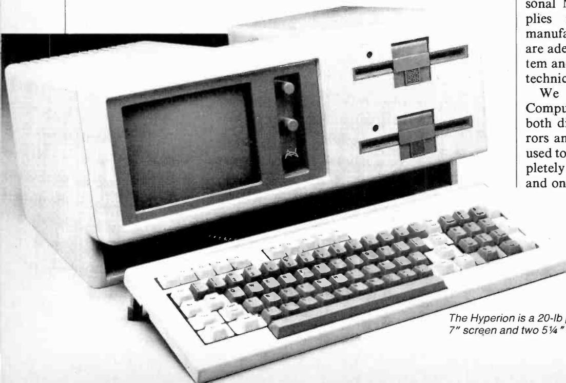
The Hyperion is a 20-lb portable with 7" screen and two 5 1/4" disk drives which run PCDOS.
