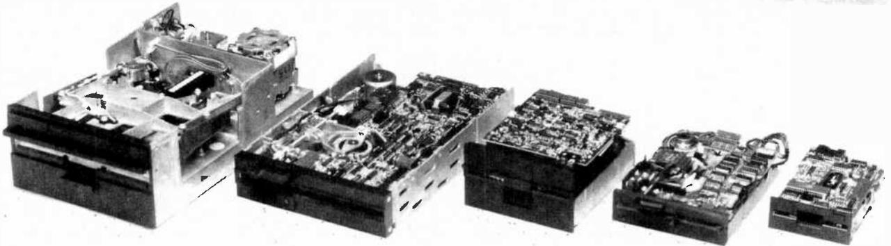
The shrinking world of disk drives is shown by a conventional 8" at left, followed by a half-size 8", conventional and half-size 5¼", and 3½" drive at far right.
