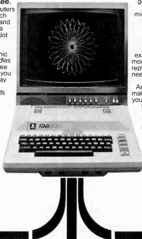
**Sound.** An ATARI computer has four sound generators, or voices, activated by a separate microchip. This leaves the principal microprocessor chips free to perform other tasks. And you can take full advantage of this capability which is designed for easy programming.
