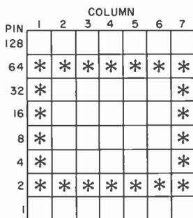
Fig. 4. Converting a shape to numbers.
