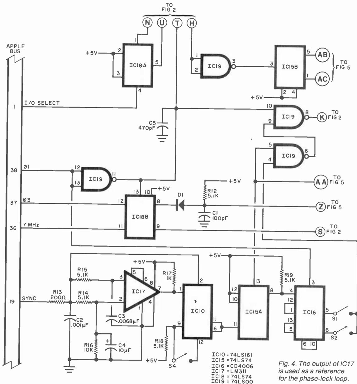
Fig. 4. The output of IC17 is used as a reference for the phase-lock loop.
