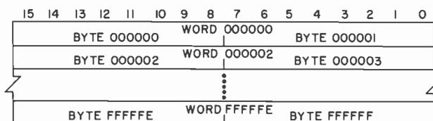
Fig. 2. The memory organization can directly address  $2^{24}$  bytes.
