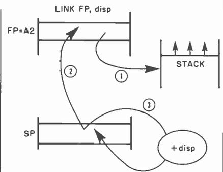
Fig. 3. How the LINK basic instruction is implemented.
