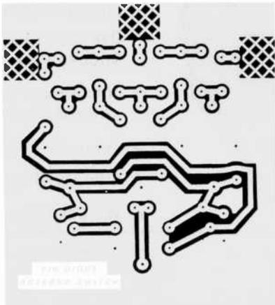
Fig. 4. Foil pattern for the printed circuit board.
