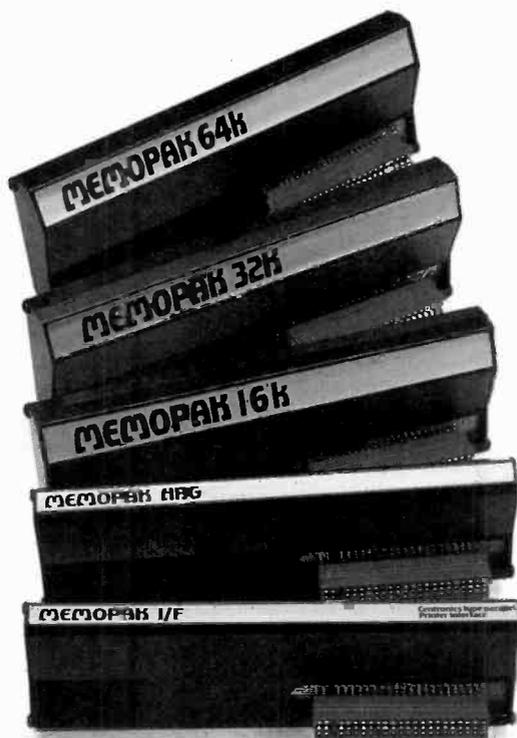
**Memopak 64K RAM** The 64K RAM extends the memory of your Sinclair by 56K to a full 64K. It is directly addressable, user transparent, is neither switched nor paged and accepts such BASIC commands as 10 DIM A (9000). The Memopak 64K turns your Sinclair into a powerful computer suitable for business, recreational and educational use. No additional power supply is required.
