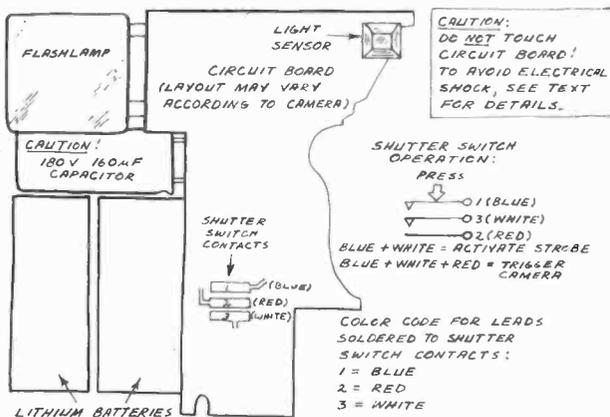
Fig. 5. Connecting leads to the shutter switch terminals.
