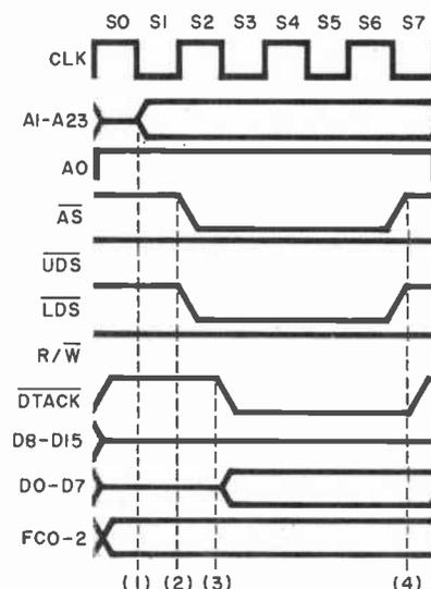
Fig. 5. Timing diagram of a byte read cycle.
