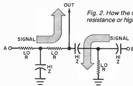
Fig. 2. How the diodes present either low resistance or high capacitance to the input.
