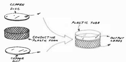
Fig. 1. Pressure-sensitive resistor.
