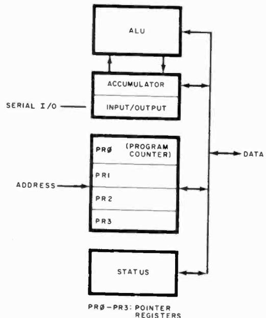
Fig. 2. Generalized block diagram of INS8075 chip.
