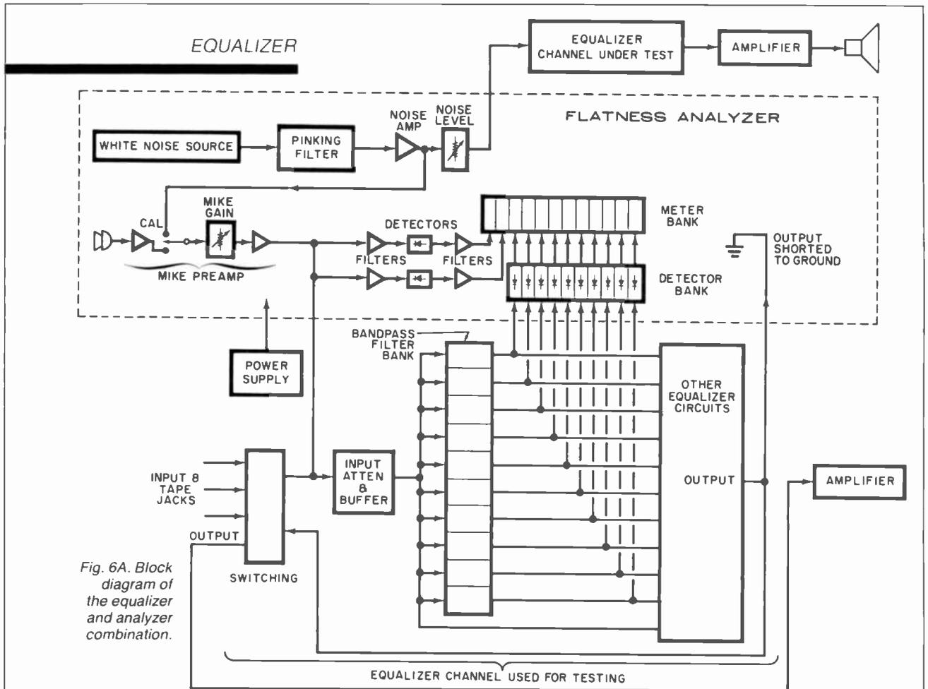
Fig. 6A. Block diagram of the equalizer and analyzer combination.
