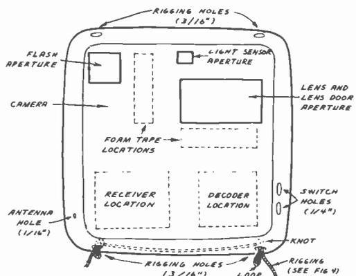
Fig. 3. Bottom view of camera package.
