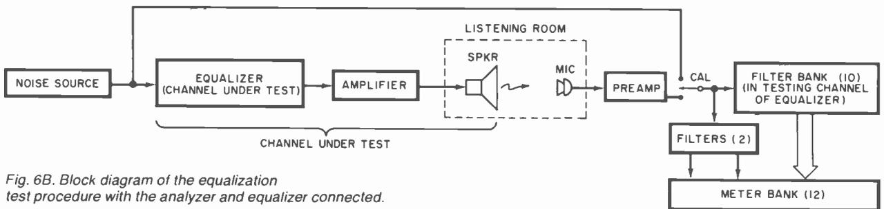
Fig. 6B. Block diagram of the equalization test procedure with the analyzer and equalizer connected.
