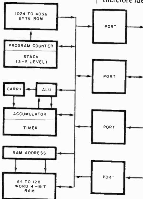
Fig. 1. Block diagram of the AMI S2000 series.
