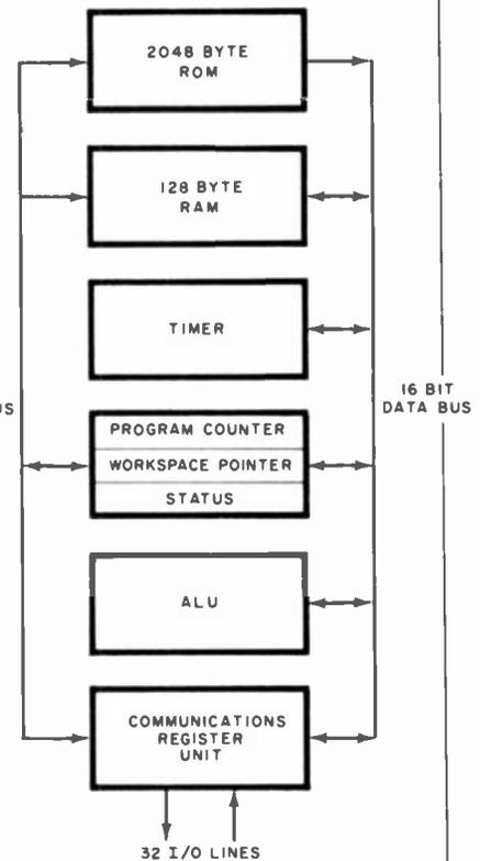
Fig. 3. Texas Instrument's TMS 9940 16-bit chip.
