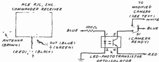
Fig. 1. Connecting RC receiver to camera.
