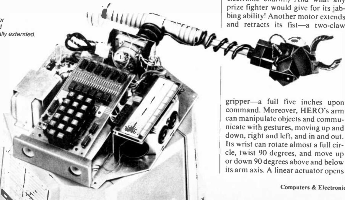
gripper—a full five inches upon command. Moreover, HERO's arm can manipulate objects and communicate with gestures, moving up and down, right and left, and in and out. Its wrist can rotate almost a full circle, twist 90 degrees, and move up or down 90 degrees above and below its arm axis. A linear actuator opens
