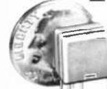
Just 1 1/2 x 3/8 x 1/4" SPDT contacts: 1 amp at 125VAC. 55-ohm. 90 mA coil. .100" centers.
