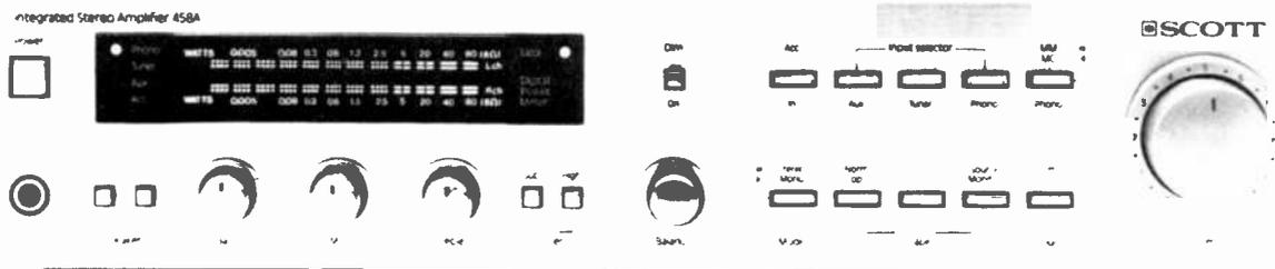
**T**HE 458A, currently heading Scott's line of integrated stereo amplifiers, is rated to deliver 65 watts per channel to 8-ohm loads, between 20 and 20,000 Hz, with no more than 0.03% total harmonic distortion. The 458A has phono preamplification for both moving magnet (MM) and moving coil (MC) cartridges, dual autoranging fluorescent power meters with peak-hold, and pushbutton mode and program selection.
