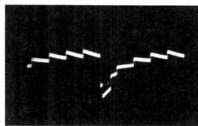
Fig. 2. Staircase signal: input (top) and output (bottom).
