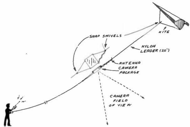
Fig. 5. Taking an oblique-away photo from kite.
