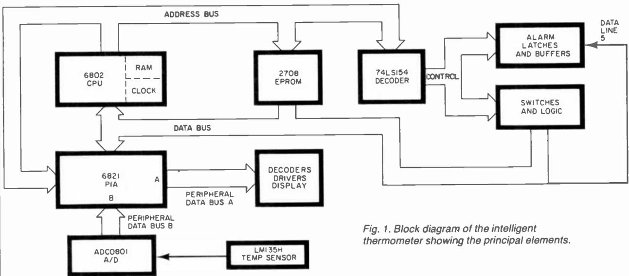
Fig. 1. Block diagram of the intelligent thermometer showing the principal elements.
