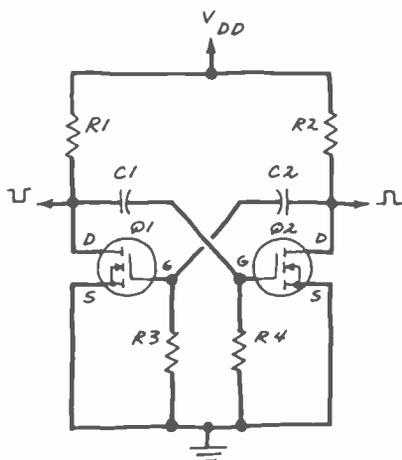
Fig. 1. Multivibrator made with a pair of VMOS MOSFETs.
