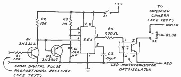
Fig. 2. Pulse-proportional RC decoder.
