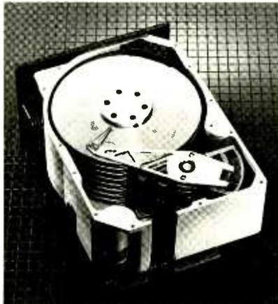
Maxtor's new 5 $\frac{1}{4}$ " Winchester has 140M bytes on eight plated disks.
