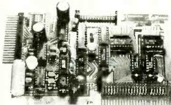
**Fast 1 bus** A/D conversion time 100 ns acquisition window 1 us D/A settling time 8 bits 0-5V or 0-2.5V full scales Board allows re arrangement of the pins and other features for easy interfacing to many types of host computers including Sinclair, Apple, TRS80 others. Switches set address. Address picks channel. Inquire about KITS and software. Assembled and tested \$230. Aluminum box and ribbon cable \$15.
