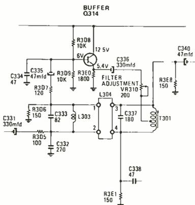
Schematic of the comb filter section of the tuner.
