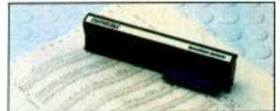
TS-1000 or other Memopaks. **MEMOPAK HRG** The Memopak High Resolution Graphics, with up to 192 by 248 pixel resolution, enables display of high resolution "arcade game" style graphics through its resident 2K EPROM, programmed with a full range of graphics subroutines.
