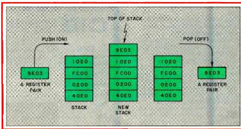
Fig. 4. Stack manipulation.
