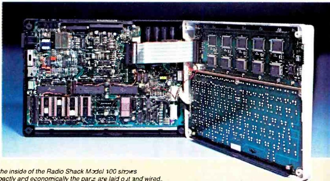
Photo of the inside of the Radio Shack Model 100 shows how compactly and economically the parts are laid out and wired.
