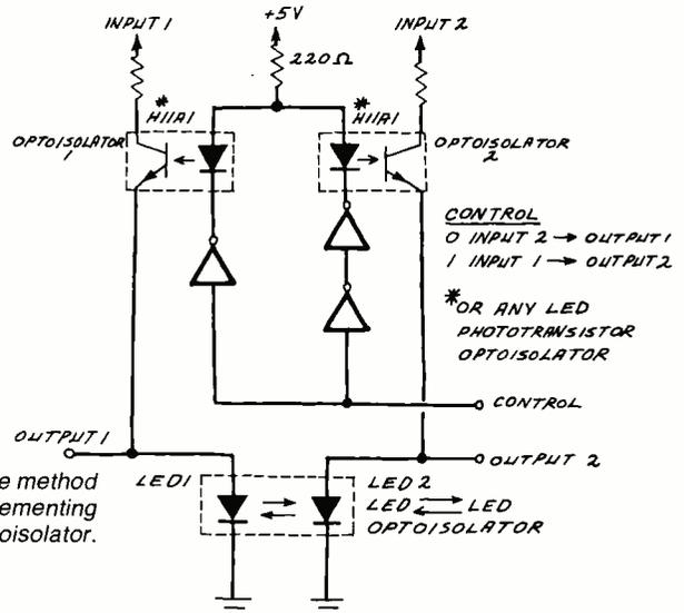
Fig. 3. One method for implementing two-way optoisolator.
