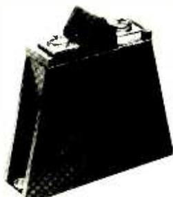
Fig. 4. The high-energy varistor at left protects against transients having peak currents of 70,000 amperes and energies of 10,000 joules.
