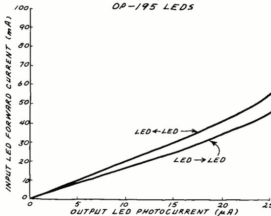
Fig. 2. LED/LED optoisolator current transfer.
