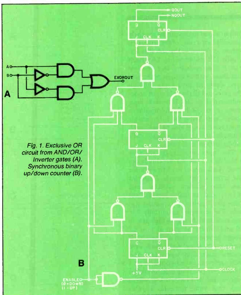
Fig. 1. Exclusive OR circuit from AND/OR/Inverter gates (A). Synchronous binary up/down counter (B).
