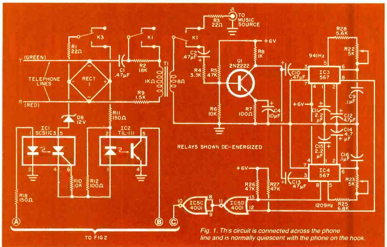
Fig. 1. This circuit is connected across the phone line and is normally quiescent with the phone on the hook.
