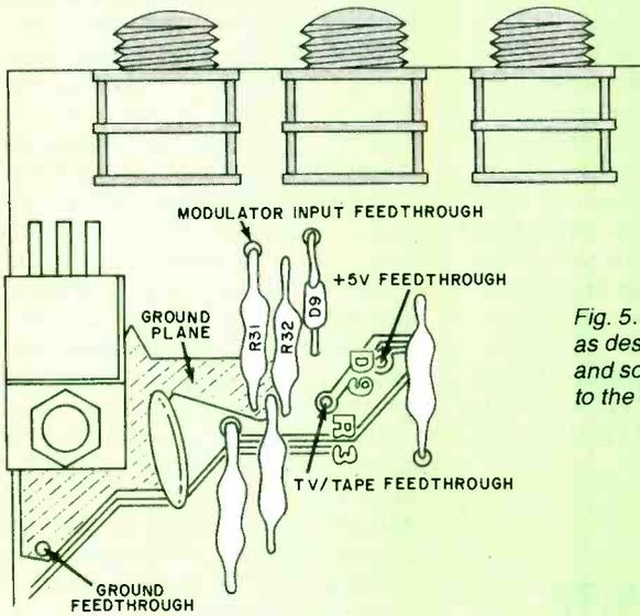
Fig. 5. Remove components as described in the text and solder four wires to the holes as indicated.
