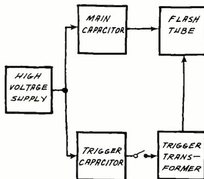
Fig. 1. Block diagram of a flash-tube trigger circuit.
