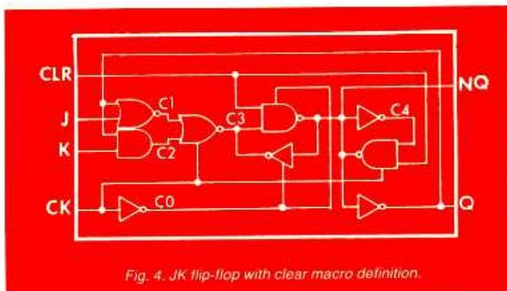
Fig. 4. JK flip-flop with clear macro definition.
