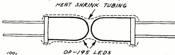
Fig. 1. How to assemble a LED/LED optoisolator.
