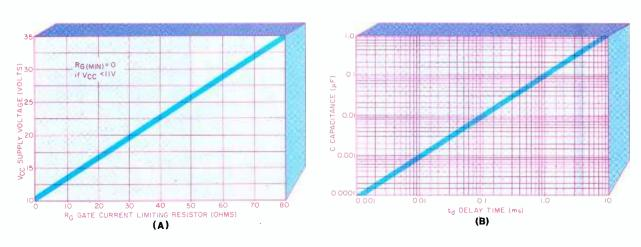
Fig. 2. The curve at (A) is used to select a value of Rg for the SCR and (B) is to choose a bypass capacitor for IC1.
