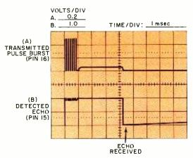
Fig. 9. Waveforms at target detection.
