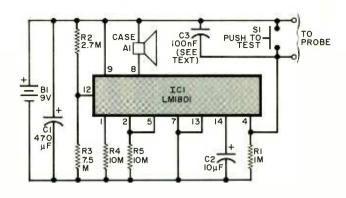
Fig. 1. The heart of the circuit is the LM1801 battery-operated alarm.
