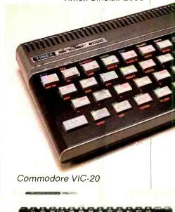
The unit has a built-in r-f modulator and cassette interface. The cassette interface, which runs at 1500 baud, can load or save 48K of memory in less than two minutes. All information saved to tape is started with a header containing information as to its type, title, length, and address information. Programs, screens, blocks of memory, and string and character arrays can all be saved separately, as well as verified if desired. Programs and arrays
