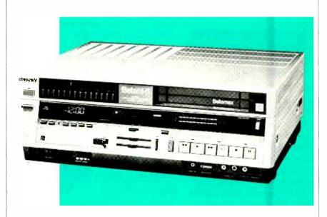
Distortion of the audio track in a VCR is fairly high, too. Harmonic distortion is typically as great as 3%, for maximum recording level. Furthermore, until recently, the audio track on both VHS- and Beta-format machines has been limited to monophonic, or single-channel, sound.
