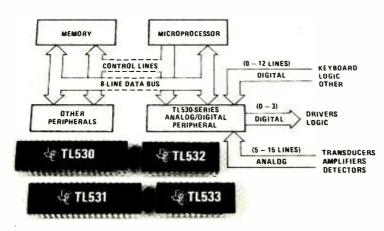
Fig. 14. Block diagram shows operation of TI's CMOS A/D converters.
