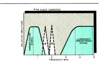
Fig. 2. In Beta Hi-Fi, extra FM audio carriers are inserted in the frequency baseband between chroma and luminance signals.
