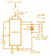
Fig. 12. Off-after-delay timer.
