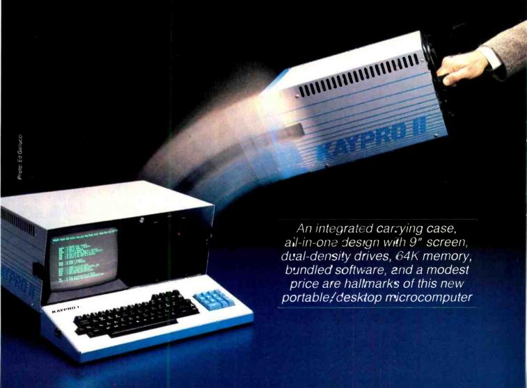
concealed as it is on the Osborne. When detached, the keyboard is connected to the computer through a plug-in telephone-type coiled cable. For travelling overseas, the Kaypro can be set to operate from 220 V ac.
