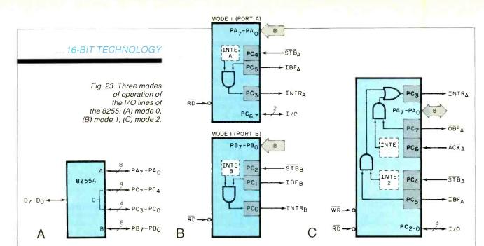
lines are used for a bidirectional bus and five lines for handshaking (borrowing one line from the other group).
