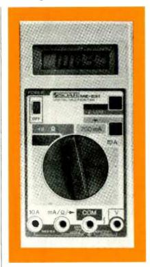
Lockheed Electronics Instrumentation Measurements Laboratory (Plainfield, NJ) against standards traceable to the National Bureau of Standards. After the tests, the IML issued a certificate attesting that the Model ME-531 met its claimed specifications in all respects.
