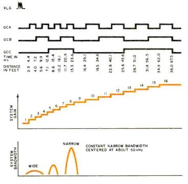
Fig. 5. Operation of gain control logic circuit.
