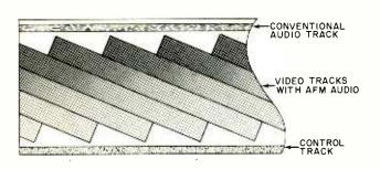
Fig. 3. Audio "r-f" carriers are recorded on video tape using same tape heads that record picture information.
