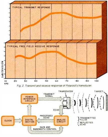
Fig. 3. Block diagram of Ultrasonic Circuit Board.
