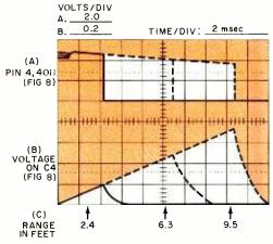
Fig. 10. Waveforms of audible output circuit.
