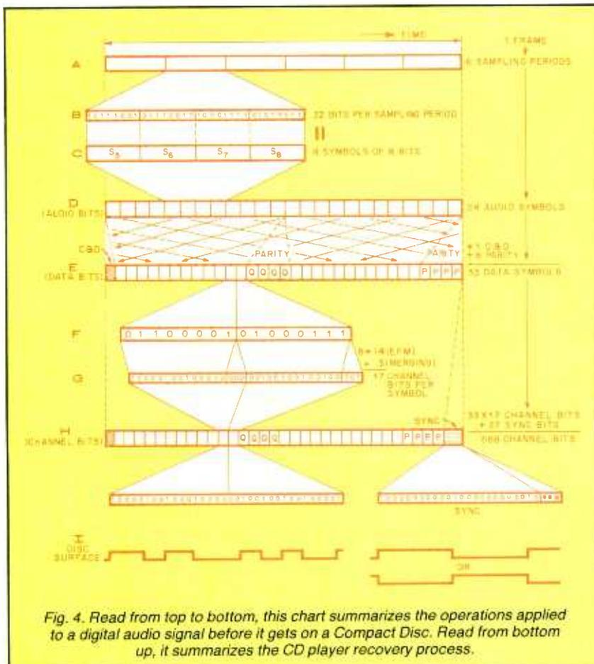
Fig. 4. Read from top to bottom, this chart summarizes the operations applied to a digital audio signal before it gets on a Compact Disc. Read from bottom up, it summarizes the CD player recovery process.
