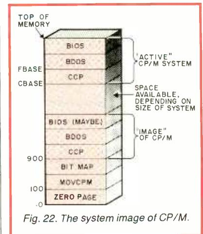
Fig. 22. The system image of CP/M.
