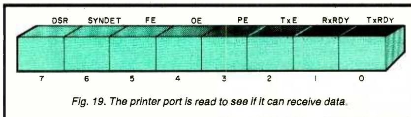
Fig. 19. The printer port is read to see if it can receive data.
