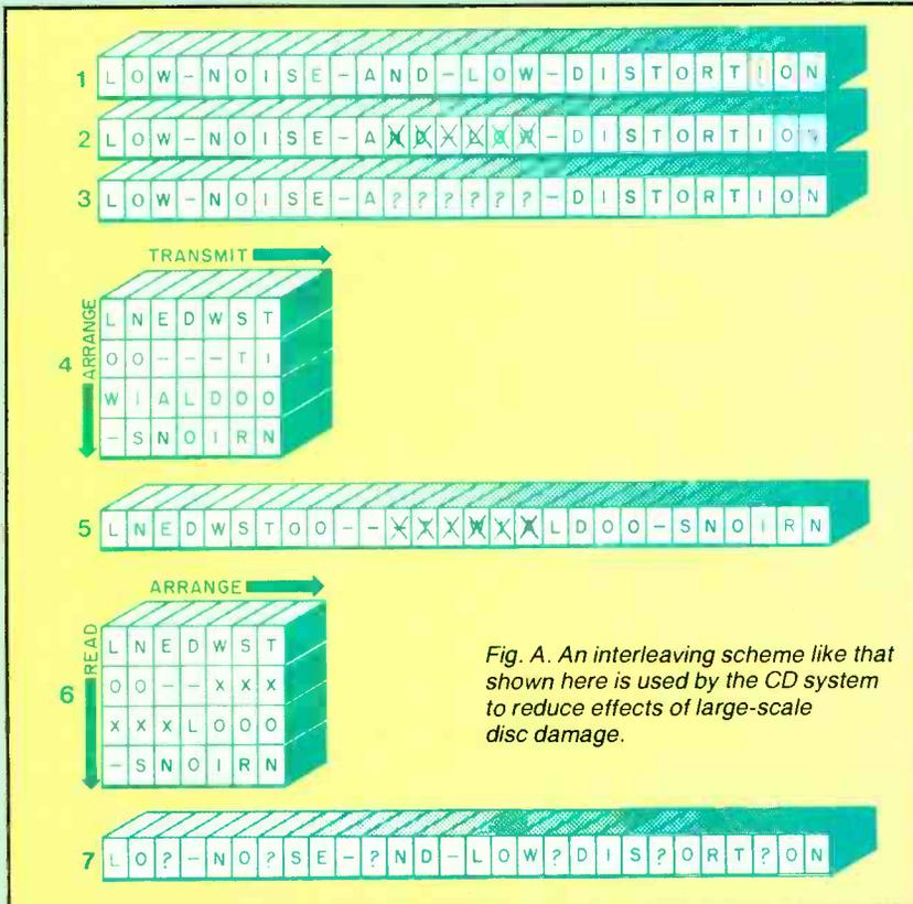
Fig. A. An interleaving scheme like that shown here is used by the CD system to reduce effects of large-scale disc damage.
