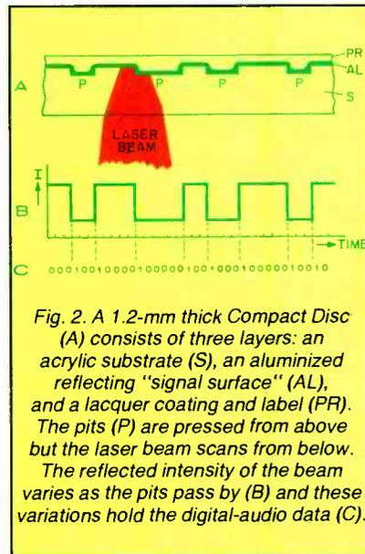
Fig. 2. A 1.2-mm thick Compact Disc (A) consists of three layers: an acrylic substrate (S), an aluminized reflecting "signal surface" (AL), and a lacquer coating and label (PR). The pits (P) are pressed from above but the laser beam scans from below. The reflected intensity of the beam varies as the pits pass by (B) and these variations hold the digital-audio data (C).
