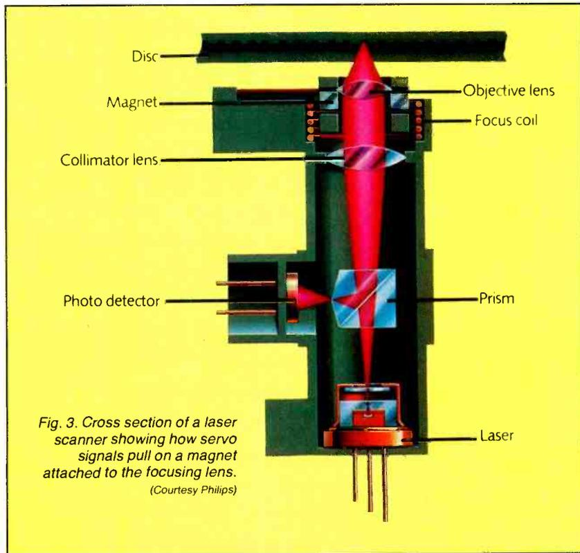
Fig. 3. Cross section of a laser scanner showing how servo signals pull on a magnet attached to the focusing lens. (Courtesy Philips)
