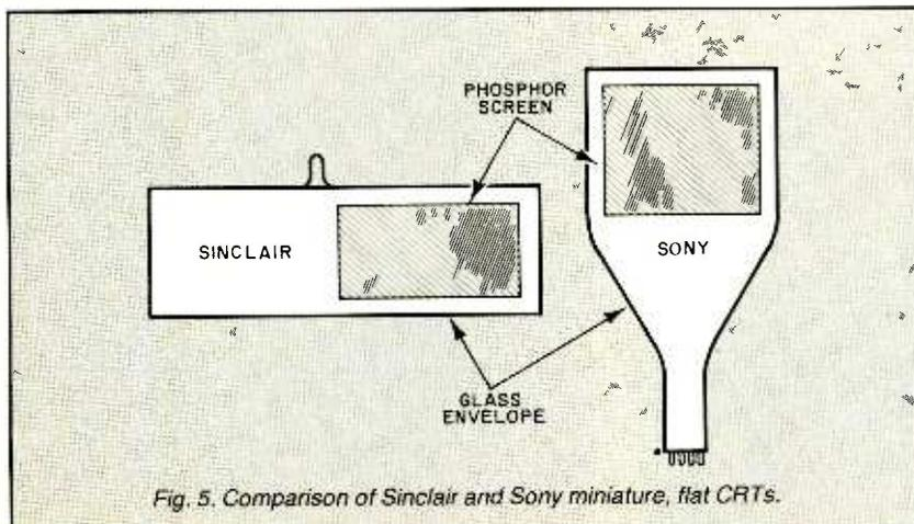
Fig. 5. Comparison of Sinclair and Sony miniature, flat CRTs.
