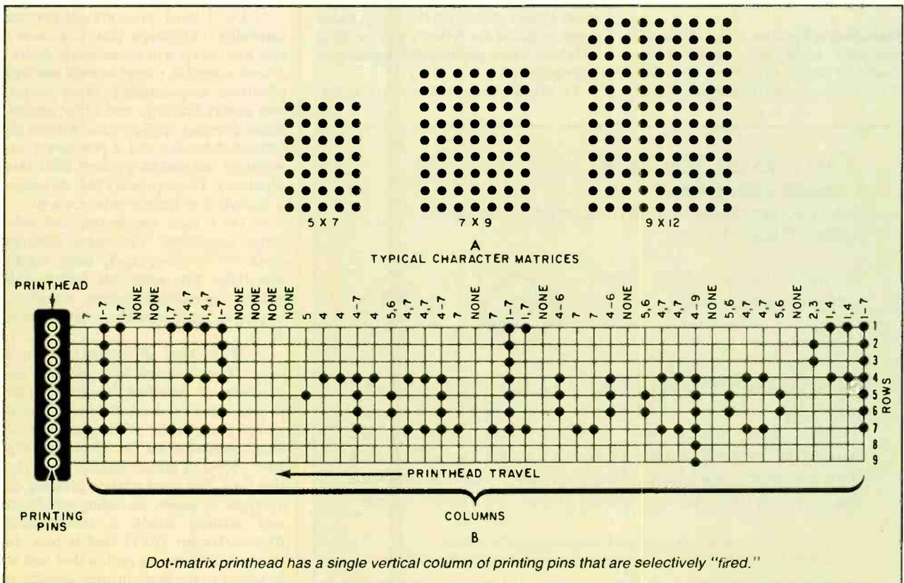
Most dot-matrix printers operated in the graphics mode are slower than in the text mode because printing is in only one direction. There are a few exceptions to this, of course. For example, Centronics recently introduced a line of dot-matrix printers capable of printing graphics bidirectionally.)
