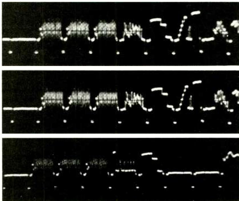
*Top and center are Teletext signals on NBC and CBS respectively. At bottom are closed-captioning signals on PBS.*
