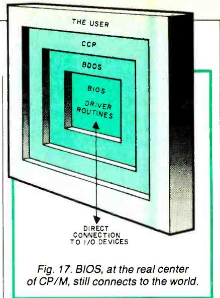
Fig. 17. BIOS, at the real center of CP/M, still connects to the world.
