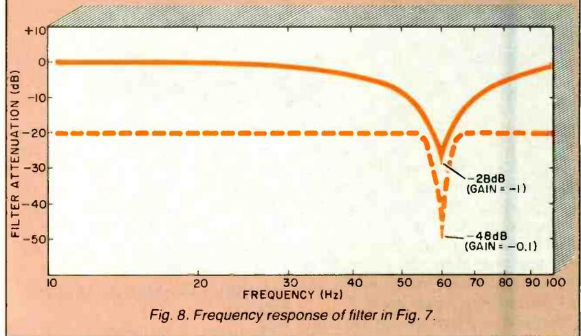
Fig. 8. Frequency response of filter in Fig. 7.
