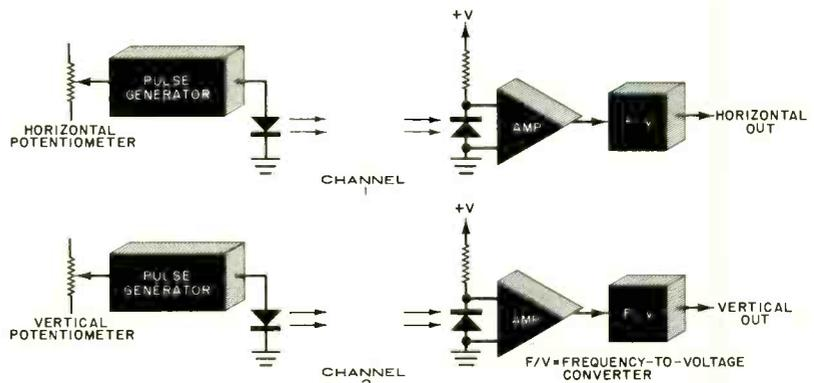
Fig. 4. Block diagram of infrared computer-joystick interface.
