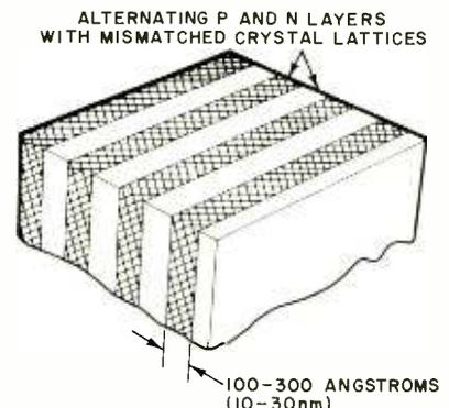
Fig. 8. Formation of a simple strained-layer superlattice device.
