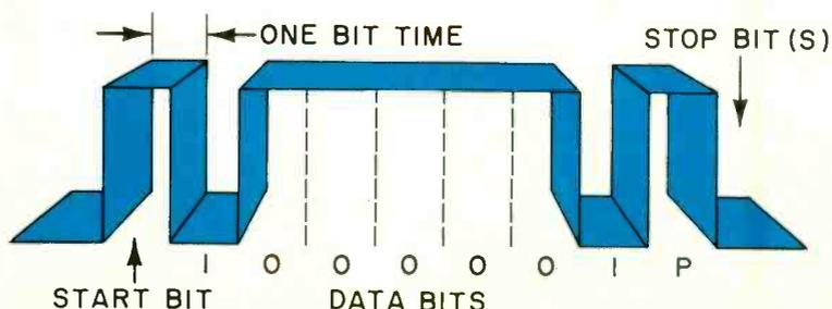
Fig. 3. Diagram of a typical serial data transmission.
