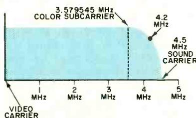
Fig. 2. Envelope bandwidth of an ideal television signal.
