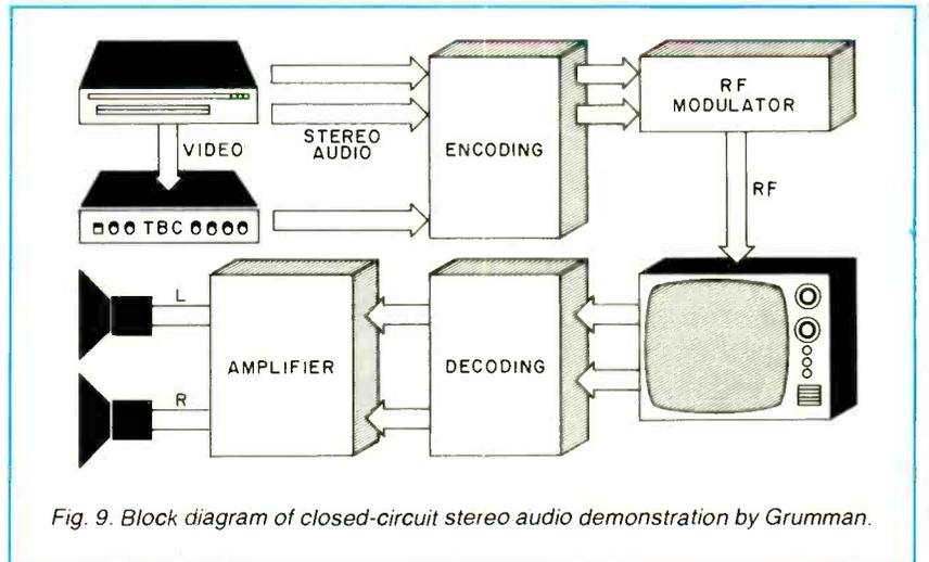
Fig. 9. Block diagram of closed-circuit stereo audio demonstration by Grumman.
