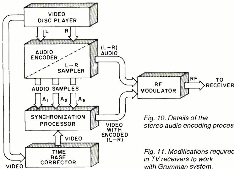
Fig. 10. Details of the stereo audio encoding process.
