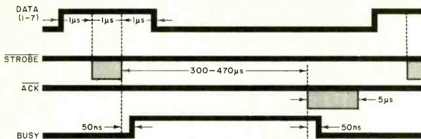
Fig. 2. Timing chart for a Centronics parallel interface.
