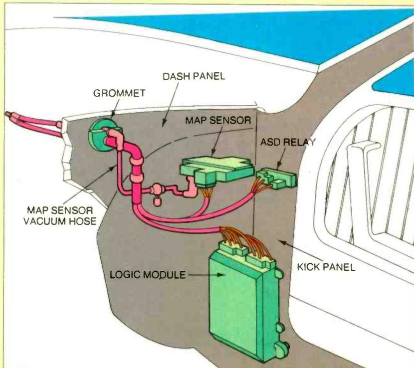
**Logic module is located behind kick panel on passenger side of automobile for easy servicing.**
