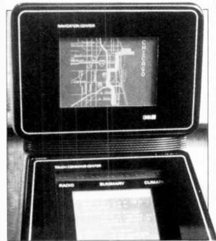
**Touch screen controls radio, interior climate, navigation and compass. Digital map is on cassette.**
