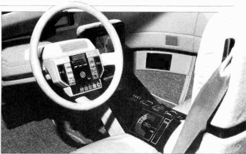
**Vehicle controls mounted on steering column of concept car: road-surface traction monitor, voice-activated telephone and laser ignition "key."**
