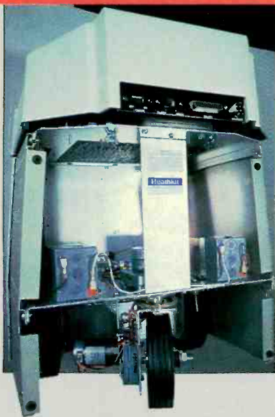
HERO JR's driving wheel can swivel a full 360 degrees.
