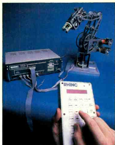
The Rhino robot can be controlled by keypad or personal computer.
