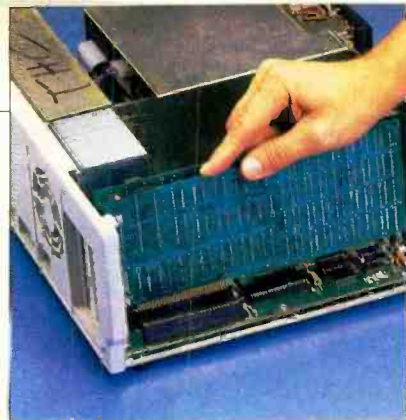
The 1000 can accommodate three IBM-compatible expansion boards.
