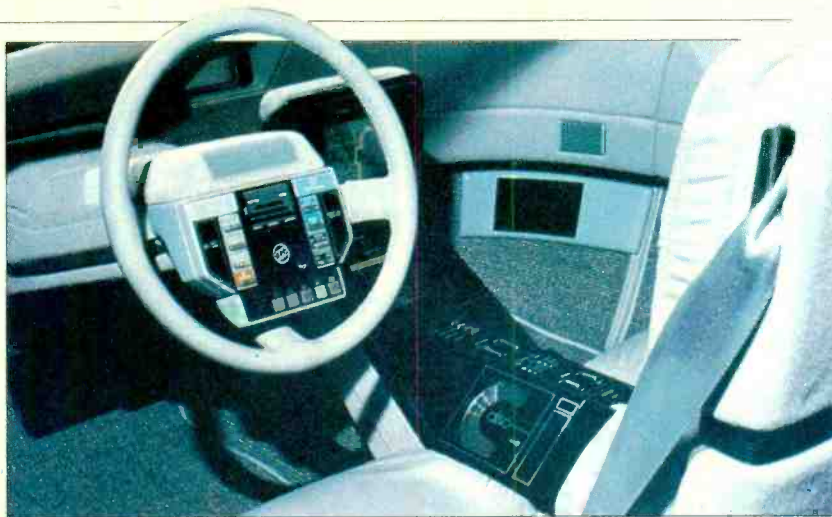
Vehicle controls mounted on steering column of concept car: road-surface traction monitor, voice-activated telephone and laser ignition "key."
