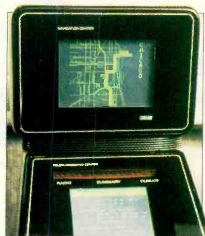
Touch screen controls radio, interior climate, navigation and compass. Digital map is on cassette.
