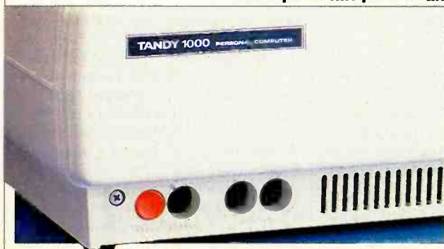
Front panel has reset button and keyboard and joystick connections. Back panel has parallel and video ports and audio output.
