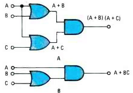
Fig. 7. A product-of-sums (A) can be simplified into a sum-of-products (B). You can see that the sum of products version (B) is much simpler.
