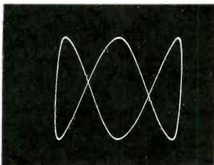
When two waves control the beam position, a Lissajous pattern is formed from them.
