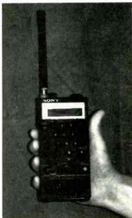
*The Sony Air-8—which is primarily designed for private pilots—features search/scan, selectable channel delays, lockouts, a 10-channel memory for each band, a backlit LCD display, keyboard locks, priority channel, and (to top it off) is keyboard programmable.*
