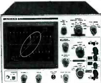
Stereo oscilloscopes (cousins of the dual-trace models) like this Leader model, allow viewing of two waveforms side-by-side simultaneously.
