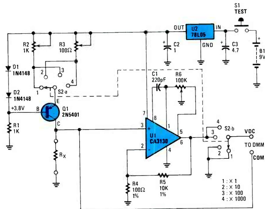
Fig. 1. The circuit consists of a 5-volt DC regulator (U2), a constant-current source (D1, D2, and Q1), and an op-amp voltage-gain stage (U1).
