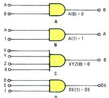
Fig. 1. Here we demonstrate the laws of intersection. In A, one input of the AND gate is 0, making the output 0. In B, a binary 1 is applied to an input, making the output simply A. Figures C and D demonstrate the same principle for multiple inputs.
