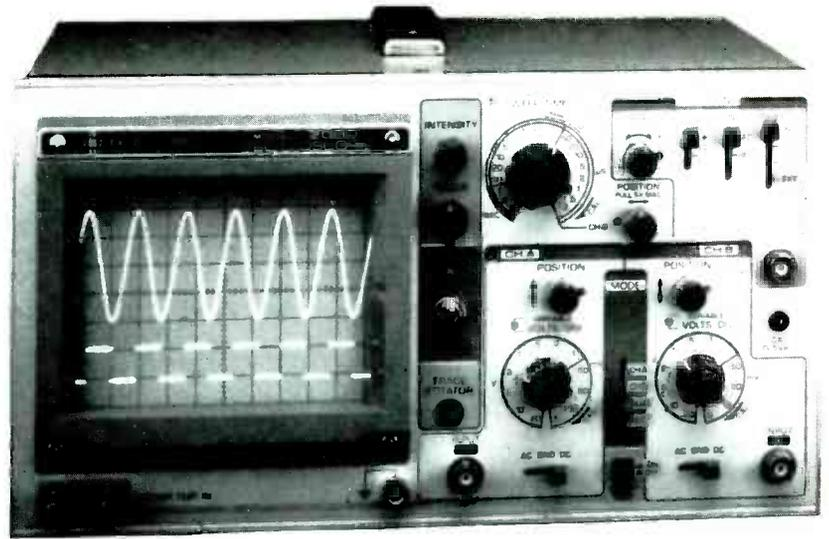
An interesting feature in this oscilloscope from JDR is Z-axis intensity modulation, which gives complex graphs a 3D feeling by altering the beam intensity.
