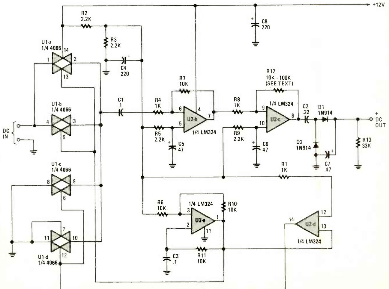
Fig. 1. The Dual Chopper Amplifier circuit is built around a 4066 quad bilateral switch and a quad op-amp.
