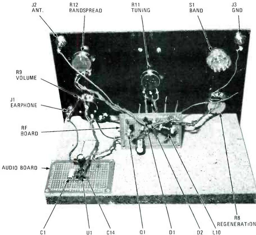
All audio components are mounted on the audio perfboard except the controls and earphone jack. Connections between the boards and outside components are made after they are mounted on the wood chassis.
