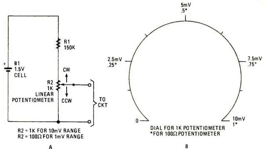
Fig. 2. This simple circuit can be used to calibrate the dual Chopper Amplifier.
