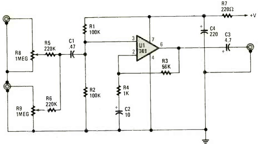
Fig. 7. The Rock Mixer allows one mike to cut while boosting another.
