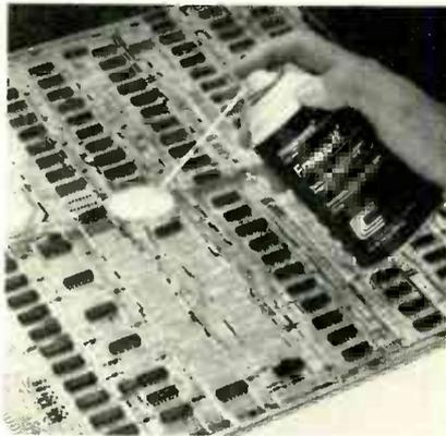
nents and systems with instant freezing of small areas to as low as  $-96^{\circ}\text{F}$  ( $-71^{\circ}\text{C}$ ). It is also useful for heat-sink protection of components during soldering and testing, and freezing of adhesives to facilitate removal.
