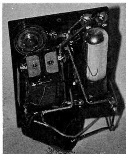
Although large by today's standards, the Cummings Solodyne was very compact for 1928. All components are mounted to the front panel by either the pin jacks or the screws holding the variable capacitor,
