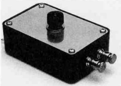
Under the knob on top of the unit is an old plastic single-pole, single-throw rotary switch. A small SPST toggle switch will work just as well.
