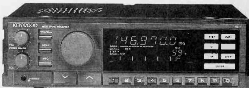
*Kenwood's RZ-1 packs a lot of features into one unit. With a range from 500 kHz to 905 MHz, you get AM/FM, SW, TV, and all the UHF/VHF bands. It stores 100 channels in memory, features band scan and memory-channel scan, and offers manual and automatic tuning.*
