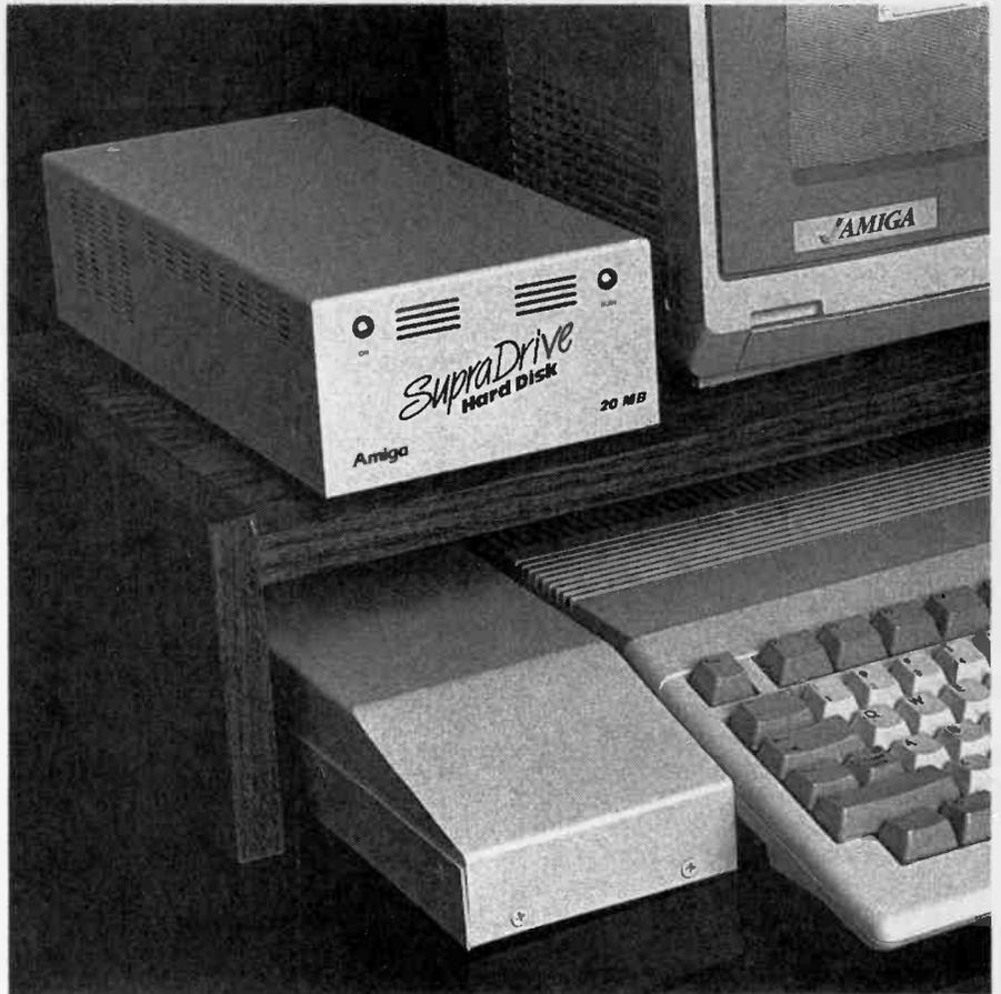
*SupraDrive hard-disk system is for the A500 and includes the hard-disk drive, SCSI expansion port, and an easy way to expand the Amiga's memory using a plug-in RAM module. The high-speed drive is available in capacities ranging from 20 to 250MB. (Photo courtesy Supra Corporation.)*
