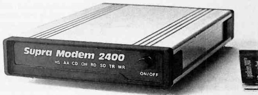
The SupraModem 2400 is an inexpensive 2400-baud modem that supports most computers with an RS-232C interface, including all Amiga models. (Photo courtesy Supra Corporation.)
