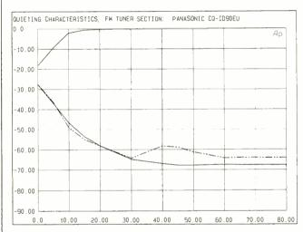
Fig. 2. In mono (lower solid trace), the best S/N was 68 dB, which is adequate for a car FM tuner. In the stereo mode (upper solid trace), the S/N was almost as good, measuring 65 dB for strong signals.
