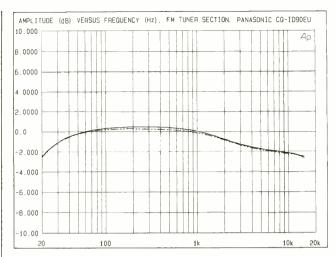
Fig. 1. At 15 kHz, the frequency response of the FM-tuner section was off by only 2.5 dB.
