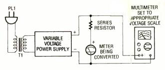
*Oops' The multimeter was shown connected incorrectly in Fig.* 2A of last month's column. Here's the proper method.
