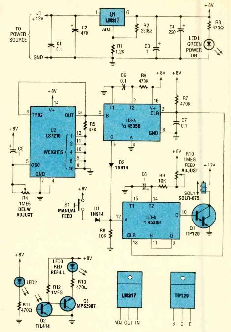
Fig. 1. The heart of the Auto-Feeder is U2, an LS7210 programmable delay timer, which institutes a 12-hour delay, between feedings. At the end of the delay, U2 triggers a dual monostable (U3), that activates a solenoid (SOL1), which a moves a flipper, allowing fish food to fall into the tank.
