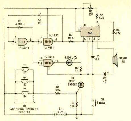
Fig. 1. The  $3 \times 3$  Alarm consists of two IC's (U1 and U2), a silicon-controlled rectifier (SCR1), a speaker (SPKR1), and a few support components.
