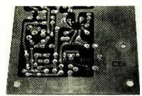
A missing land on this board has been replaced by a small wire as shown. That technique can save many a board along the way.
