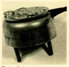
The Auto Feeder uses a rotary type solenoid (SOLI), which draws about 400 milliamperes when energized and is operated from the unregulated 12-volt supply, to eliminate any effects its current drain might have on the regulated 8-volt power supply. When this rotary solenoid is energized, the circular plate on top rotates about 20 degrees. On deenergizing, the circular plate returns to its original position.
