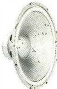
Dual voice coil. 40 oz. magnet. 6 ohm imp. 100W RMS, 140W max. Response 20-20KHz. Resonant frequency: 21Hz. SPL=93 dB 1W/1M.
