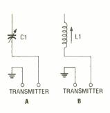
Fig. 2. A capacitor (A) can be connected in series with the antenna to electrically shorten it; placing an inductor (B) in series with the antenna electrically lengthens it.
