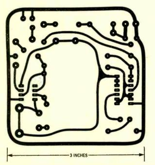
Fig. 2. While there is nothing critical about the construction of the  $3 \times 3$  Alarm to preclude its being built on perfboard, printed-circuit construction is recommended for ease of assembly. Here's the author's printed-circuit board foil pattern.
