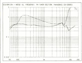
Fig. 3. At mid-frequencies, mono distortion plus noise (solid trace) measured 0.33%, while in stereo (dashed line), the distortion increased to 0.6% at that same test frequency.
