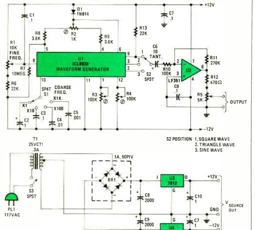
Fig. 1. The Function Generator is built around Intersil's ICL8038 waveform generator. With the addition of a few support components, the circuit was given the ability to switch through several coarse frequencies in decade steps.
