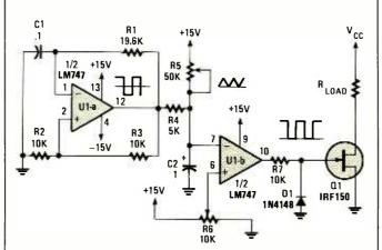
Fig. 6. This Pulse Width Modulation Circuit uses an op-amp to lessen the amount of power dissipated by the FET transistor.
