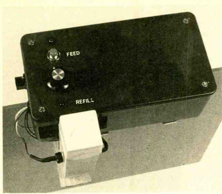
Four holes were drilled in the lid of the enclosure to accommodate SI (MANUAL FEED), LEDI (POWER ON), LED3 (REFILL), and R10 (FEED ADJUST).
