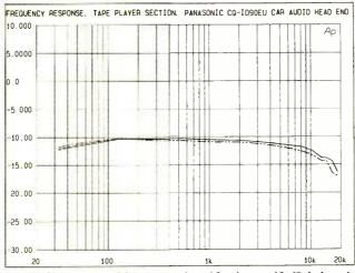
Fig. 7. Using normal-bias tape played back at -10 dB below the reference level, frequency response was down by approximately 7 dB at 18.5 kHz, the highest frequency available on the test tape.
