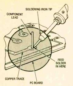
Fig. 1. If you hold the iron as shown, both surfaces will get hot, and the solder will flow properly.
