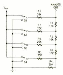
Fig. 3. Here we have the resistor ladder from Fig. 2 connected to a switching network. It contains four single-pole, double-throw switches. Note that we're using 5 volts as the reference voltage.
