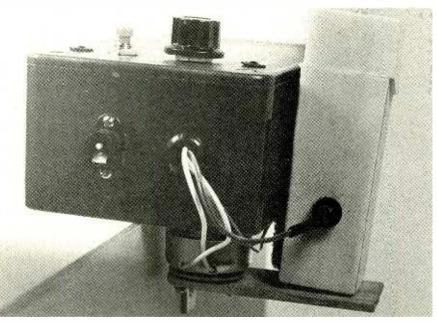
The solenoid mounts underneath the project enclosure. One end of a wooden flipper mounts on the solenoid's rotating circular plate, the other end rests under a fish-food bin, which has a hole in its bottom. When the solenoid is energized, the flipper moves away from the hole, and fish food falls through the hole into the fish tank. In addition to automatic feeding, you can manually feed your fish by pressing SI (FEED).
