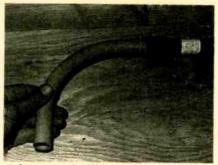
A factory-made 90° bend eliminates the need for a conduit bender. Just cut the conduit to length and glue the parts together.
