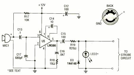
Fig. 5. This simple circuit allows the strobe circuit to be used as a sound detector: such a circuit might be used to detect sounds within a covered area, indicating that the perimeter has be breached.
