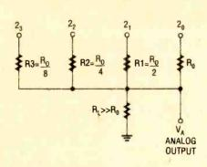
Fig. 1. The analog output voltage  $(V_A)$  of our resistor divider can be most easily found through Millman's theorem, which states that the voltage appearing at any node in a resistive network is equal to the sum of the currents entering the node divided by the sum of the conductances connected to the node.
