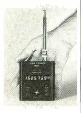
overlapping ranges-1-500 MHz and 200-1500 MHz-and two switch-selectable gate times. The fast gate time of 0.25 seconds yields a 1-kHz resolution; the slow gate time of 2.5 seconds yields a 100-Hz resolution.
