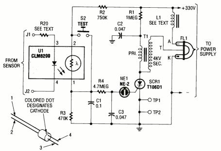
Fig. 1. The SentryStrobe is built around a trigger transformer, a Xenon flash lamp, an SCR, and a neon lamp (which is used to trigger the SCR). A CLM6200 optoisolator/ coupler accepts trigger inputs from an external signal source to fire the strobe circuit.
