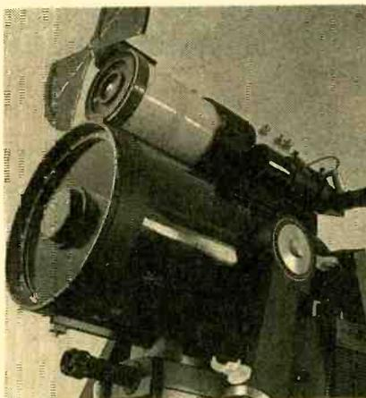
This is an electronically controlled search telescope with top-mounted biosensor assembly. The Faraday tube is shuttered to prevent electromagnetic interference.
