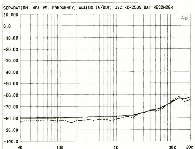
Fig. 5. Stereo separation at 1 kHz measured around 80 dB, but decreased to between 62 and 65 dB at 20 kHz. While we have measured higher, these separation figures are certainly more than adequate for good stereo reproduction.
