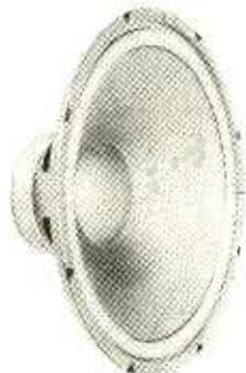
Dual voice coil. 40 oz. magnet. 6 ohm imp. 100W RMS, 140W max. Response 20-1.2KHz. Resonant frequency: 21Hz. SPL=93 dB 1W/1M
