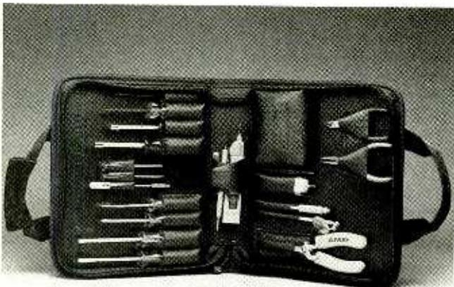
wire crimper/stripper; a four-inch compudriver; an RS-232 insertion extraction tool; a DIP inserter and a DIP extractor; an inspection mirror; and an adjustable 4-inch wrench. The tools are held securely in place in a compact (11½ × 10 × 2½-inch) case that features two roomy outside pockets.
