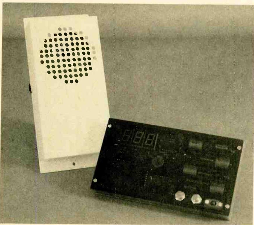
Here are two custom fitted project enclosures. The one to the left has a perforated speaker area near the top; the other has its front panel made of tinted translucent acrylic eliminating the need of a cutout area for the display.
