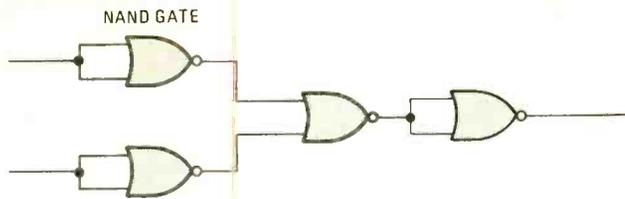
Fig. 3. By adding one more inverter, we can take our equivalent AND gate a step farther to turn it into an NAND gate.
