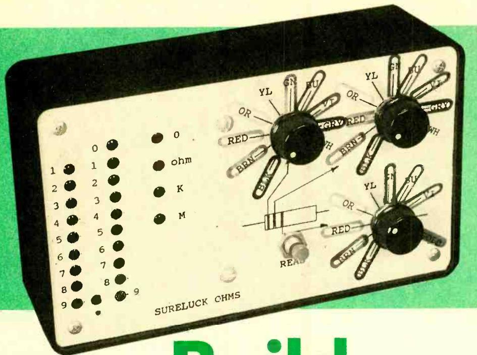
*If selecting a required resistor solely by color code is giving you headaches, or if you simply don't know the code well enough to use it accurately, check out Sure-luck Ohms—the easy-to-build color-code sleuth!*
