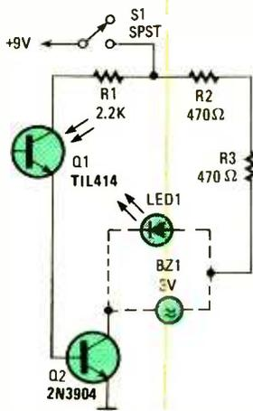
Fig. 12. This detector circuit provides audible as well as visual indications.
