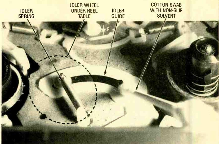
*Fig. 1. A lot of problems can be traced to slipping idler wheels. If your VCR has a guide like the one shown here between the reel hubs, it uses an idler wheel. The idler wheel (indicated by the dashed outline) is below the reel table. To avoid a lot of disassembly, apply non-slip solvent to the rubber part of the idler by inserting a cotton swab through the hole in the guide.*
