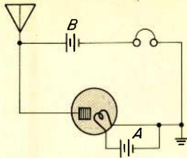
Fig. 3. Lee de Forest's diode audion detector allowed him to eliminate the flame by using a low-vacuum glass tube.
