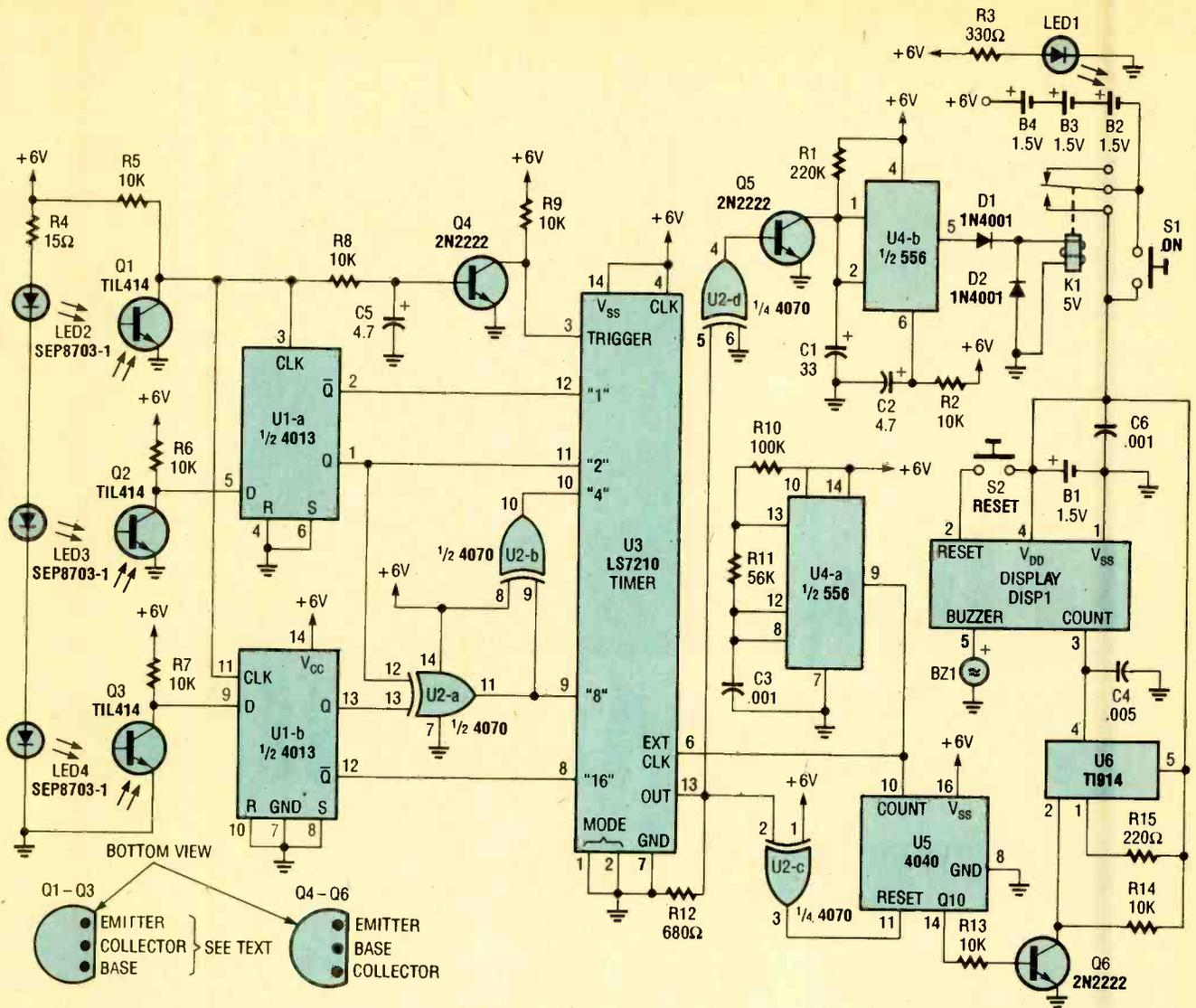
Fig. 1. This is the circuit for the "Slot-Machine" Bank. The phototransistors on the left determine what coin has been put in the slot and that is converted into pulses for the counter.
