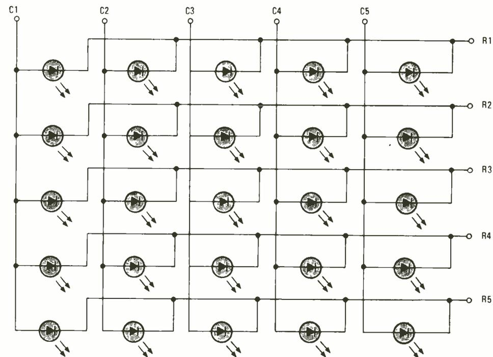
Fig. 4. This is a multiplexed display of LED's. A particular LED can be lit by connecting its row and column terminals to a power supply.
