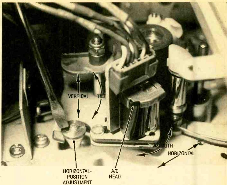
*Fig. 3. This is the A/C (audio/control) head. There are four adjustments: horizontal position, vertical position, tilt, and azimuth. The adjustments affect sound quality and sync. They also have an effect on picture tracking.*
