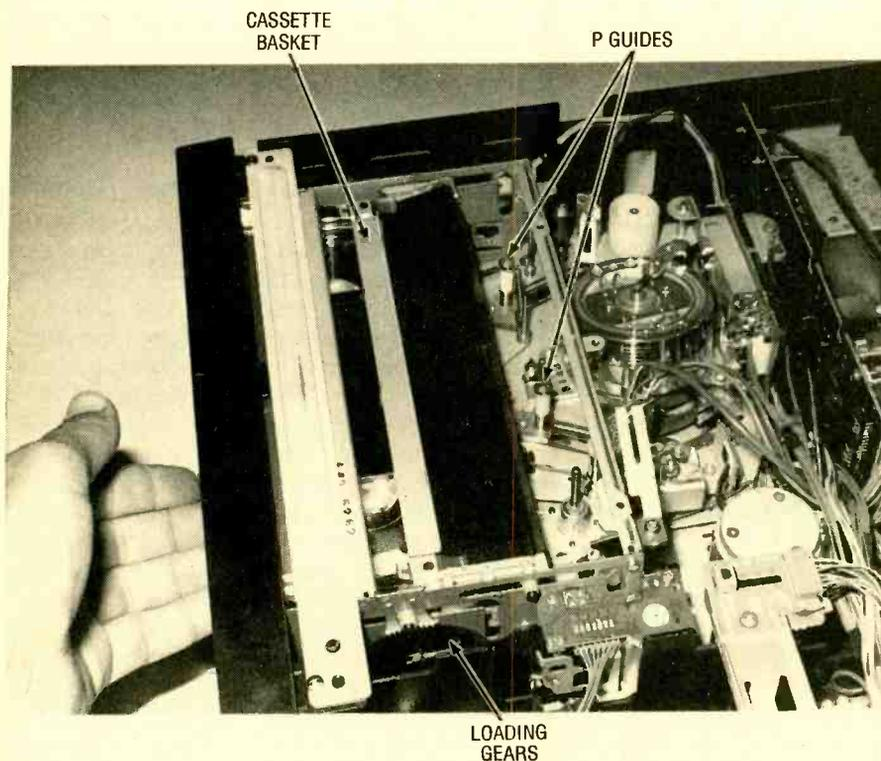
*Fig. 2. When you insert a cassette, a switch activates a motor that drives the cassette basket. The basket pulls the cassette in and then lowers it onto the reel table. If the loading gears become out of time (slip a tooth), then the mechanism will jam as it lowers the basket.*
