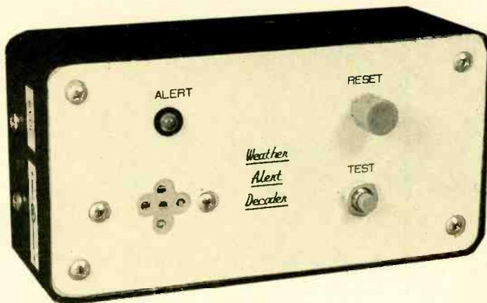
*Catch all the latest weather bulletins transmitted by the NOAA with this easy-to-build circuit that alerts you to impending NOAA broadcasts.*
