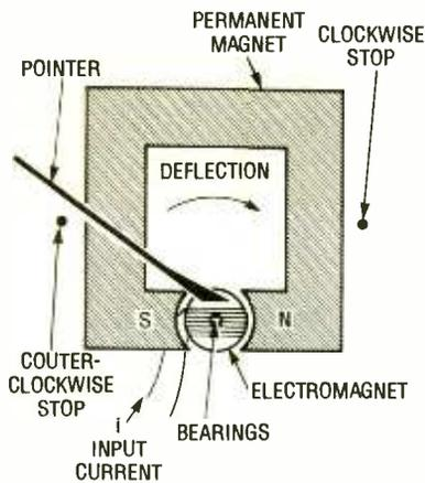
Fig. 1. This is a simple d'Arsonval movement. The deflection of the needle is proportional to the input current ( $i$ ).
