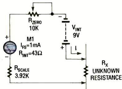
Fig. 4. A meter's internal voltage source is used to drive an ohmmeter circuit.
