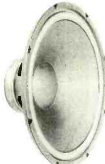
Dual voice coil. 40 oz. magnet. 6 ohm imp. 100W RMS, 140W max. Response: 20-1.2KHz. Resonant frequency: 21Hz. SPL=93 dB 1W/1M.
