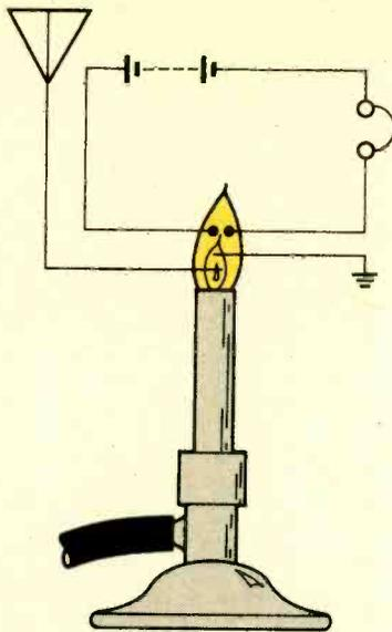
*Fig. 2. The second style of flame detector had a local battery circuit which allowed it to operate better.*
