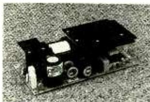
*FLU4-100 Series* is a family of highly reliable quad-output, 100-watt switching power supplies. Five models provide outputs of +5 VDC and combinations of -5, +/-12, +/-15, and +24 VDC. Three models include a fully isolated auxiliary output. The FLU4-100 units are each fabricated on a single 4 x 8-inch printed-circuit board.
