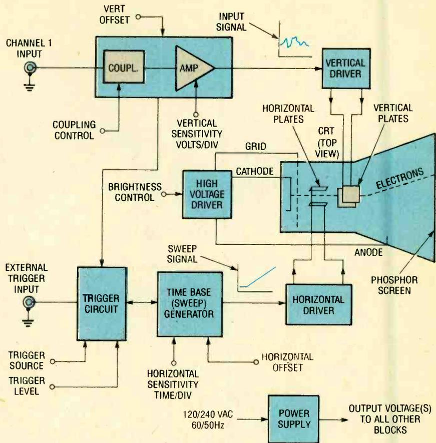
Fig. 1. Block diagram of a simple oscilloscope.
