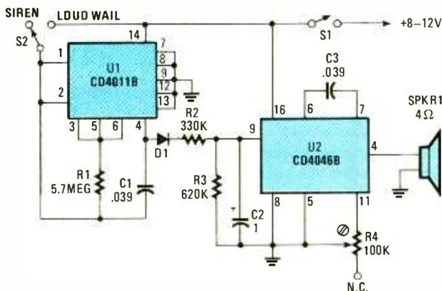
Fig. 6. This siren has very low power consumption. It could sound-off for a long time before draining its battery power supply.
