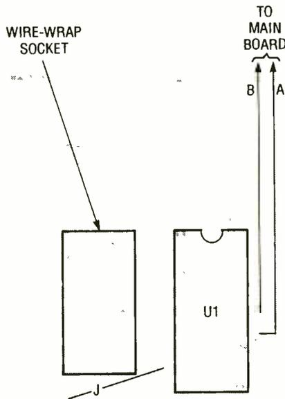
Fig. 7. The adapter board contains only two parts: an IC socket and a 6-bit ADC. Don't forget to add the jumper wire though.
