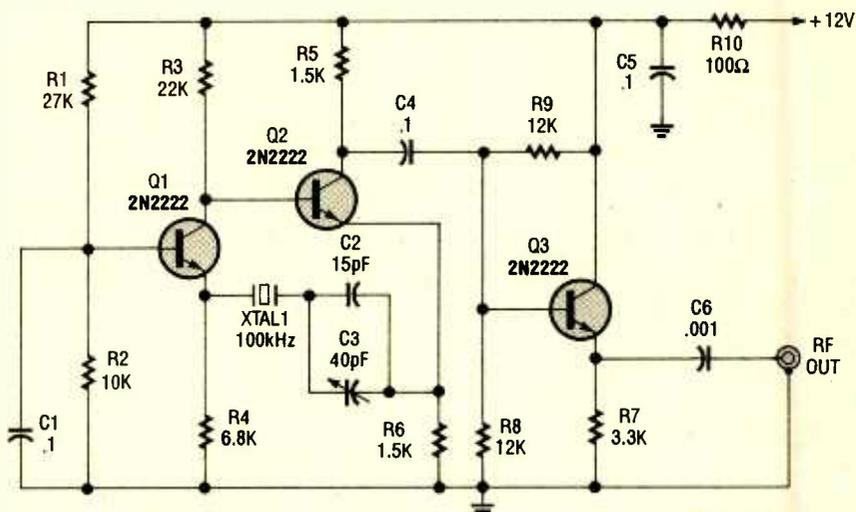
Fig. 7. This 100-kHz crystal-based calibrator can be built from readily available parts. It can be calibrated using the either the WWV or WWVH radio signals.
