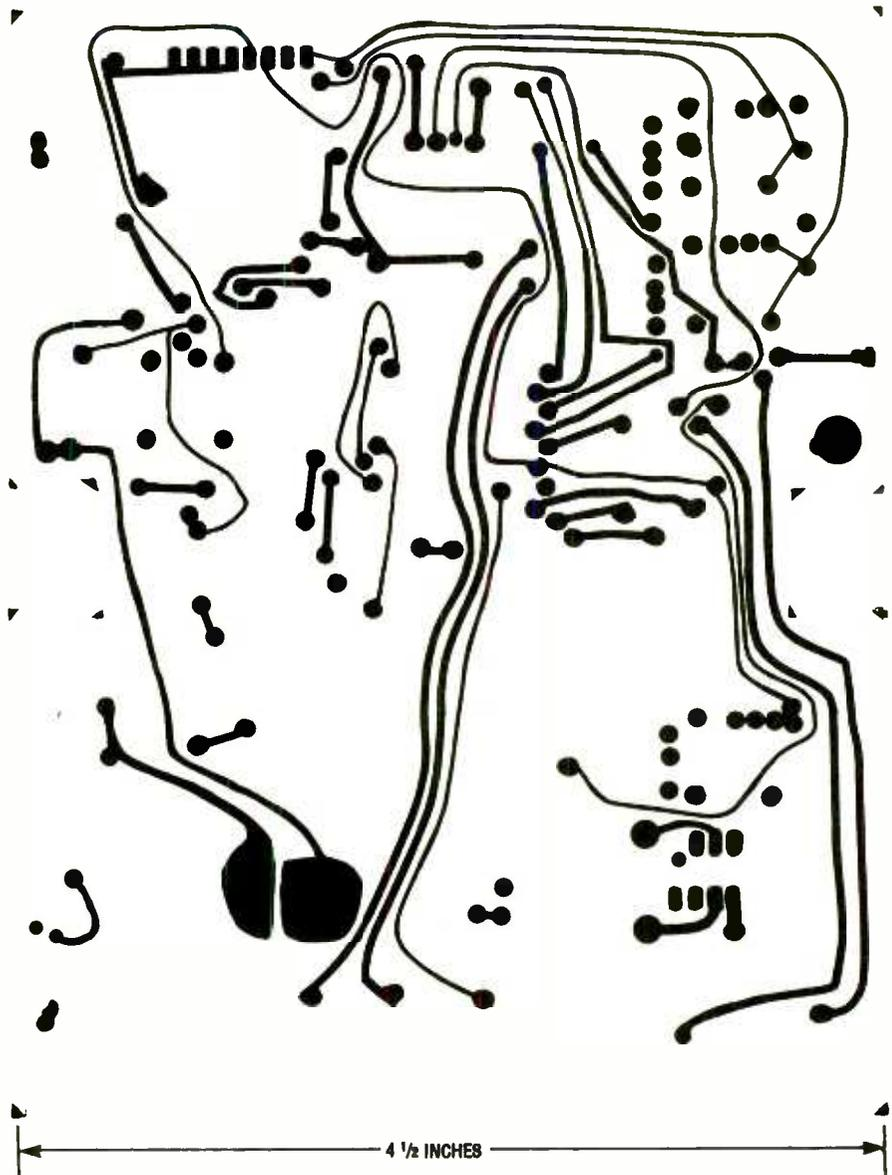
Fig. 3. This is one foil pattern for the main circuit board. Most of the components will be mounted on this side.
