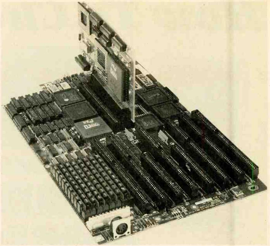
*This is the motherboard of a 386 computer. If in the future you find that you'll need the power of a 486-based machine, you could always upgrade it with an expansion board (also shown here). The point is don't go for overkill; you can always upgrade later.*
