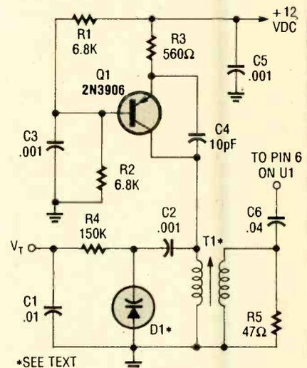
Fig. 6. You can make the circuit of Fig. 5 tunable by replacing its crystal-based local oscillator with this voltage-controlled oscillator. The operating frequency is determined by the voltage at  $V_T$ .
