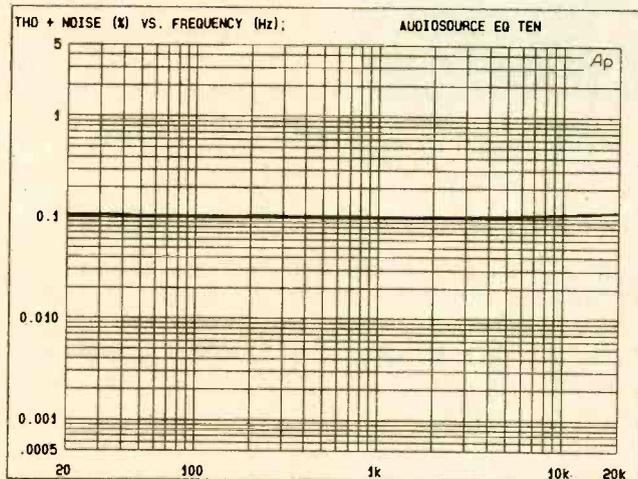
*This plot of harmonic distortion plus noise versus frequency showed that the THD plus noise remained virtually constant throughout the test-frequency range. At 0.1% it was certainly acceptable, although considerably higher than the .008% claimed by the manufacturer.*
