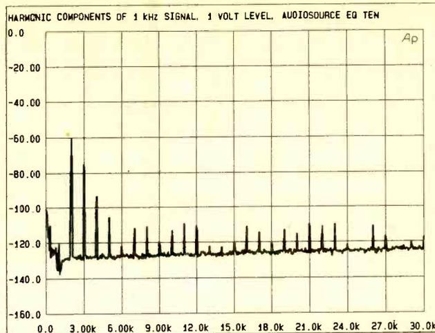
*This spectrum analysis of the harmonics of the 1-kHz, 1-volt test signal showed that the most prominent harmonic, at 2 kHz, is at  $-60$  dB relative to the fundamental 0-dB reference level, corresponding to a distortion level of 0.1%. Note that the 1-kHz fundamental was notched out for this test.*
