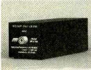
proven nine-pole Chebyshev low-pass filter design. The low-pass filter handles a full 1500 watts of power with low SWR, and insertion loss is less than 0.5 dB. The compact unit measures 8¼ inches deep by 2¾ inches wide by 3 inches high.
