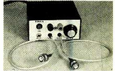
When used with a scope the EZ-Curve Signature Tracer can diagnose the condition of a variety of components.
