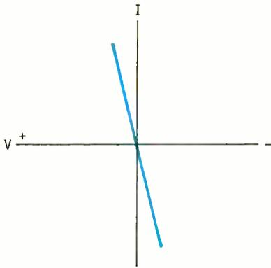
Fig. 3. Resistors produce the most boring characteristic curves. The inverse of the slope is the resistance.
