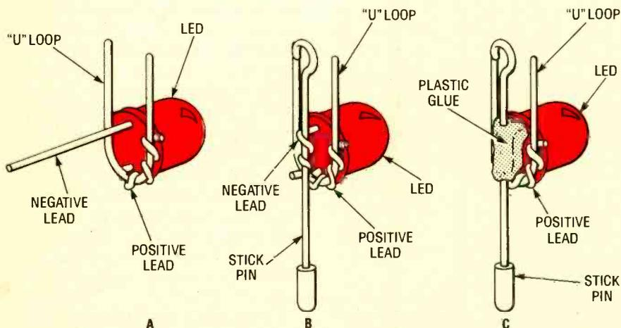
*Fig. 1. Wrap a turn or two of the LED's positive lead around the U-loop (A), with the negative loop extending through the center of the loop. Coil the LED's negative lead around the pin (B), and solder. Then fill the space between the LED's base and the stick pin with glue (C).*
