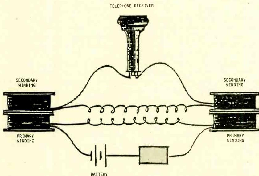
*The rheotome (R) used in Hughes' induction balance to produce current pulses in the circuit's primary windings initially consisted of a mechanical interrupter, but later was changed to a ticking clock and microphone.*
