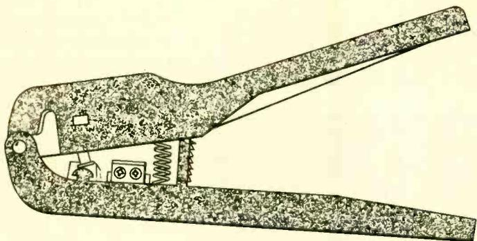
Fig. 7. This is what the crimping tool required to attach a modular plug to quad line cord looks like. To use it, simply load a plug into the tool, insert the line cord into the slot on the plug, and squeeze.
