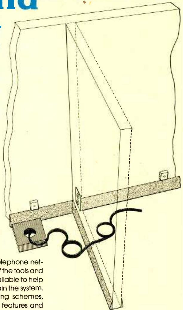
quad-terminal connection block (see Fig. 1). The terminal block has four color-coded screw terminals, labeled R for red, G for green, Y for yellow, and B for black. The R and G (in telephone parlance, ring and tip, respectively) terminals are the main connection points for any telephone installation; they carry both the ring signal and verbal communications.
