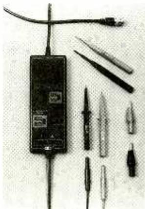
rate measurements of small signal differences even in the presence of very high common-mode voltages. It has a bandwidth of DC-15 MHz and a switchable  $\times 20$ - $\times 200$  attenuation ratio. It comes with standard probes, alligator clips, and spring-tip probes with banana plug leads.
