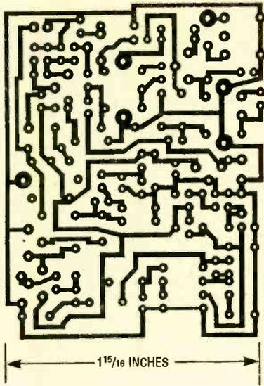
Fig. 4. The author's prototype was assembled on a printed-circuit board that measures about 1<sup>15</sup>/<sub>16</sub> by 2 inches. This full-size template of the printed-circuit artwork is provided so that you can etch your own printed-circuit board.
