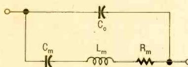
Fig. 3. The operation of a quartz crystal is best explained through this simplified equivalent circuit, consisting of a series-resonator network made up of  $C_m$ ,  $L_m$ , and  $R_m$ , with a parallel capacitor,  $C_o$ , shunting the crystal's terminals.
