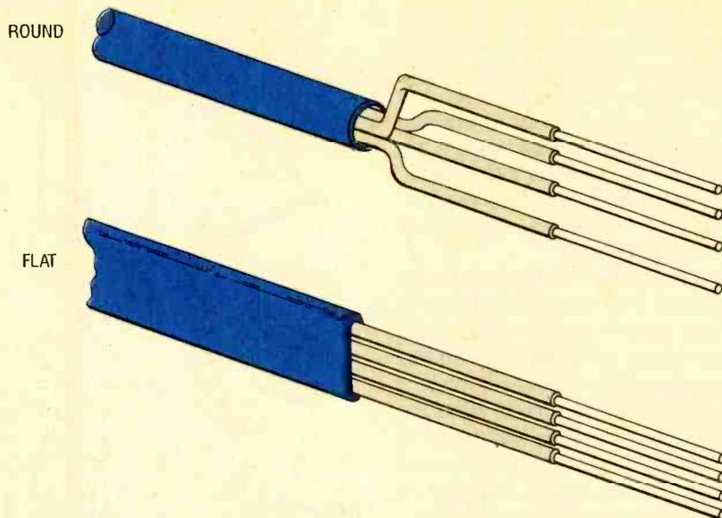
*Fig. 4. Station wire—which is designed for both inside and outside use—differs from line cord in that its conductors are solid, as opposed to the stranded stuff used for line cord, and it is round rather than flat. The insulation of the station wire is also thicker than that of the line cord.*
