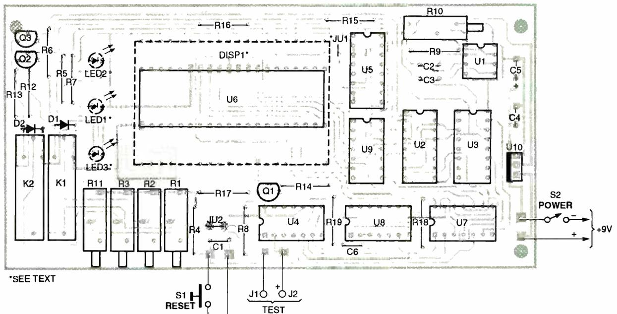
Fig. 4. All components, except the LCD readout and LED's, mount on the component side of the board.
