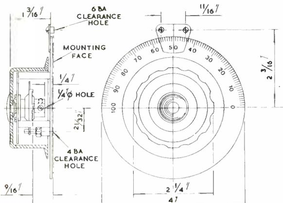
Here's a detailed sketch of the Jackson Brothers 4489/C dial drive. The mechanism offers a 6:1 turns ratio.
