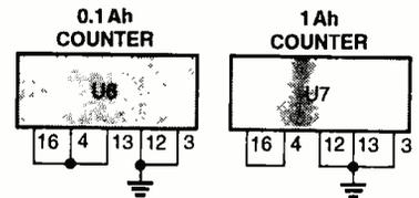
Fig. 6. For options 2 and 3, U6 and U7 must be pre-programmed as described in text. This example shows how to pre-program the chips for a starting value of 1.5 Ah.
