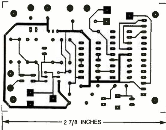
Fig. 3. The author's prototype was assembled on a double-sided printed circuit board, measuring about 2<sup>7</sup>/<sub>8</sub> by 1<sup>15</sup>/<sub>16</sub> inches. Shown here is a full-size template of the foil side of the board.
