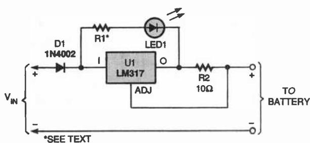
Fig. 5. This current-limiting circuit is great for keeping lead-acid batteries on their toes. All it needs is an appropriate transformer to make it complete.
