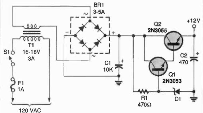
Fig. 7. Here's a 12-volt power supply that is easy-to-build while producing a smooth output.
