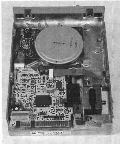
*A 5 1/4-inch drive has a 34-pin card-edge connector on the back end along with one or more power connectors.*
