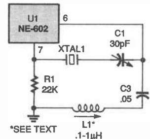
Fig. 3. For higher frequencies, use an overtone crystal oscillator like the one shown here.
