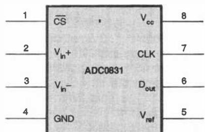
Fig. 1. This is the pinout of the ADC0831, which is the heart of the A/D Converter.
