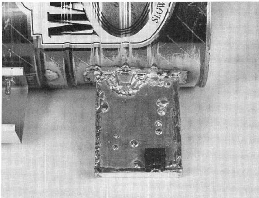
Center the oscillator-board antenna in the 1/4-inch hole, 1 7/8 inches from the closed end of the can, and solder it to the can assembly, completely filling the gap with solder.
