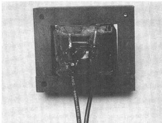
The new choke leads are firmly attached to the coil by a glob of epoxy cement (center) so that the solder joints (at the top of the coil) will not break again.
