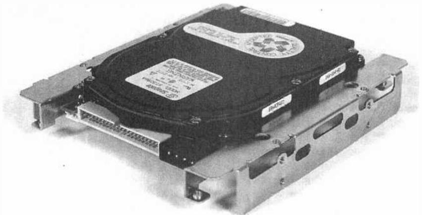
*A mounting kit adapts the hard drive to fit in a 5¼-inch drive bay.*
