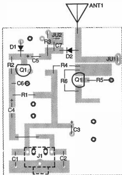
Fig. 6. Careful soldering and the shortest possible lead lengths are important on the microwave-oscillator board. Any lead shown mounted over a circular pad goes through the board and is soldered on both sides, and all other leads are tack soldered on the surface. Note that J1 mounts on the solder side.
