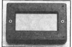
Meter. Features include: 200mV full scale input sensitivity, single 9VDC operation and decimal point selectable. In addition, it has 13mm figure height, automatic polarity indication, guaranteed zero reading for 0 volt input and high input impedance (>100M ohms). Specifications: Max input 199.9mV DC-Max. Display: 1999 counts (3-1/2 digits). Measuring method: Dual slope integration A-D converter system, plus many other features.
